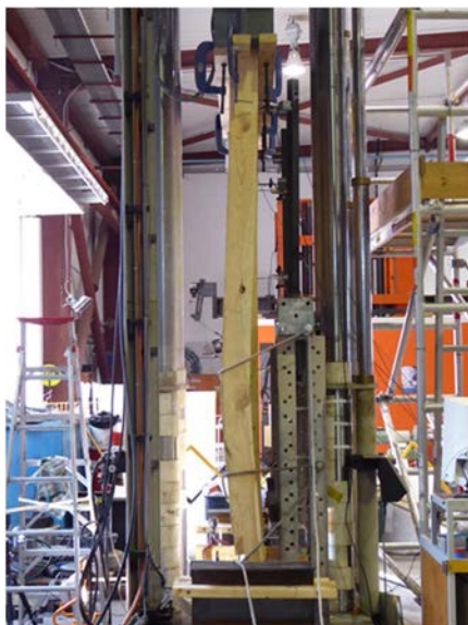
Figure 42a: Buckling initiated by Knot cluster
