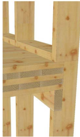
Figure 9: European Notched Stud Direct Bearing Method
