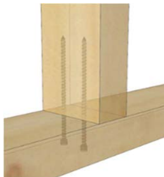
Figure 7: Screw reinforced Wall Plates
