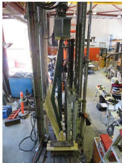
Figure 30: Test 3.1D - Victorian Ash Wall Plate
