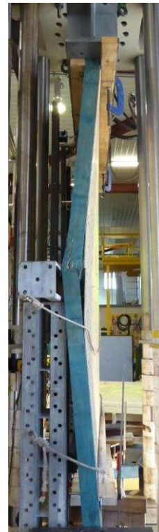
Figure 46: Buckling shape of Configuration 6
