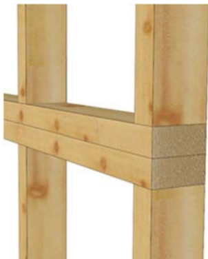
Figure 5: Control Wall Frame - MGP10 plates
