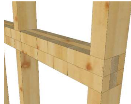
Figure 6: CLT Wall Plates
