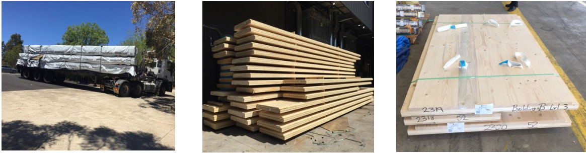
Figure 20: Strongbuild factory's storage yards and tagged panels (Left: raw panel arrival, Middle: Finished panels stack up, Right: Tagged finished panels)
