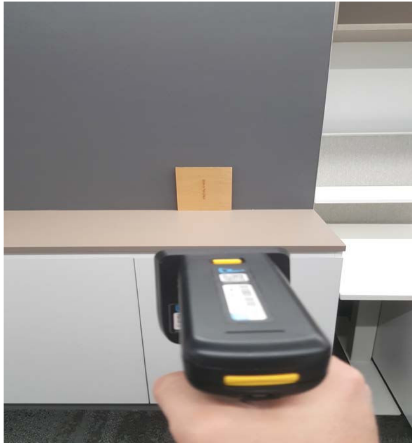
Figure 5: Testing read range through different materials and different thicknesses using UHF reader
