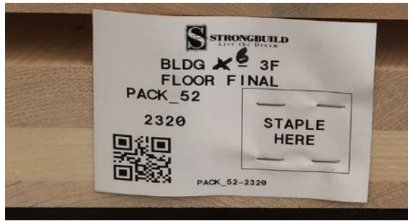
Figure 4: RFID Label stapled to CLT panel (Source: Strongbuild P/L)
