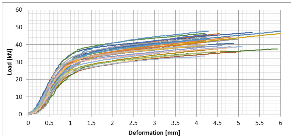
Figure 81: Radiata Pine – End of Plate (S10), All test results – Perpendicular to the grain bearing - Load/Deformation
