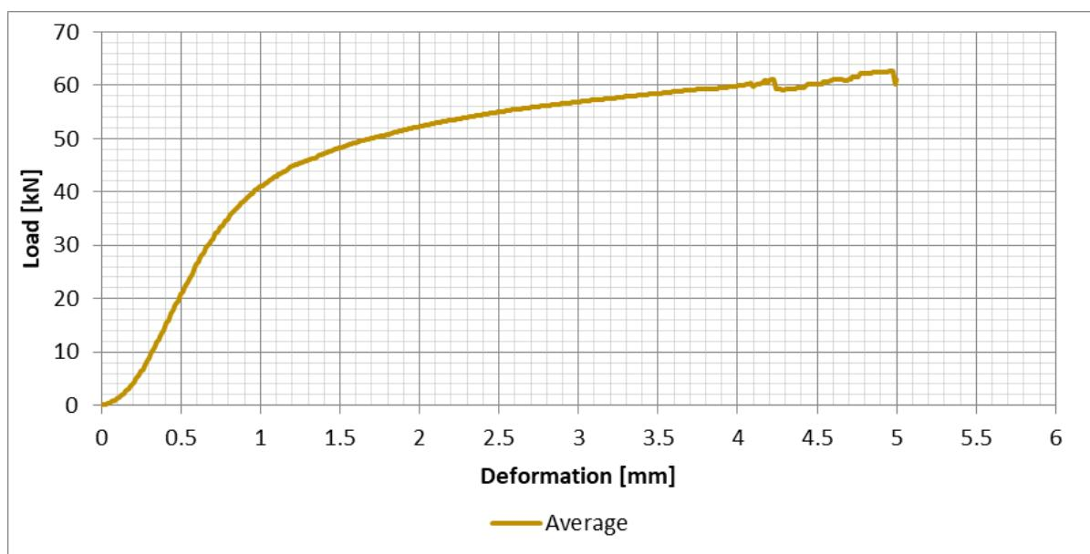
Figure 74: Scot Pine – 150 mm Bearing (Three studs) (I7), Average of all test results – Perpendicular to the grain bearing - Load/Deformation
