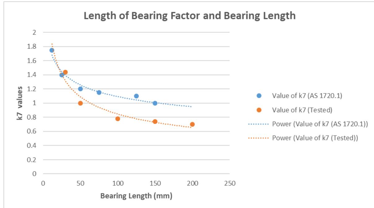
**Figure 87: Comparison of  $K_7$  factor: AS 1720.1 and test results**
