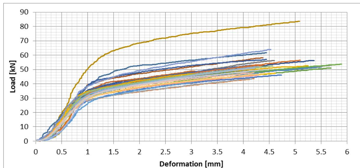
Figure 79: Radiata Pine – Middle of Plate (S10), All test results – Perpendicular to the grain bearing - Load/Deformation
