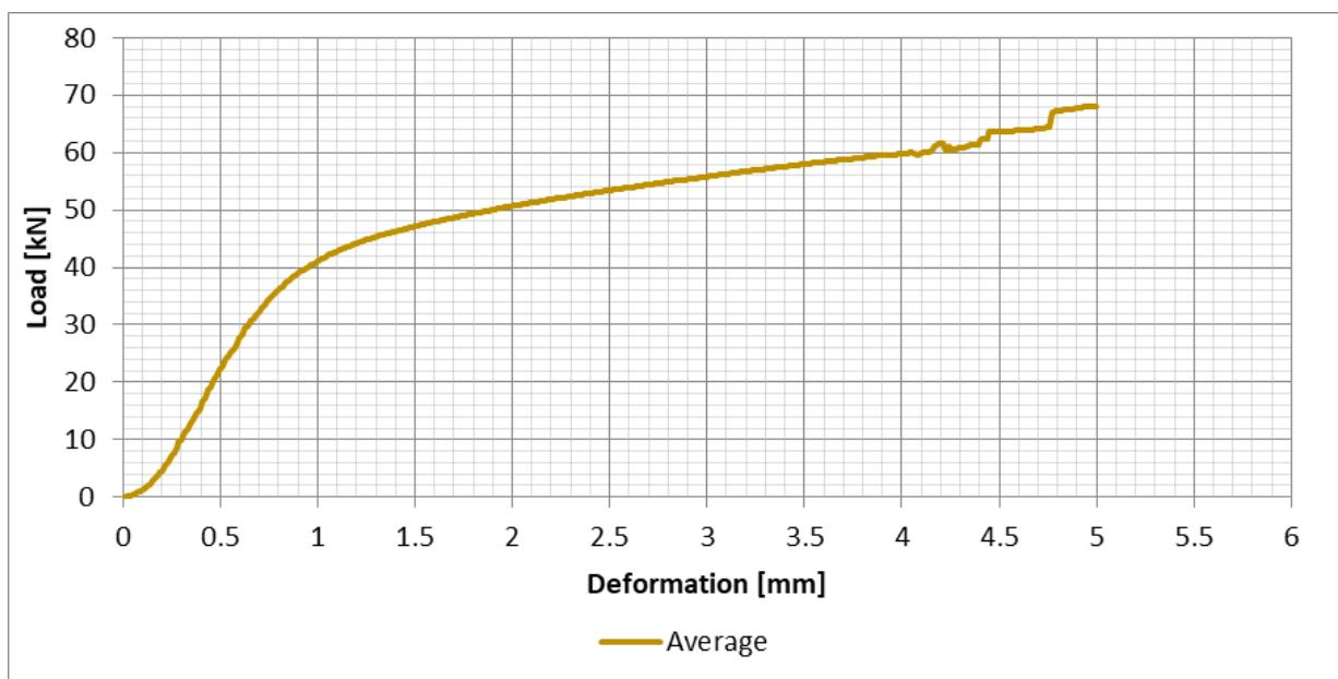
Figure 44: Radiata Pine (S8), Average of all test results – Perpendicular to the grain bearing - Load/Deformation
