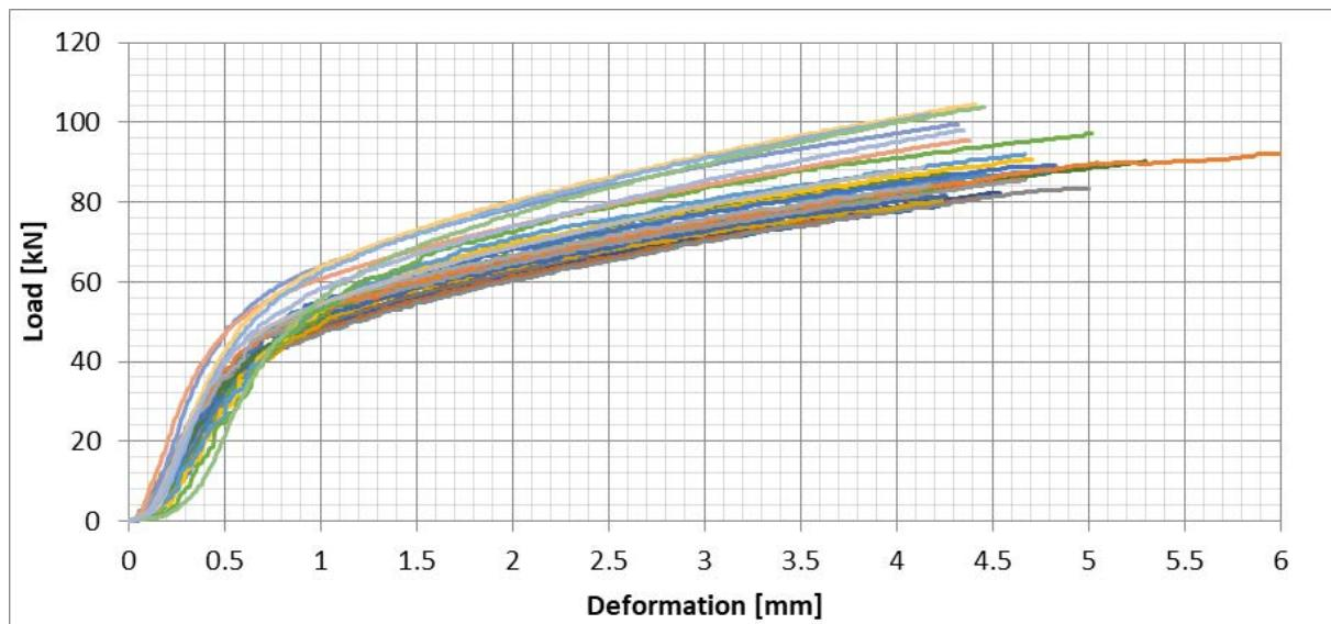
Figure 53: Alpine Ash (H1), All test results – Perpendicular to the grain bearing - Load/Deformation
