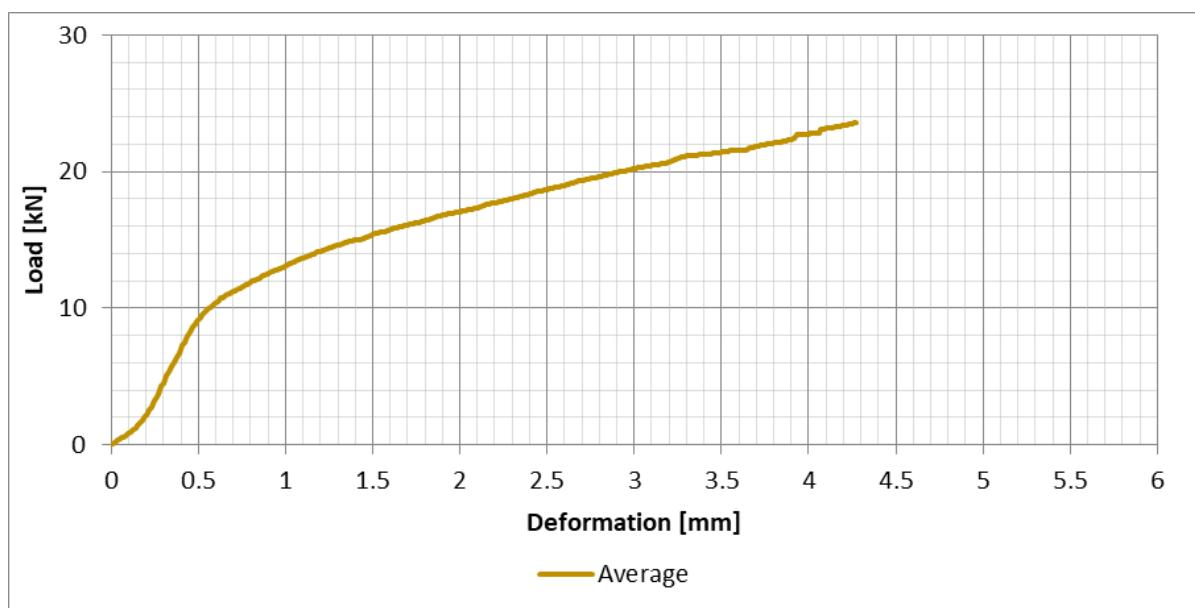
Figure 78: Scot Pine – 25 mm Bearing (Half studs) (I7), Average of all test results – Perpendicular to the grain bearing - Load/Deformation
