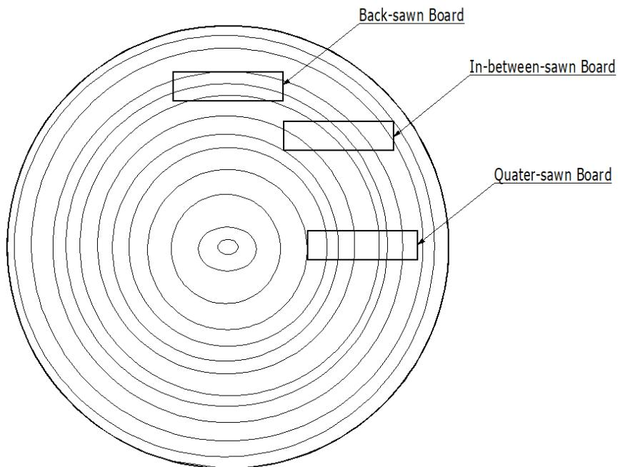
Figure A1: Sawn timber Cutting Directions
