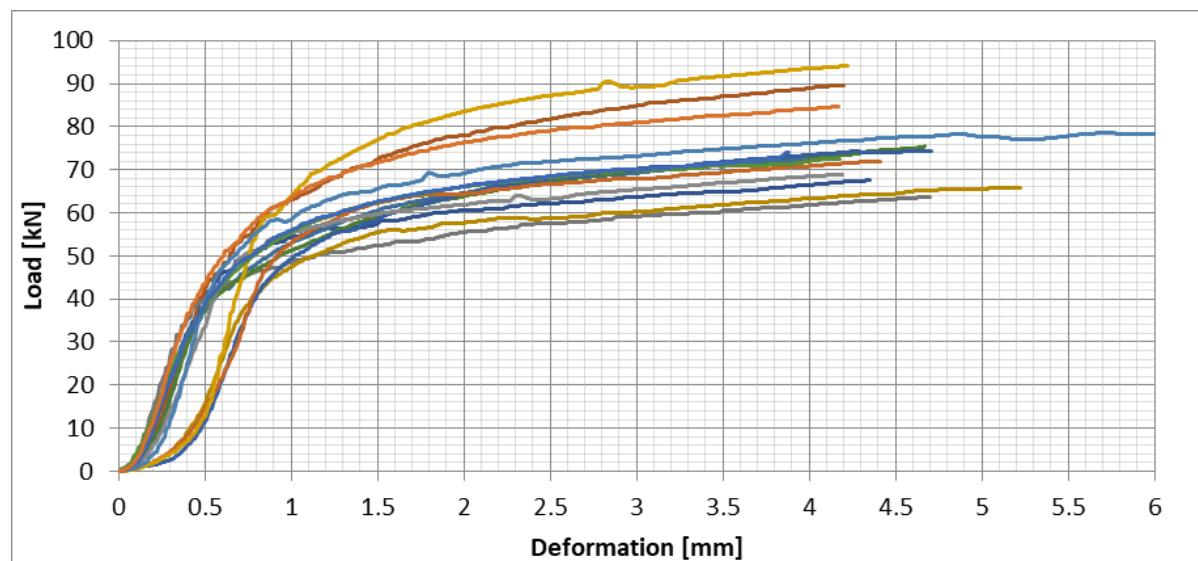
Figure 75: Scot Pine – 200 mm Bearing (Four studs) (I7), All test results – Perpendicular to the grain bearing - Load/Deformation
