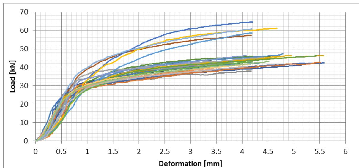
Figure 71: Scot Pine – 100 mm Bearing (Two studs) (I7), All test results – Perpendicular to the grain bearing - Load/Deformation
