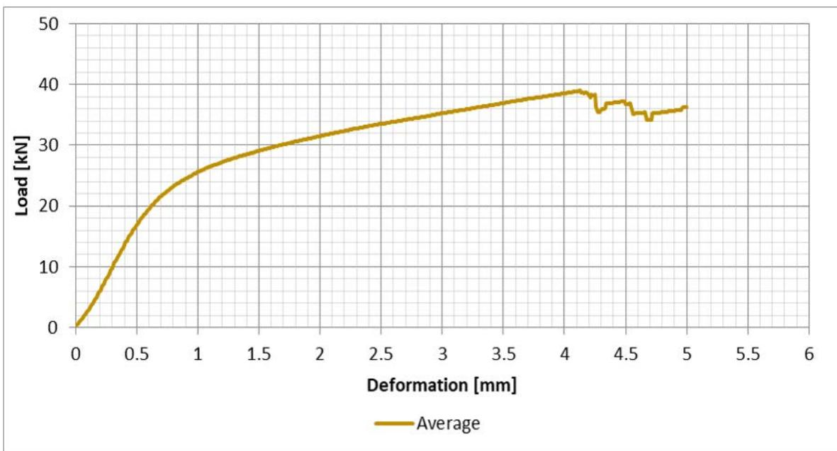
Figure 24: Douglas Fir (new) (I4), Average of all test results – Perpendicular to the grain bearing - Load/Deformation
