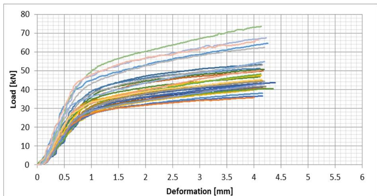
Figure 29: Radiata Pine (S1), All test results – Perpendicular to the grain bearing - Load/Deformation
