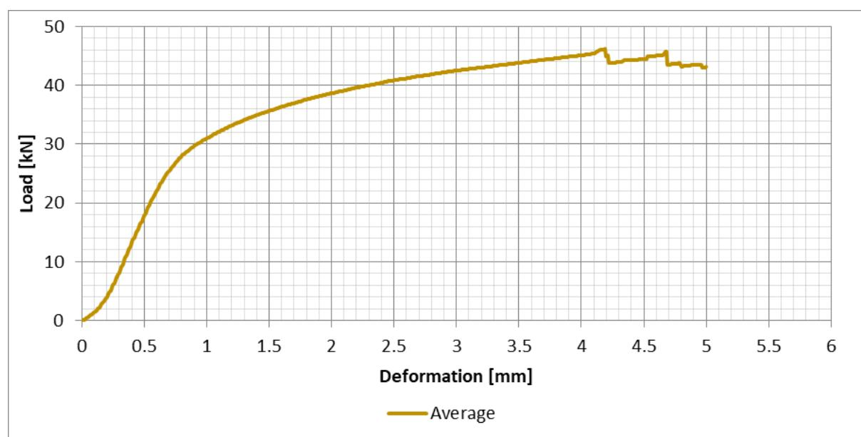
Figure 72: Scot Pine – 100 mm Bearing (Two studs) (I7), Average of all test results – Perpendicular to the grain bearing - Load/Deformation
