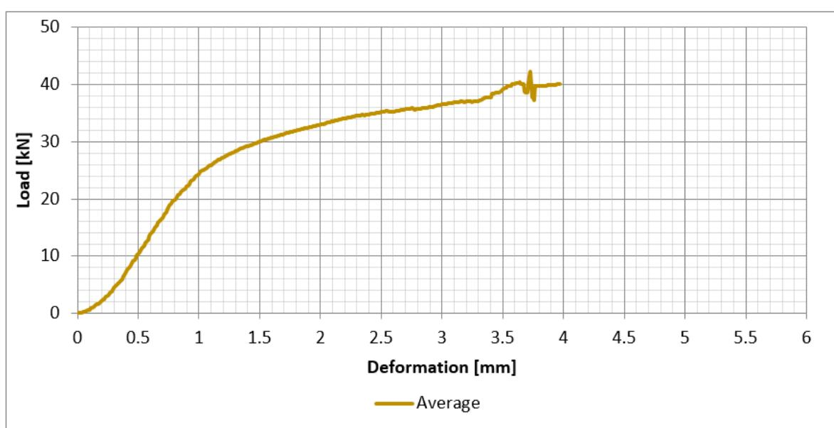
Figure 20: Scots Pine (I2), Average of all test results – Perpendicular to the grain bearing - Load/Deformation
