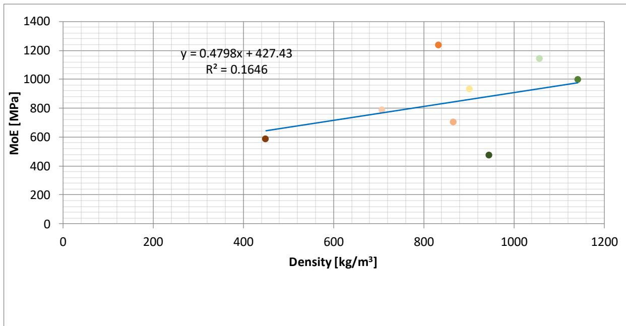
Figure 93: Average MoE Perpendicular to the grain against hardwood density
