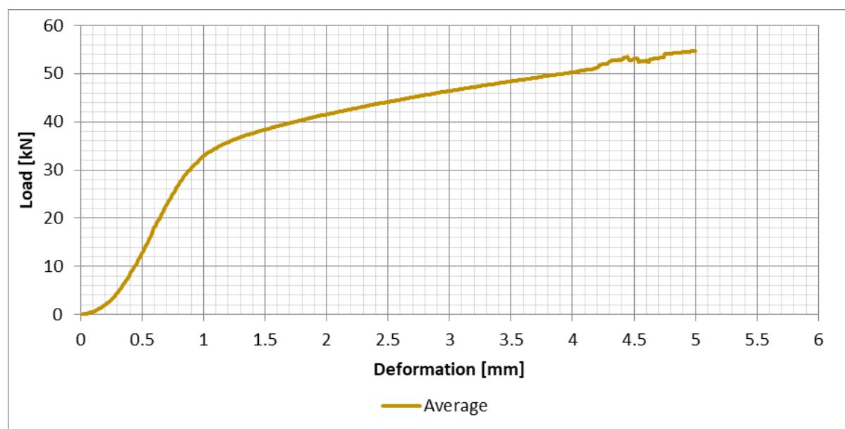
Figure 80: Radiata Pine – Middle of Plate (S10), Average of all test results – Perpendicular to the grain bearing - Load/Deformation
