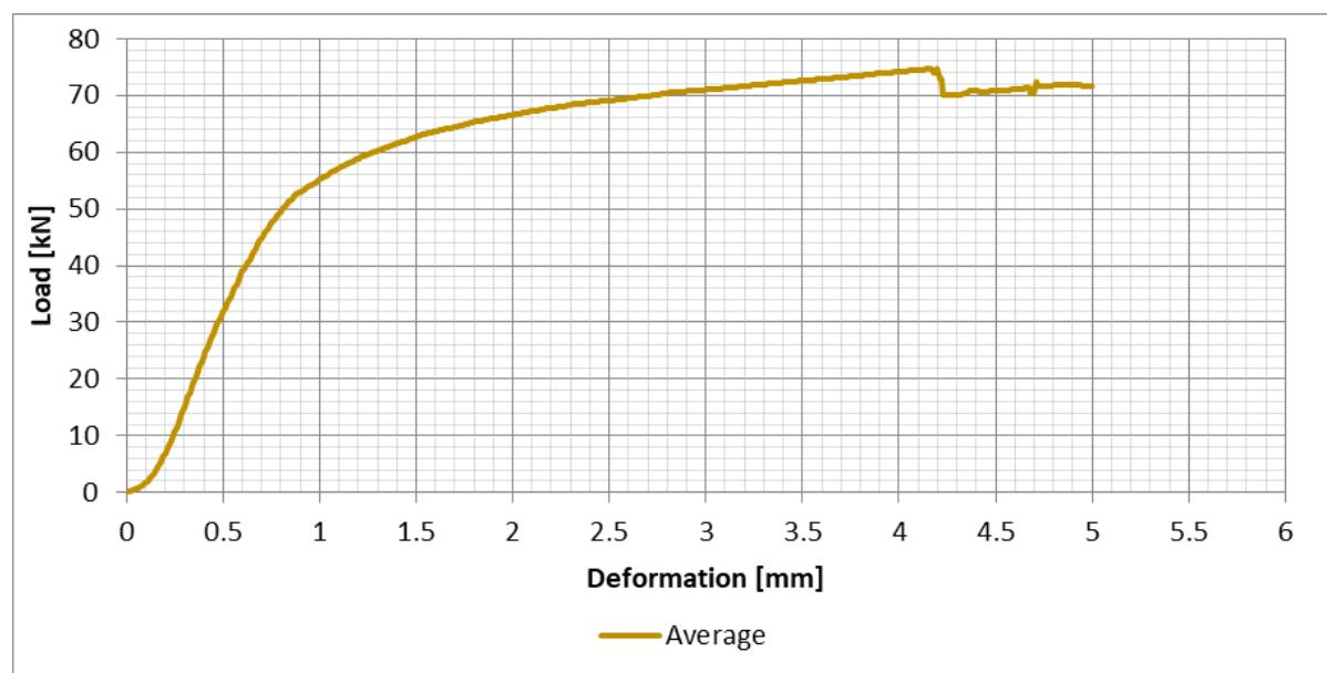
Figure 76: Scot Pine – 200 mm Bearing (Four studs) (I7), Average of all test results – Perpendicular to the grain bearing - Load/Deformation
