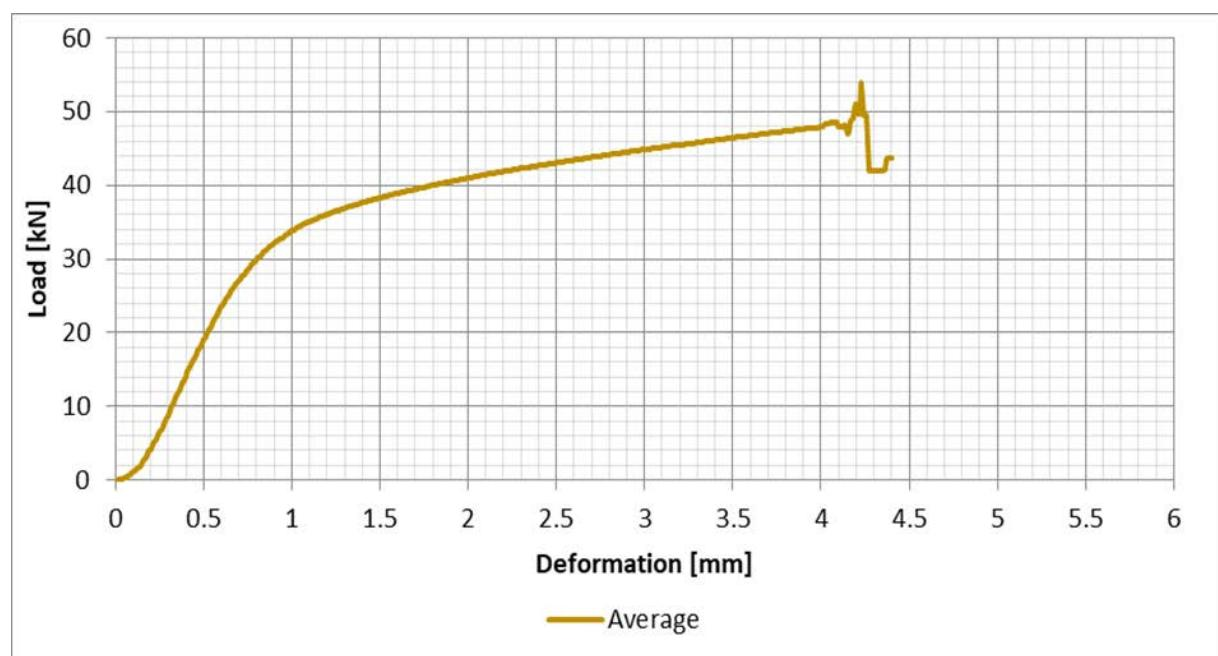
Figure 30: Radiata Pine (S1), Average of all test results – Perpendicular to the grain bearing - Load/Deformation
