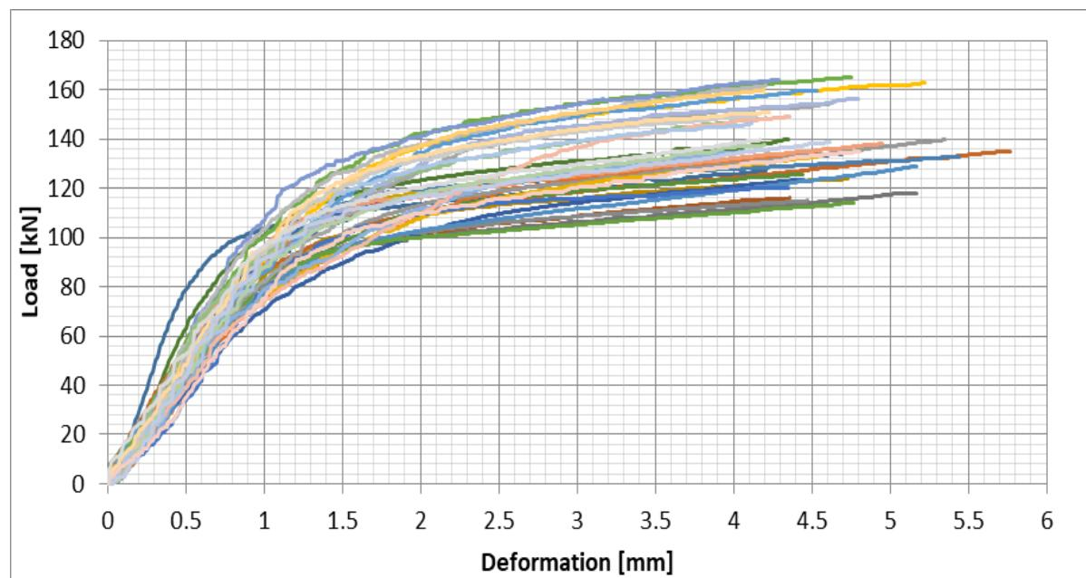
Figure 50: Caribbea Hybrid (S14), Average of all test results – Perpendicular to the grain bearing - Load/Deformation
