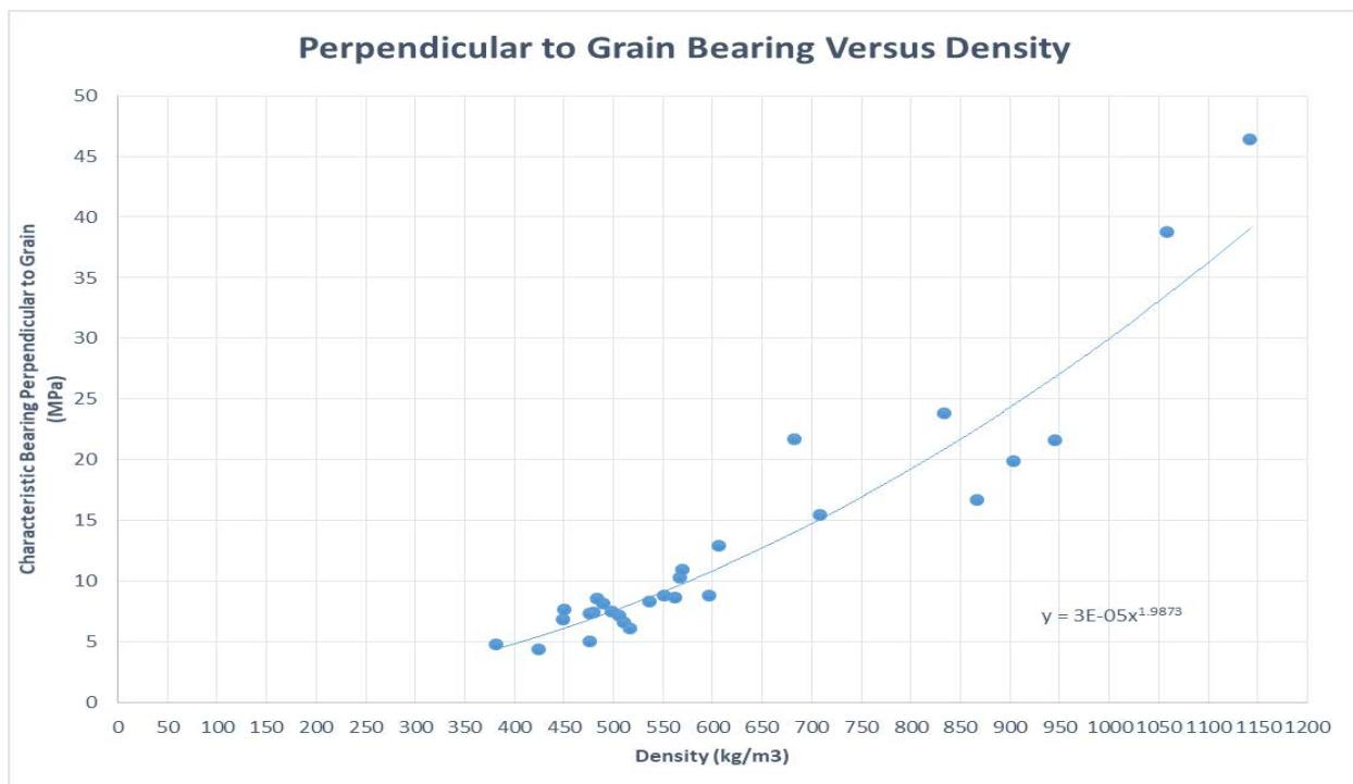
Figure 83: Characteristic perpendicular to the grain bearing values against the average density at 12% moisture
