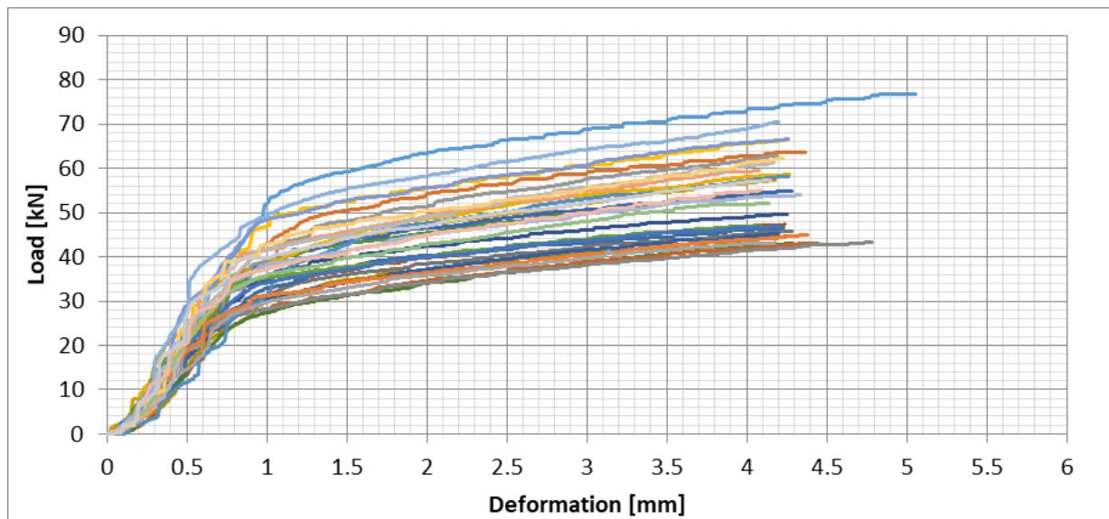
Figure 45: Radiata Pine (S11), All test results – Perpendicular to the grain bearing - Load/Deformation
