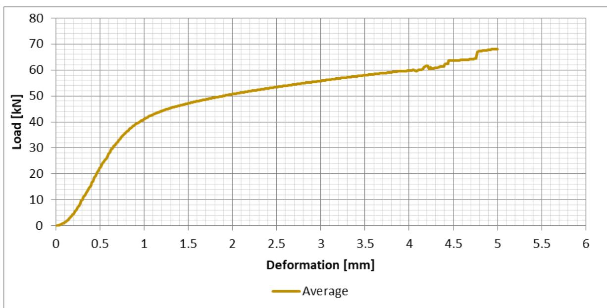
Figure 50: Caribbea Hybrid (S14), Average of all test results – Perpendicular to the grain bearing - Load/Deformation
