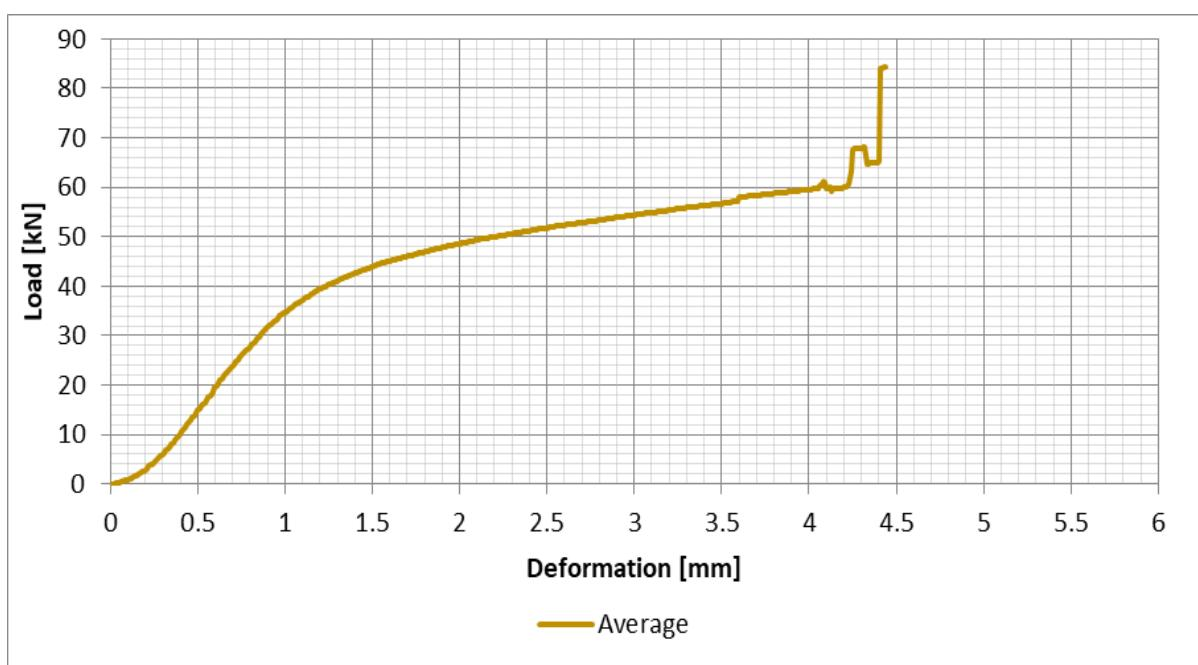
Figure 38: Radiata Pine (S5), Average of all test results – Perpendicular to the grain bearing - Load/Deformation
