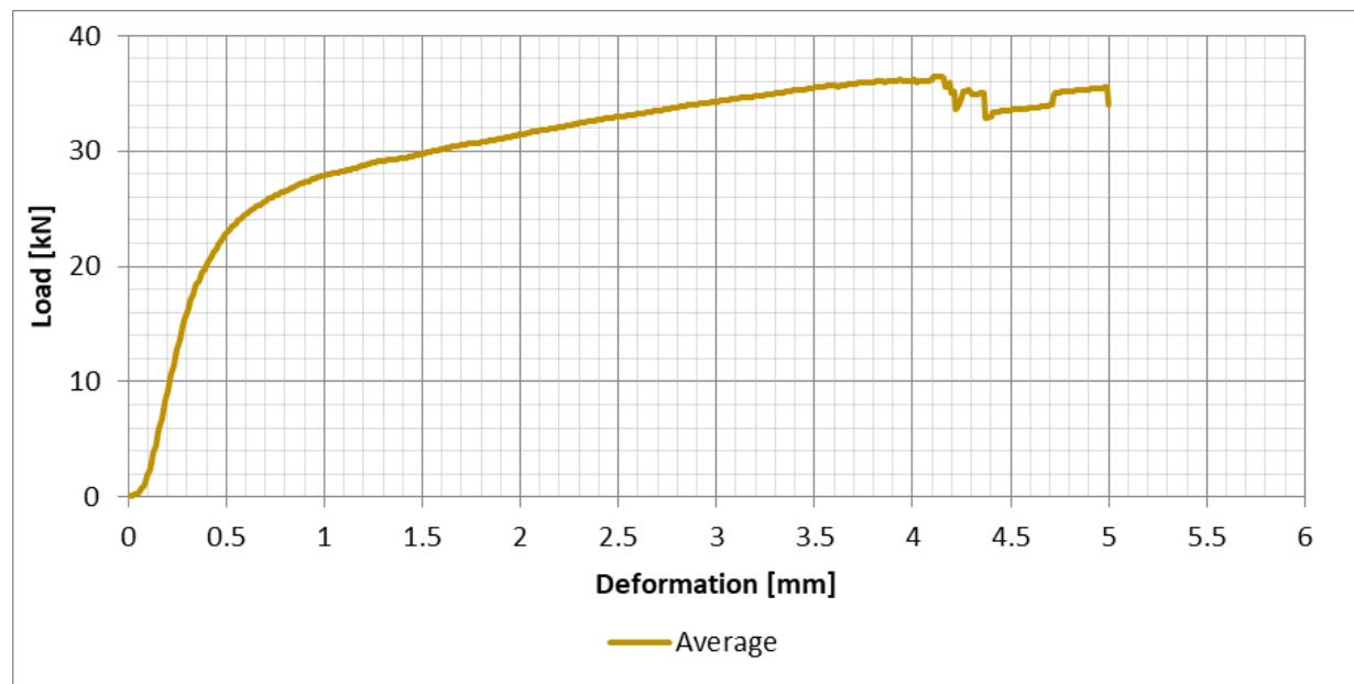
Figure 28: Western Red Cedar (I6), Average of all test results – Perpendicular to the grain bearing - Load/Deformation
