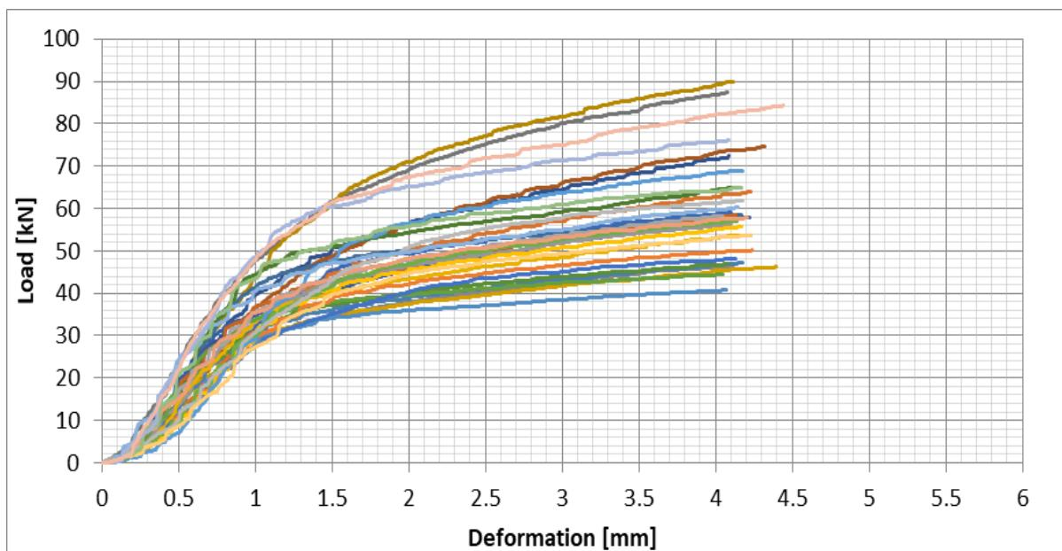
Figure 37: Radiata Pine (S5), All test results – Perpendicular to the grain bearing - Load/Deformation
