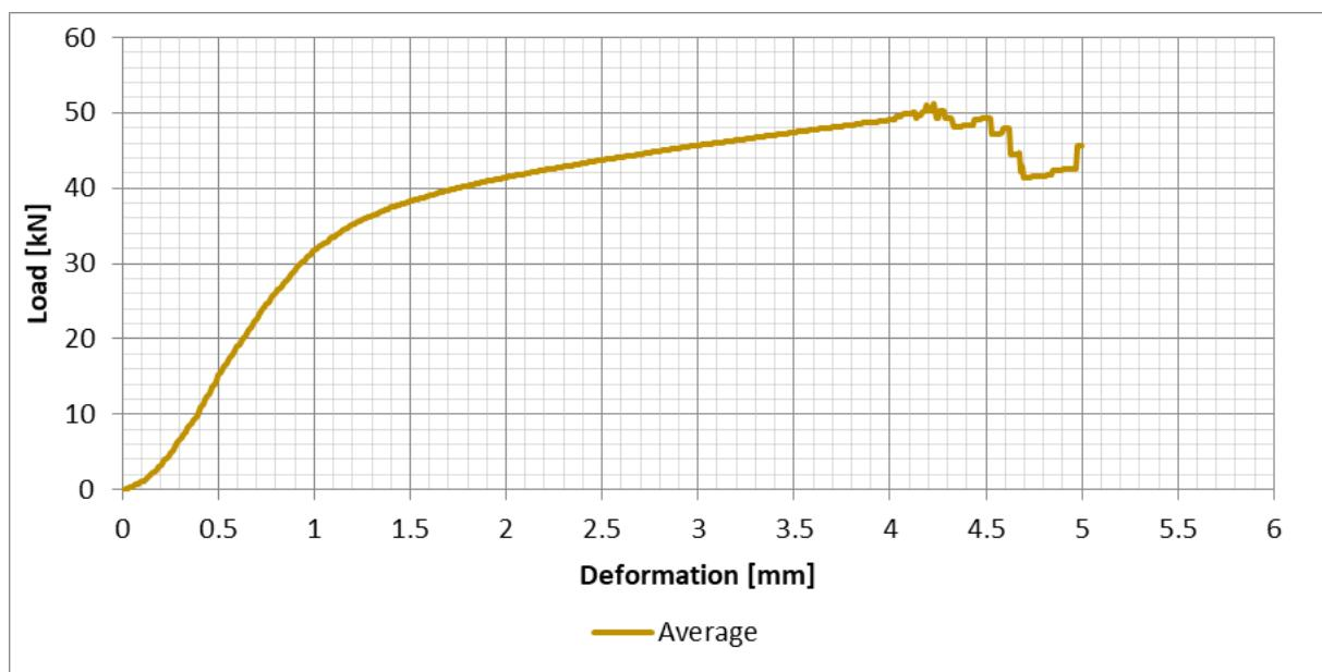
Figure 34: Radiata Pine (S3), Average of all test results – Perpendicular to the grain bearing - Load/Deformation
