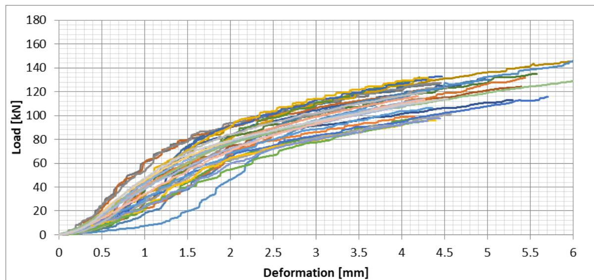
Figure 65: Southern Mahogany (H9), All test results – Perpendicular to the grain bearing - Load/Deformation
