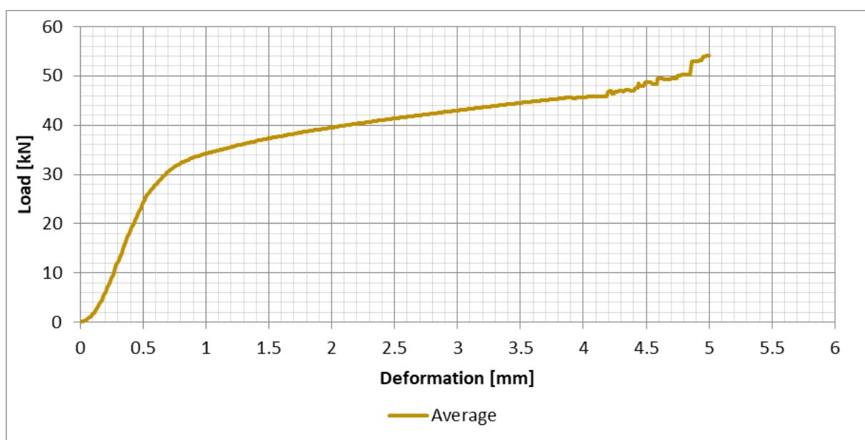
Figure 68: Meranti, Light red (H10), Average of all test results – Perpendicular to the grain bearing - Load/Deformation
