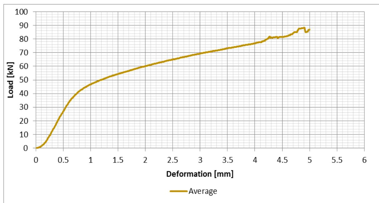
Figure 42: Radiata Pine (S7), Average of all test results – Perpendicular to the grain bearing - Load/Deformation
