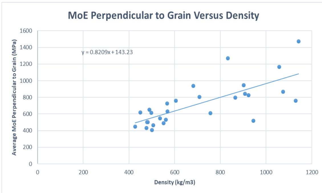
**Figure 94: Average MoE Perpendicular to Grain versus Timber Density at 12 % MC**
