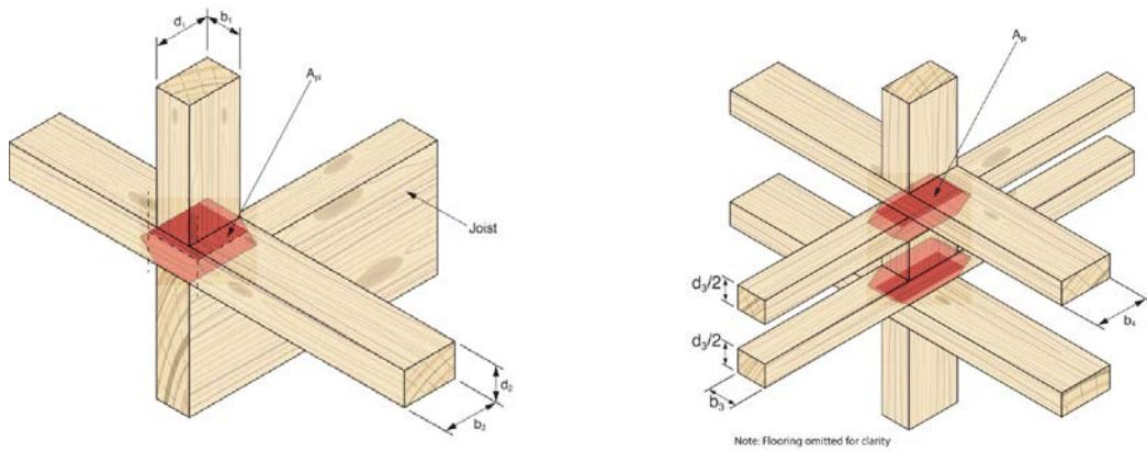
**Figure 6.2b – Bearing in top plate (left) and top and bottom floor truss (right)**
