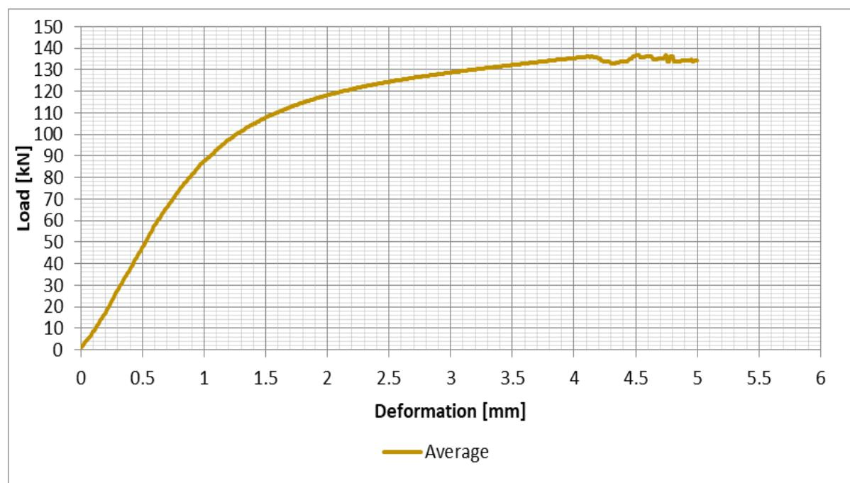
Figure 52: Cypress (S17), Average of all test results – Perpendicular to the grain bearing - Load/Deformation
