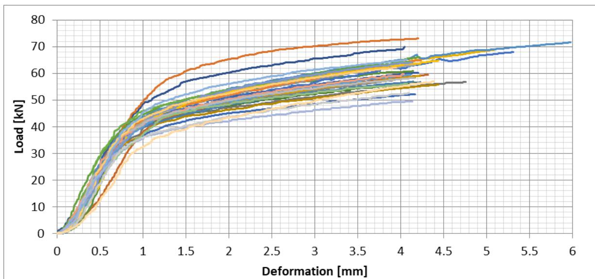
Figure 43: Radiata Pine (S8), All test results – Perpendicular to the grain bearing - Load/Deformation
