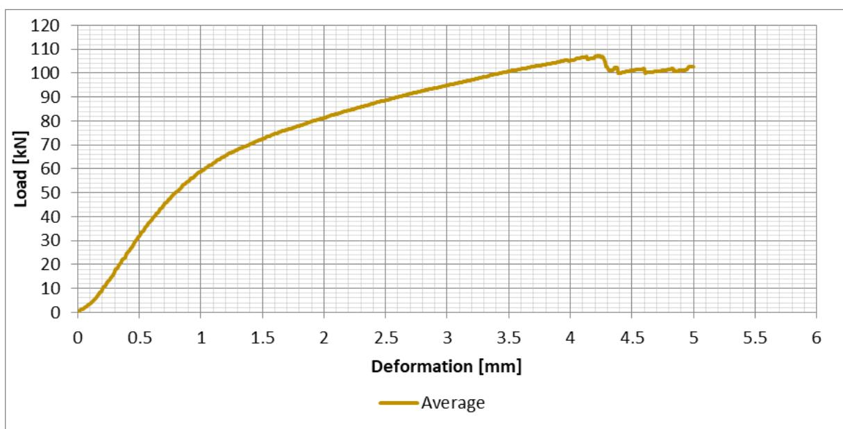
Figure 58: Karri (H5), Average of all test results – Perpendicular to the grain bearing - Load/Deformation
