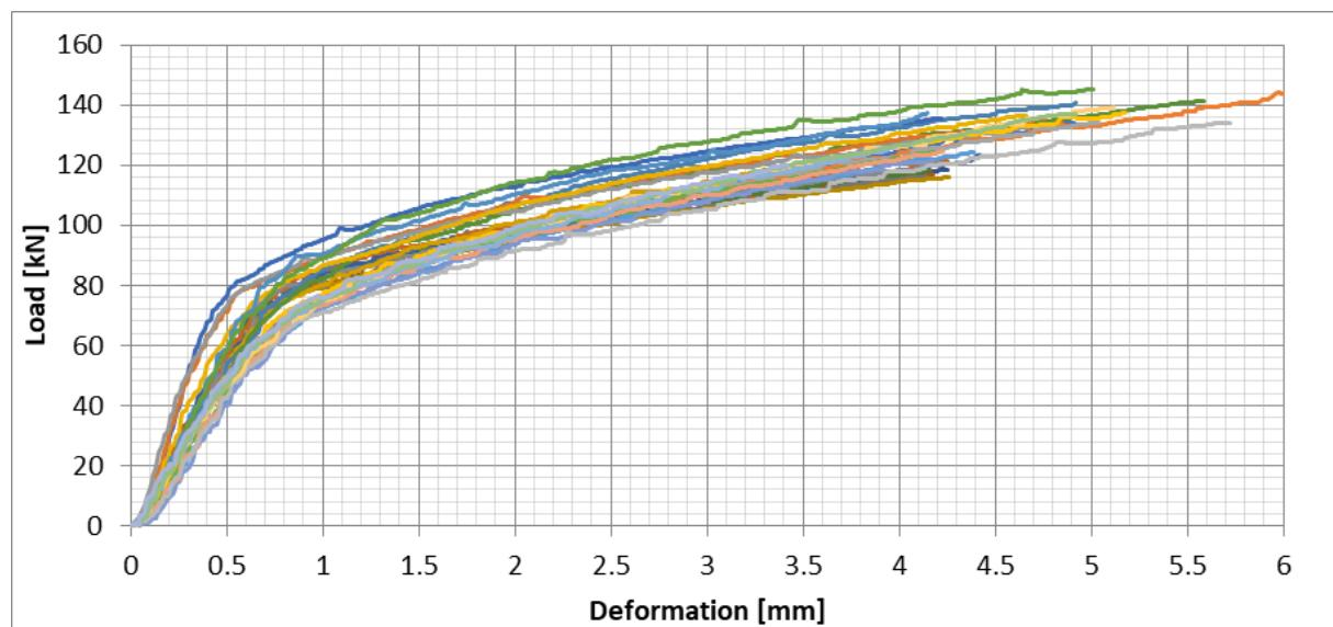
Figure 55: Jarrah (H4), All test results – Perpendicular to the grain bearing - Load/Deformation
