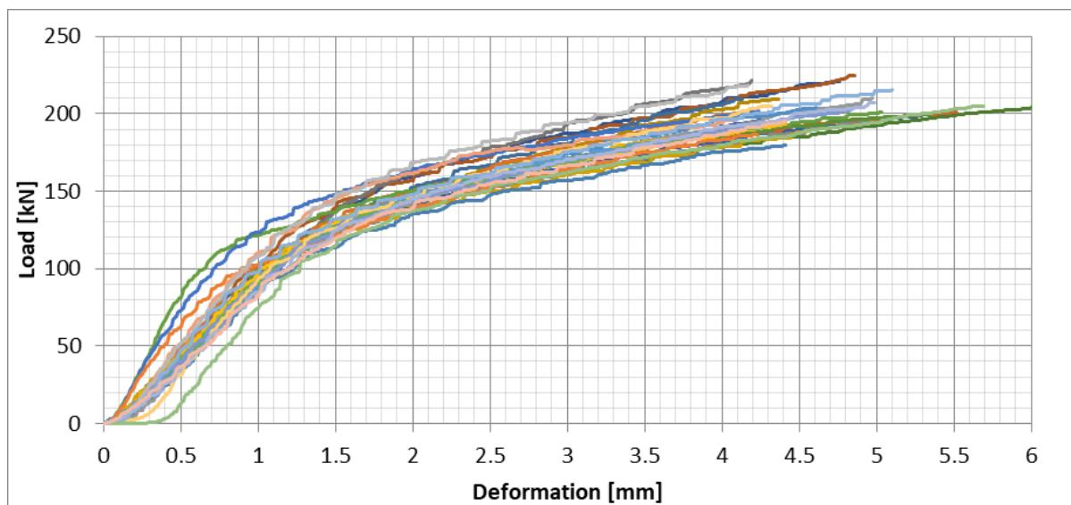
Figure 63: Spotted Gum (H8), All test results – Perpendicular to the grain bearing - Load/Deformation
