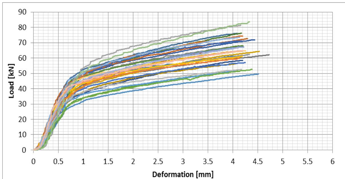
Figure 39: Radiata Pine (S6), All test results – Perpendicular to the grain bearing - Load/Deformation
