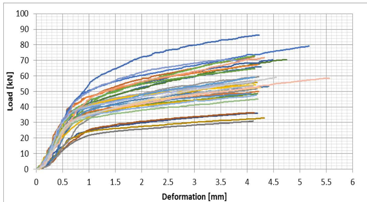
Figure 31: Radiata Pine (S2), All test results – Perpendicular to the grain bearing - Load/Deformation
