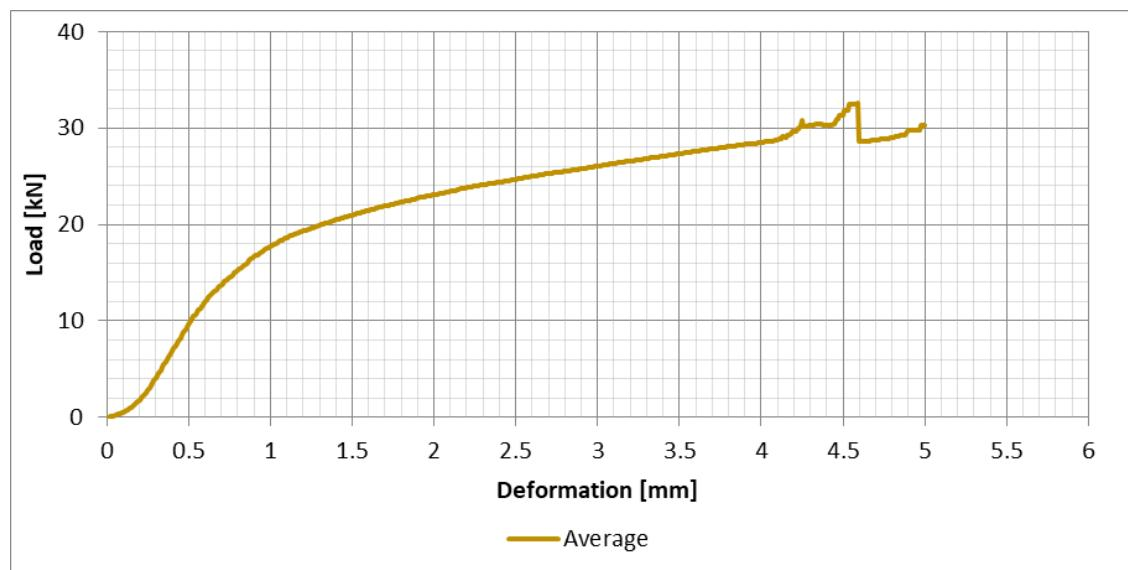
Figure 70: Scot Pine – 48 mm Bearing (one stud) (I7), Average of all test results – Perpendicular to the grain bearing - Load/Deformation
