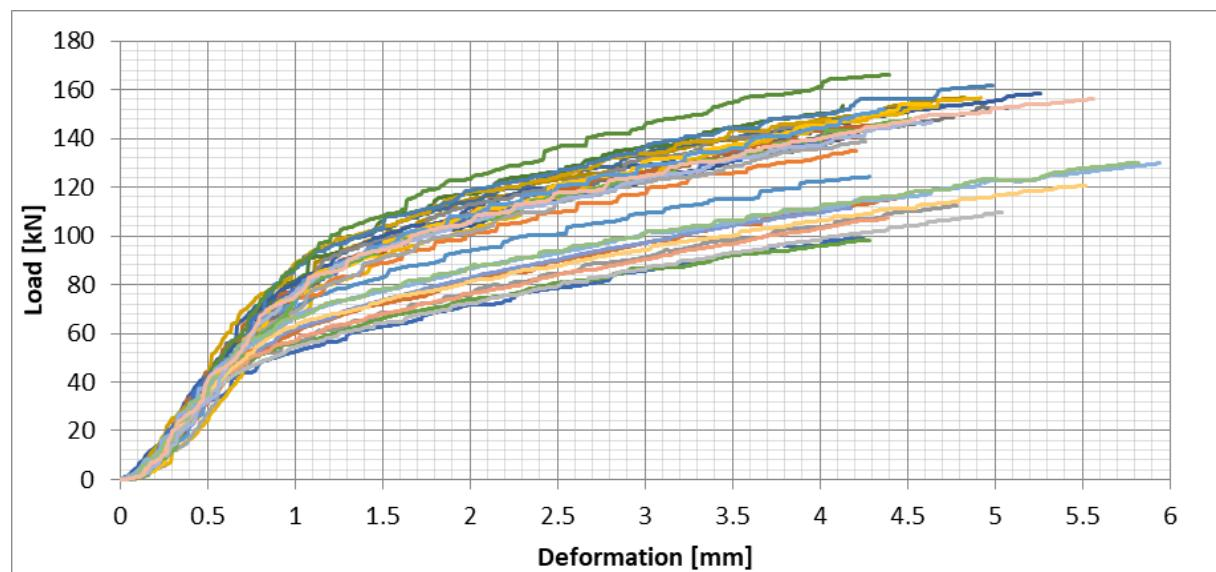
Figure 59: Blackbutt (H6), All test results – Perpendicular to the grain bearing - Load/Deformation
