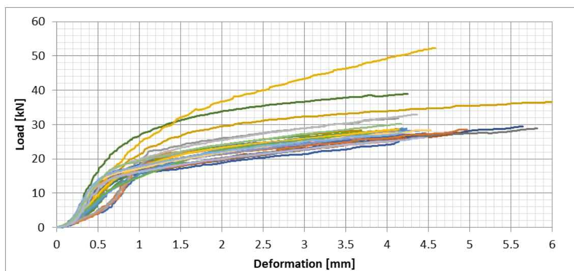
Figure 69: Scot Pine – 48 mm Bearing (one stud) (I7), All test results – Perpendicular to the grain bearing - Load/Deformation
