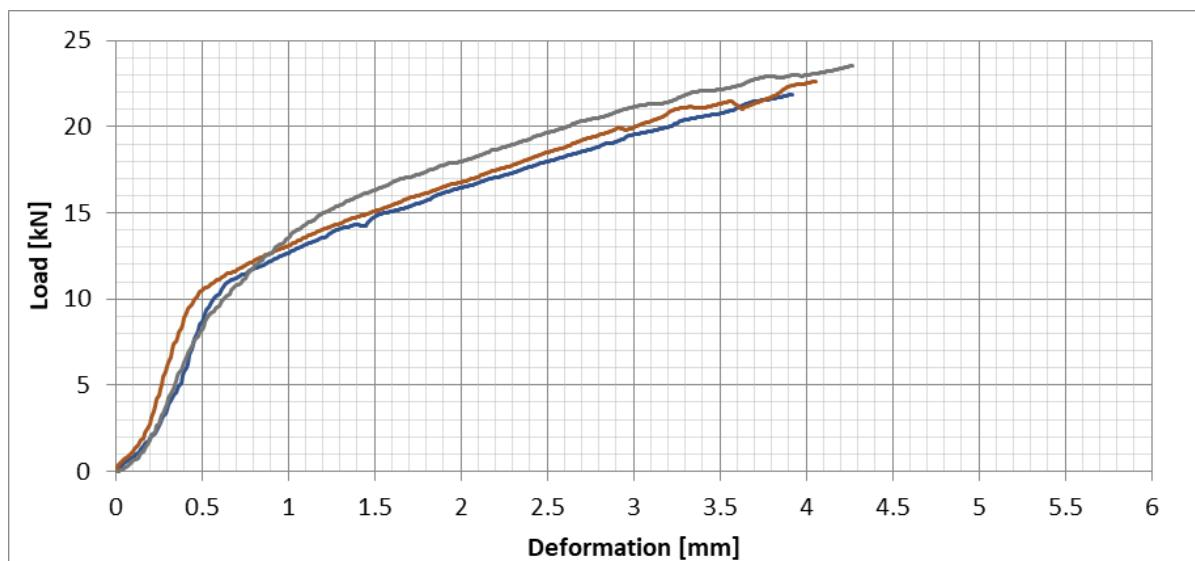
Figure 77: Scot Pine – 25 mm Bearing (Half studs) (I7), All test results – Perpendicular to the grain bearing - Load/Deformation
