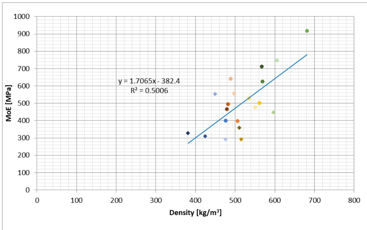
Figure 92: Average MoE Perpendicular to the grain against softwood density
