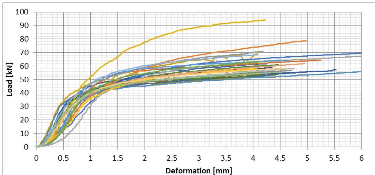
Figure 73: Scot Pine – 150 mm Bearing (Three studs) (I7), All test results – Perpendicular to the grain bearing - Load/Deformation
