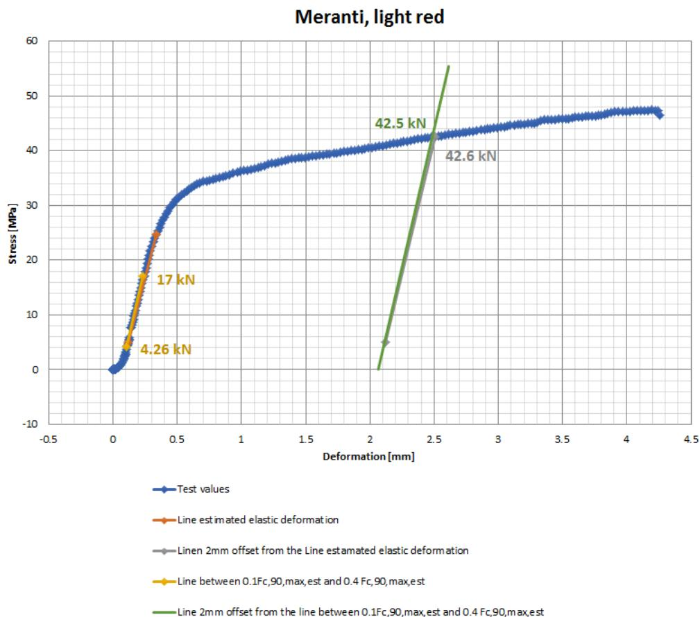
Figure 1B: Load-deformation curve for compression perpendicular to the grain for Meranti
