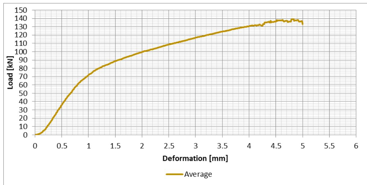
Figure 60: Blackbutt (H6), Average of all test results – Perpendicular to the grain bearing - Load/Deformation
