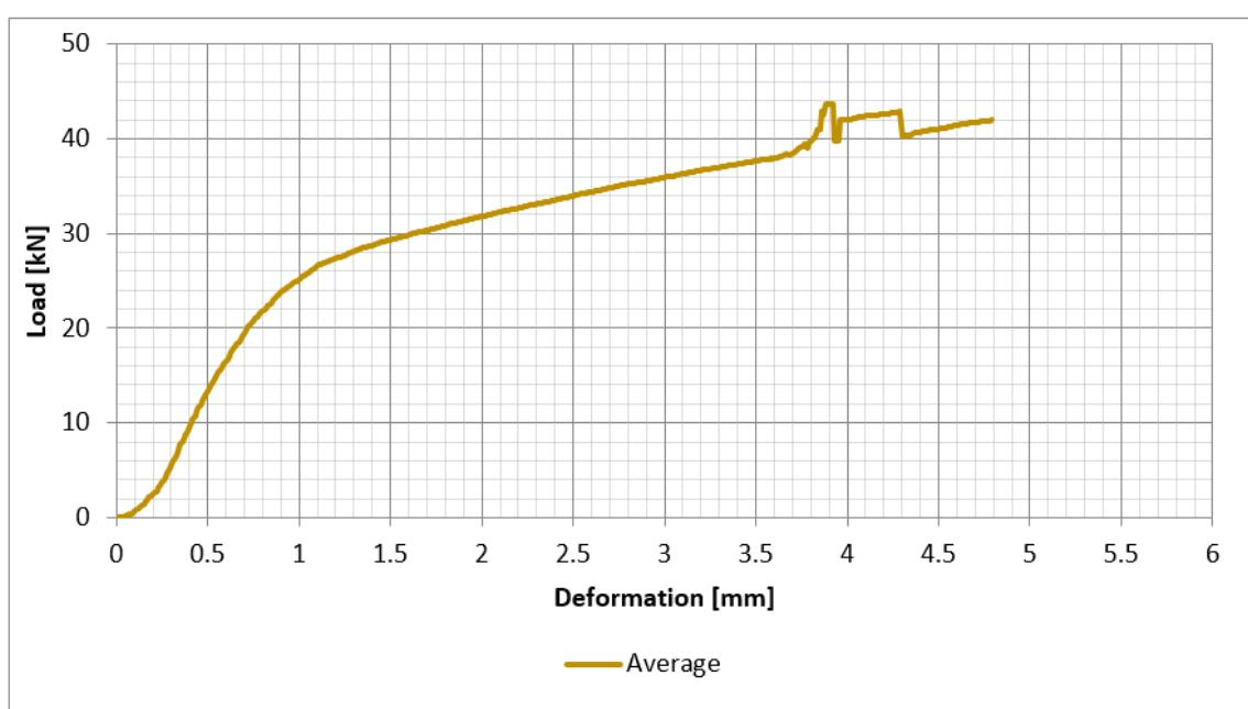
Figure 18: Spruce (I1), Average of all test results – Perpendicular to the grain bearing - Load/Deformation
