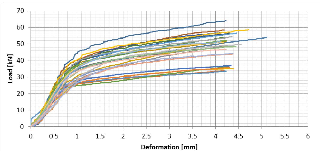
Figure 47: Radiata Pine (S12), All test results – Perpendicular to the grain bearing - Load/Deformation
