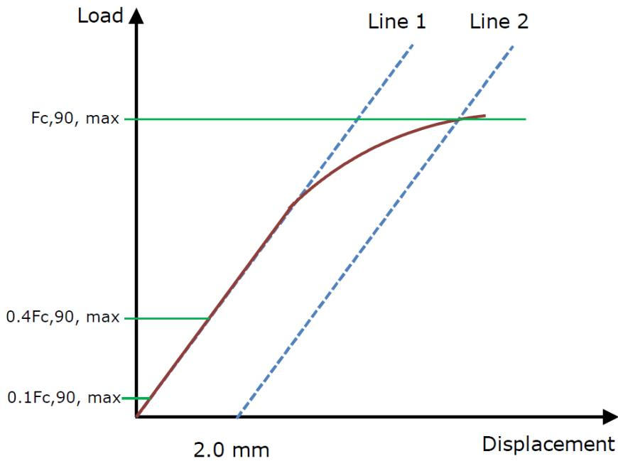
Figure 16: Load-deformation curve for compression perpendicular to the grain, definition of compression strength  $F_{c,90,max}$  at 2.0 mm off-set
