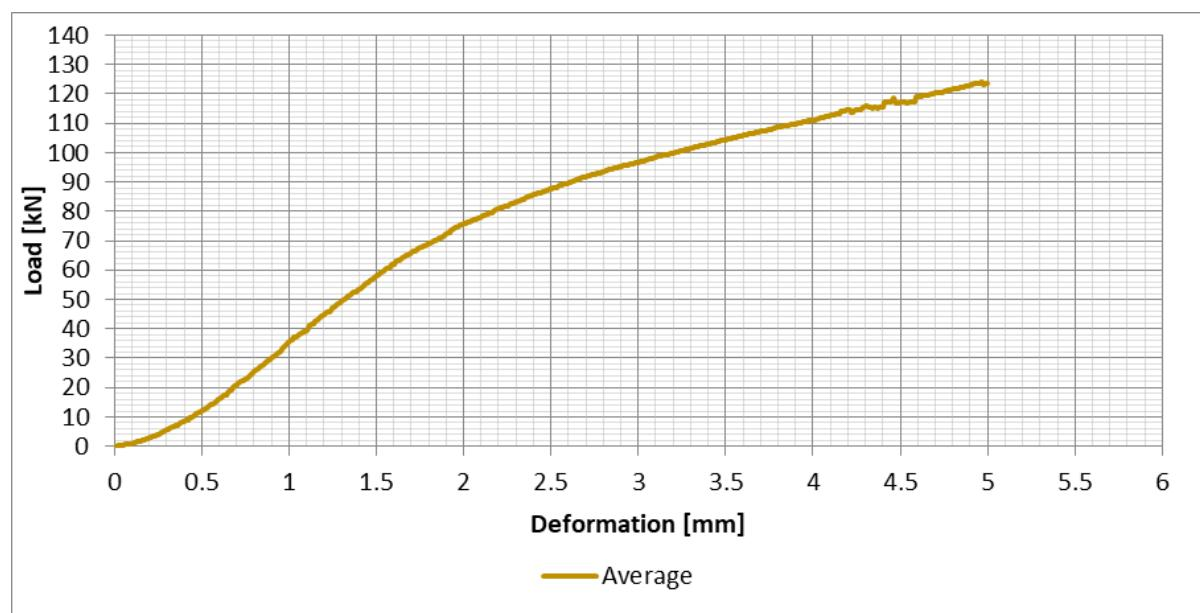
Figure 66: Southern Mahogany (H9), Average of all test results – Perpendicular to the grain bearing - Load/Deformation
