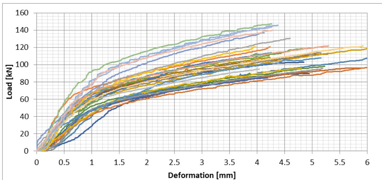
Figure 57: Karri (H5), All test results – Perpendicular to the grain bearing - Load/Deformation
