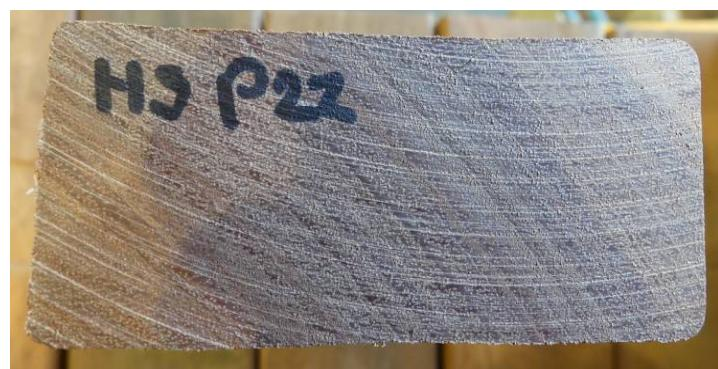
Figure A3: Cross section of sample Southern Mahogany showing cupping
