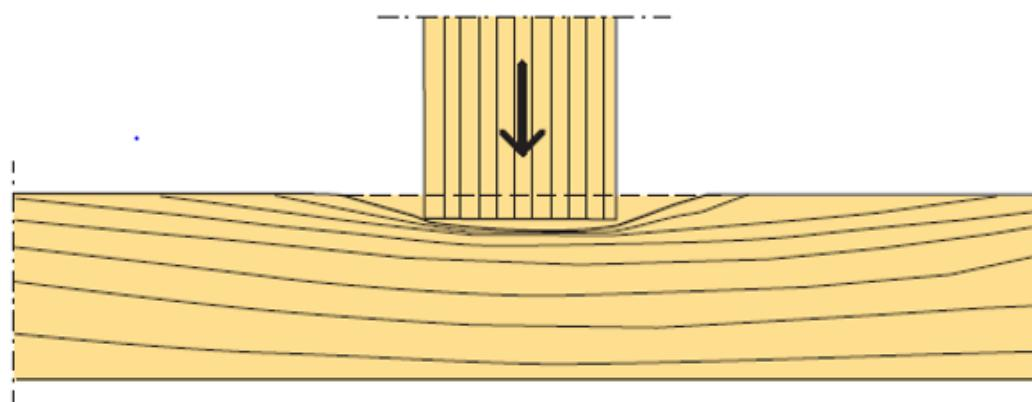
**Figure 88: Perpendicular to grain bearing (Swedish Wood, 2015)**
