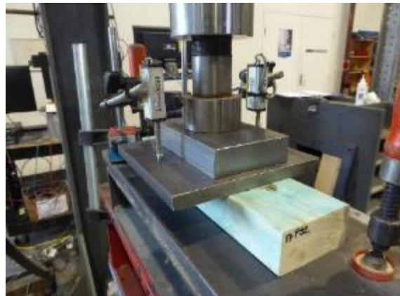
Figure 6: Four studs test set up
