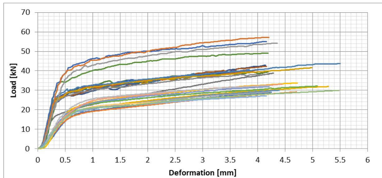
Figure 27: Western Red Cedar (I6), All test results – Perpendicular to the grain bearing - Load/Deformation
