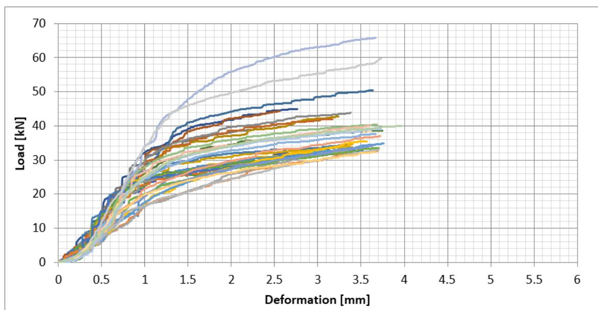
Figure 19: Spruce (I1), All test results – Perpendicular to the grain bearing - Load/Deformation
