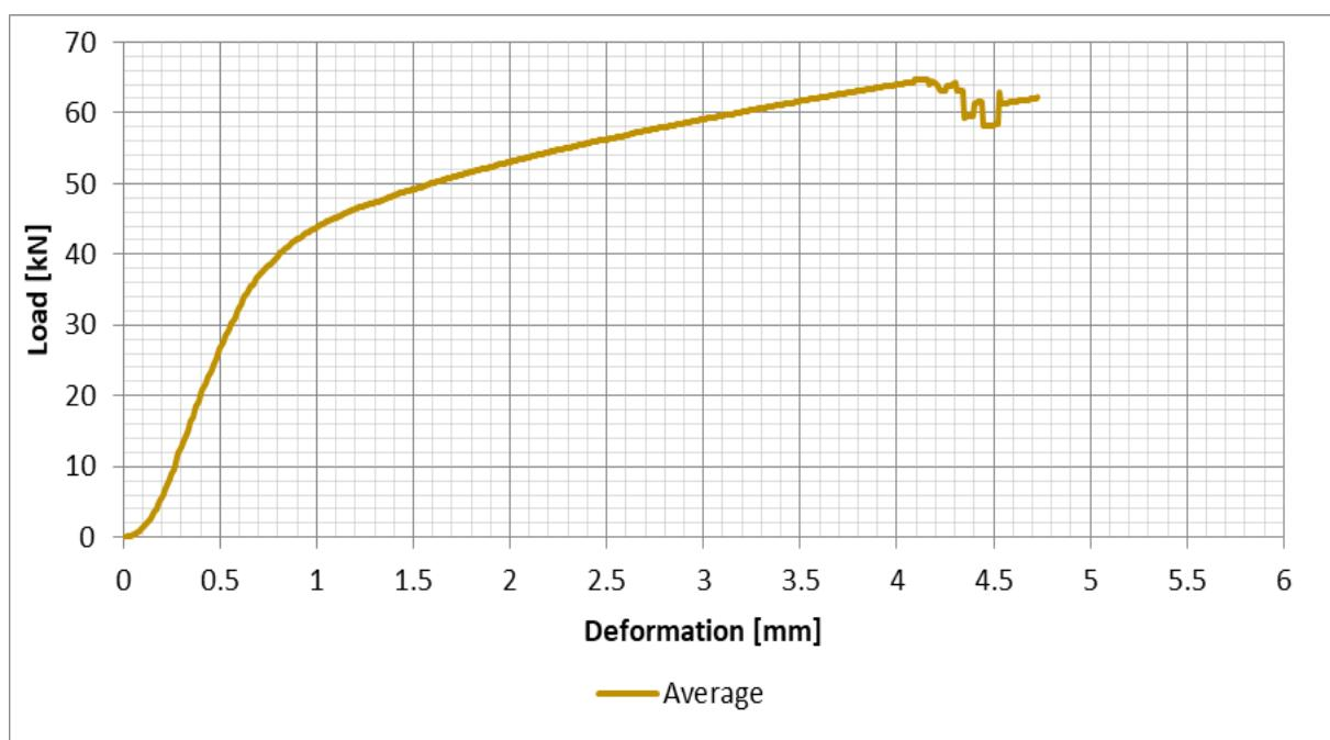
Figure 40: Radiata Pine (S6), Average of all test results – Perpendicular to the grain bearing - Load/Deformation
