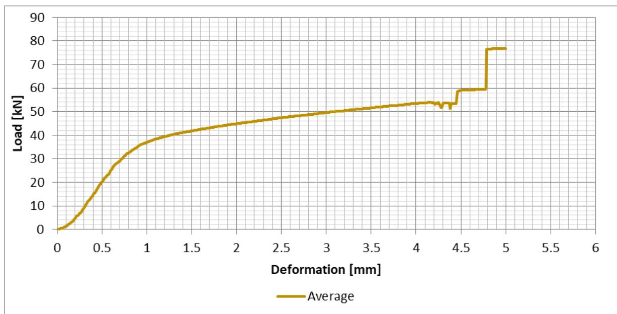
Figure 46: Radiata Pine (S11), Average of all test results – Perpendicular to the grain bearing - Load/Deformation
