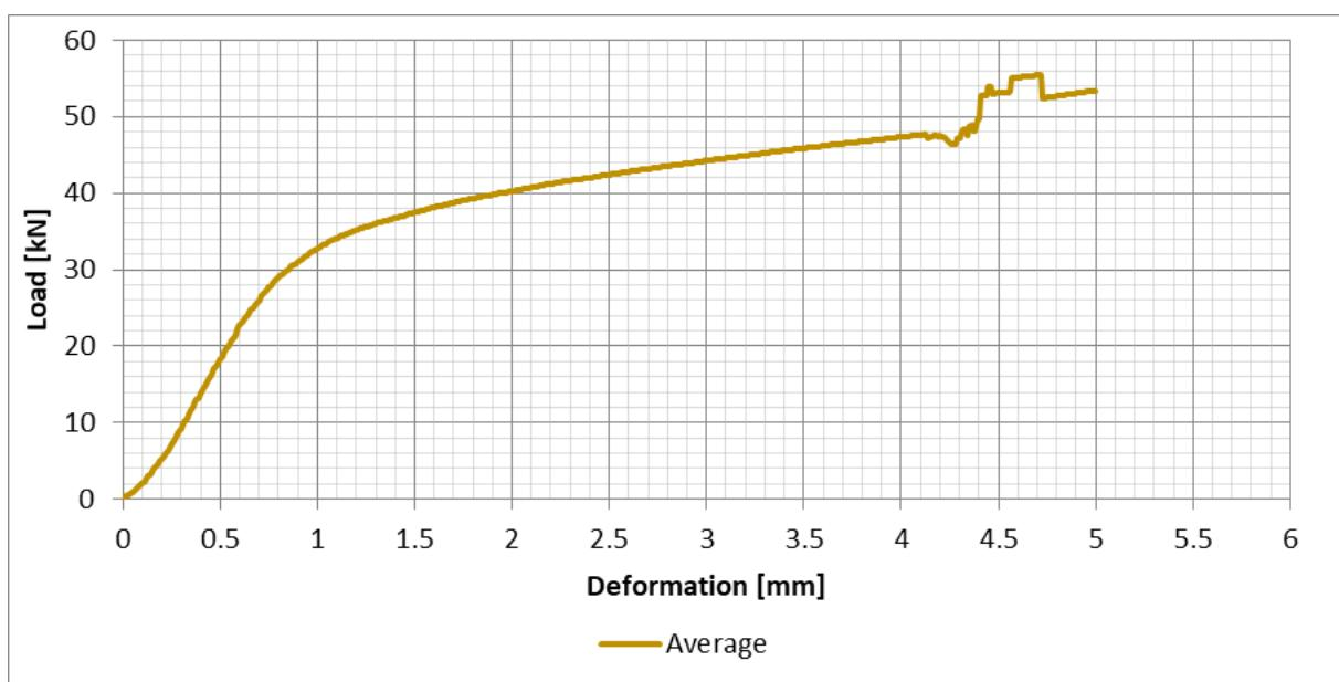
Figure 48: Radiata Pine (S12), Average of all test results – Perpendicular to the grain bearing - Load/Deformation
