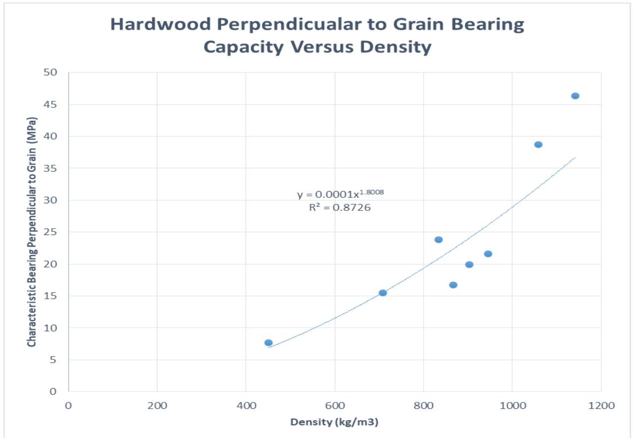
Figure 85: Hardwood Characteristic Perpendicular to Grain Bearing against Density at 12% moisture
