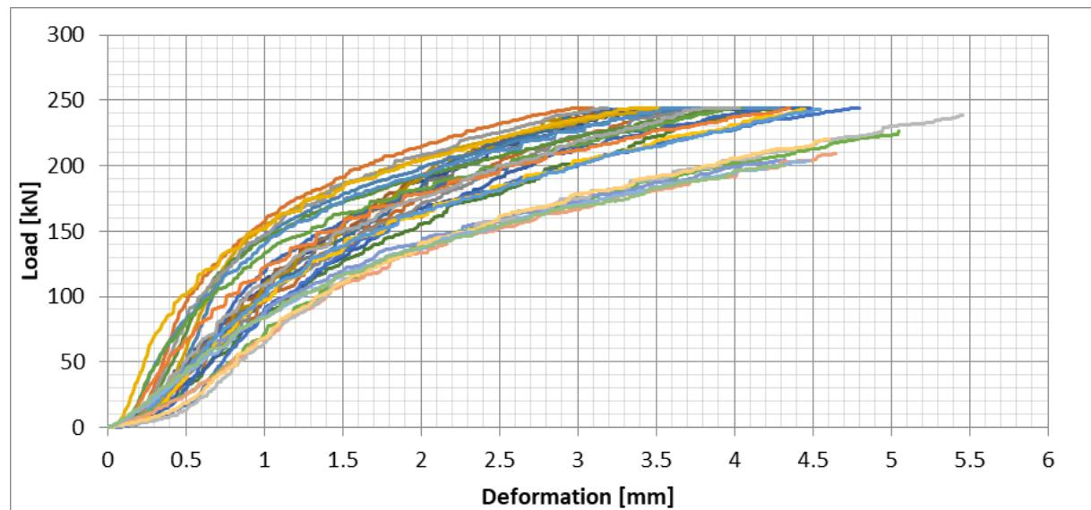
Figure 60: Blackbutt (H6), Average of all test results – Perpendicular to the grain bearing - Load/Deformation
