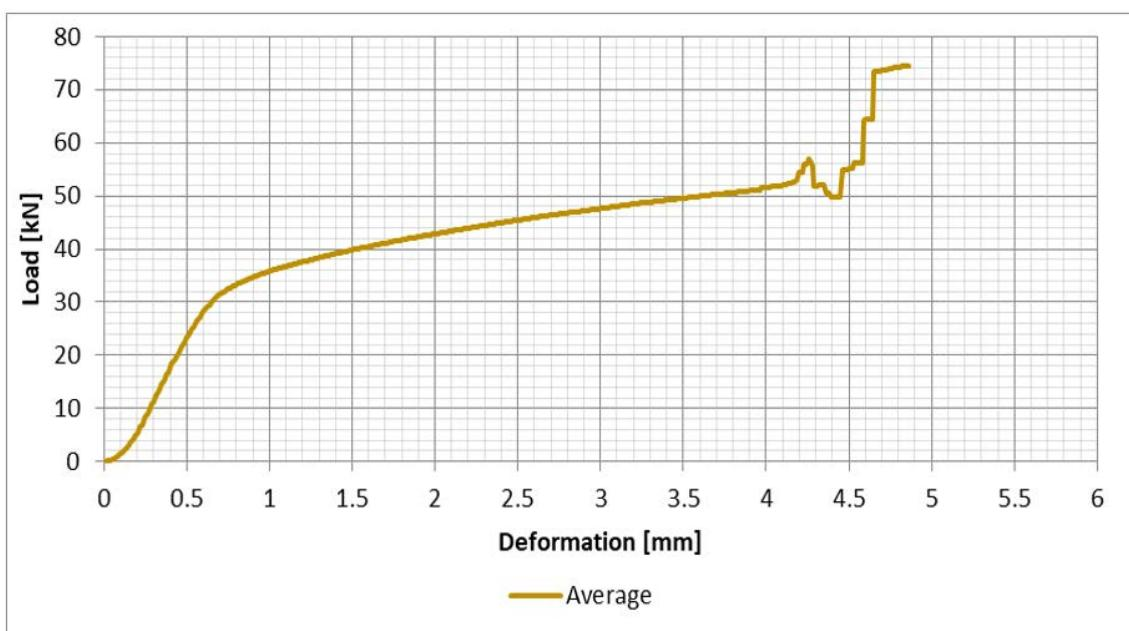
Figure 22: Radiata Pine New Zealand (I3), Average of all test results – Perpendicular to the grain bearing - Load/Deformation
