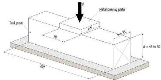
Figure 4: Bearing test configuration
