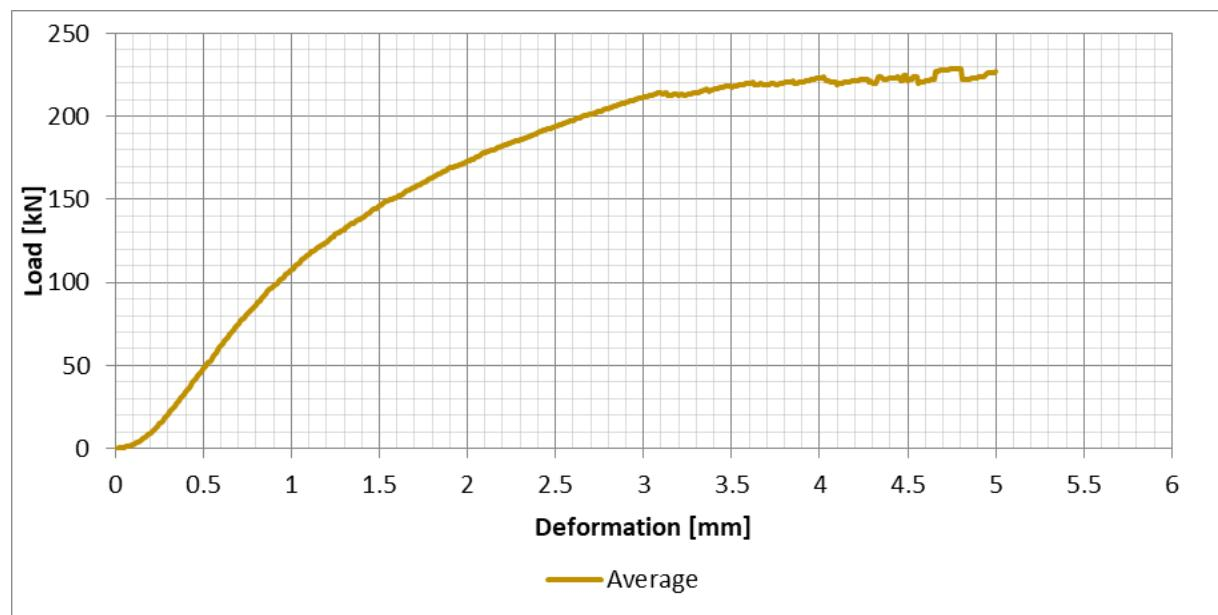
Figure 62: Grey Ironbark (H6), Average of all test results – Perpendicular to the grain bearing - Load/Deformation
