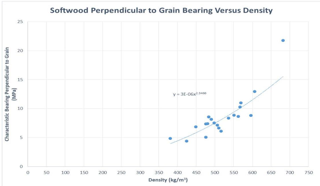
Figure 84: Softwood's Characteristic Perpendicular to the Grain Bearing against Density at 12% moisture
