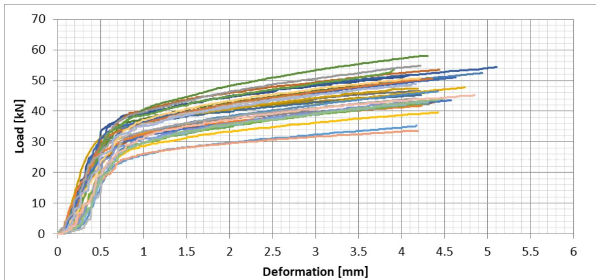
Figure 67: Southern Mahogany (H9), Average of all test results – Perpendicular to the grain bearing - Load/Deformation
