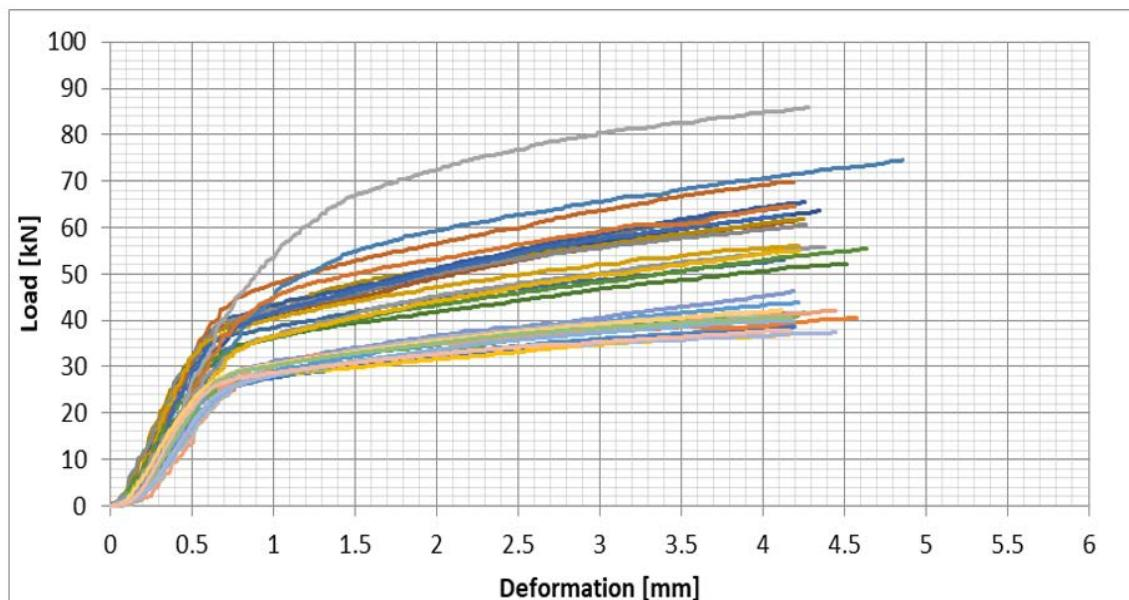
Figure 21: Radiata Pine New Zealand (I3), All test results – Perpendicular to the grain bearing - Load/Deformation
