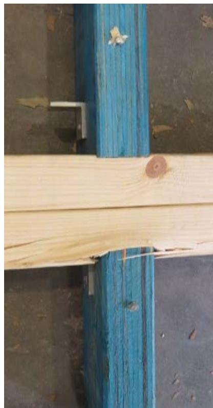
Figure 1: Crushing of wall plate after buckling of the wall stud has occurred
