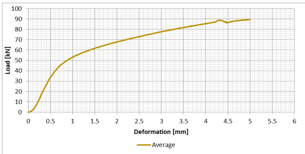
Figure 54: Alpine Ash (H1), Average of all test results – Perpendicular to the grain bearing - Load/Deformation
