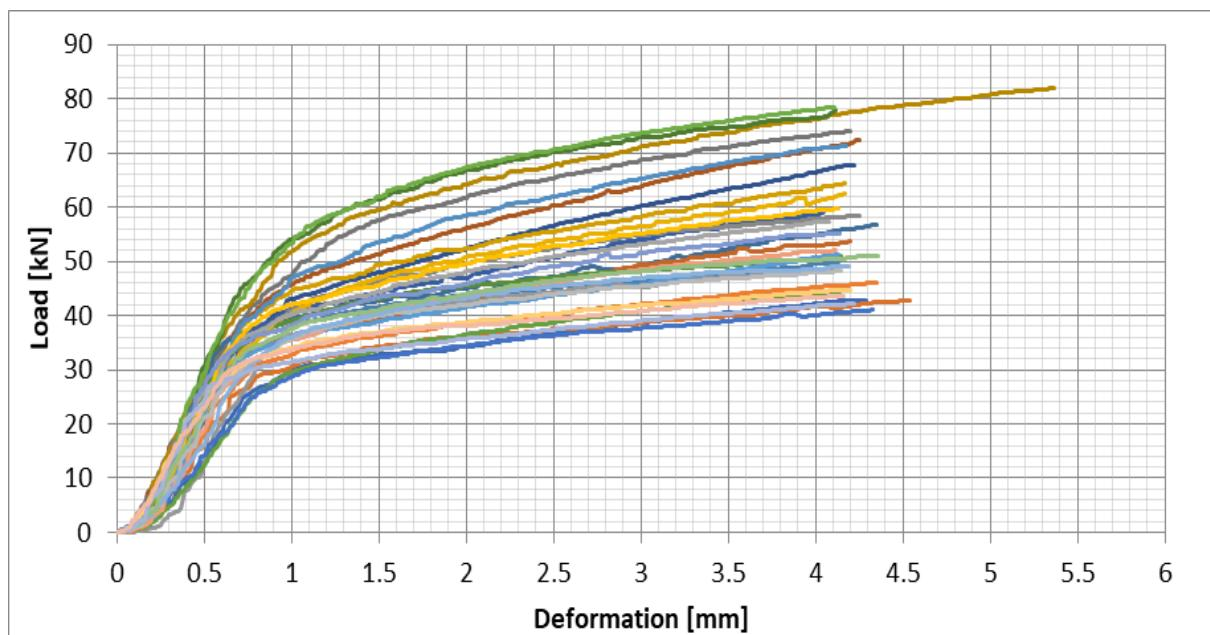
Figure 35: Radiata Pine (S4), All test results – Perpendicular to the grain bearing - Load/Deformation
