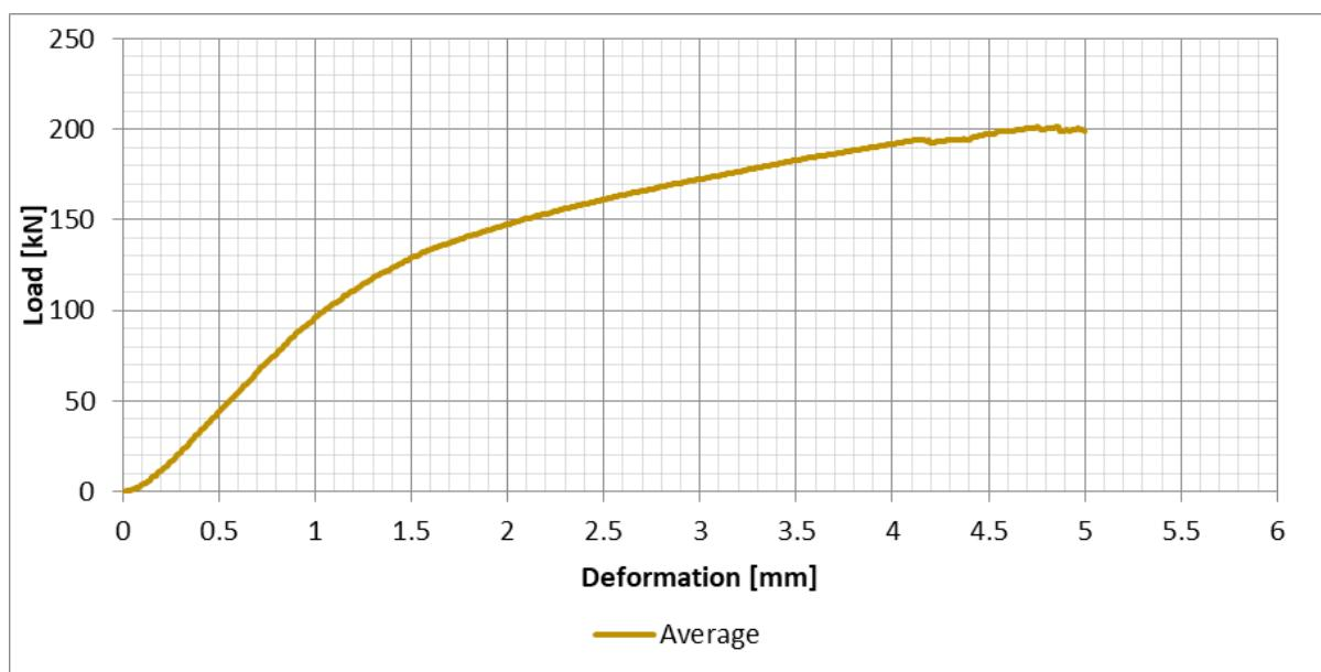
Figure 64: Spotted Gum (H8), Average of all test results – Perpendicular to the grain bearing - Load/Deformation
