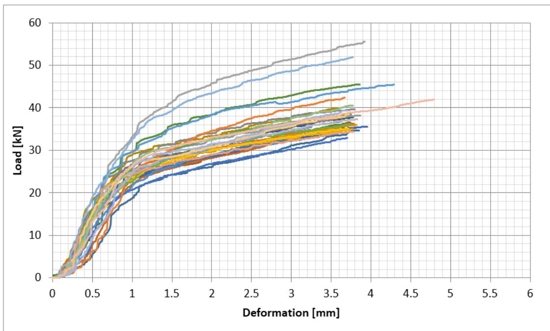
Figure 17: Spruce (I1), All test results – Perpendicular to the grain bearing - Load/Deformation
