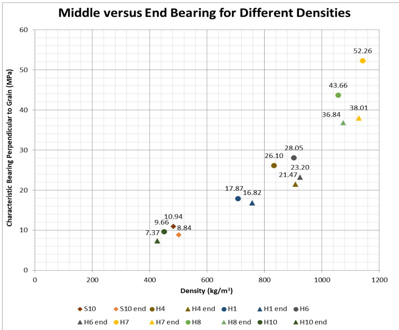
Figure 90: Comparison between the bearing location: the middle and at the end for different wood species
