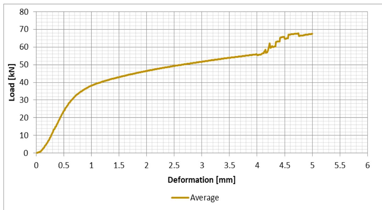
Figure 32: Radiata Pine (S2), Average of all test results – Perpendicular to the grain bearing - Load/Deformation
