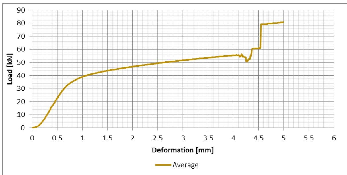
Figure 36: Radiata Pine (S4), Average of all test results – Perpendicular to the grain bearing - Load/Deformation
