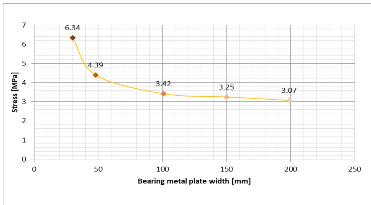
**Figure 86: Characteristic Bearing Perpendicular to the Grain Compared with the Size of the Bearing Area**
