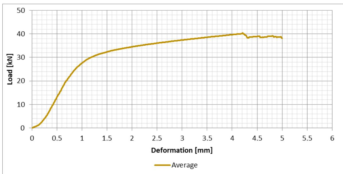
Figure 82: Radiata Pine – End of Plate (S10), Average of all test results – Perpendicular to the grain bearing - Load/Deformation
