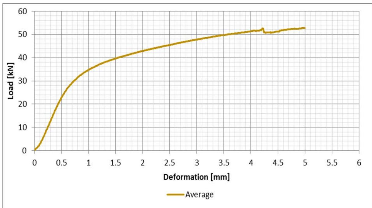
Figure 26: Douglas Fir (old) (I5), Average of all test results – Perpendicular to the grain bearing - Load/Deformation
