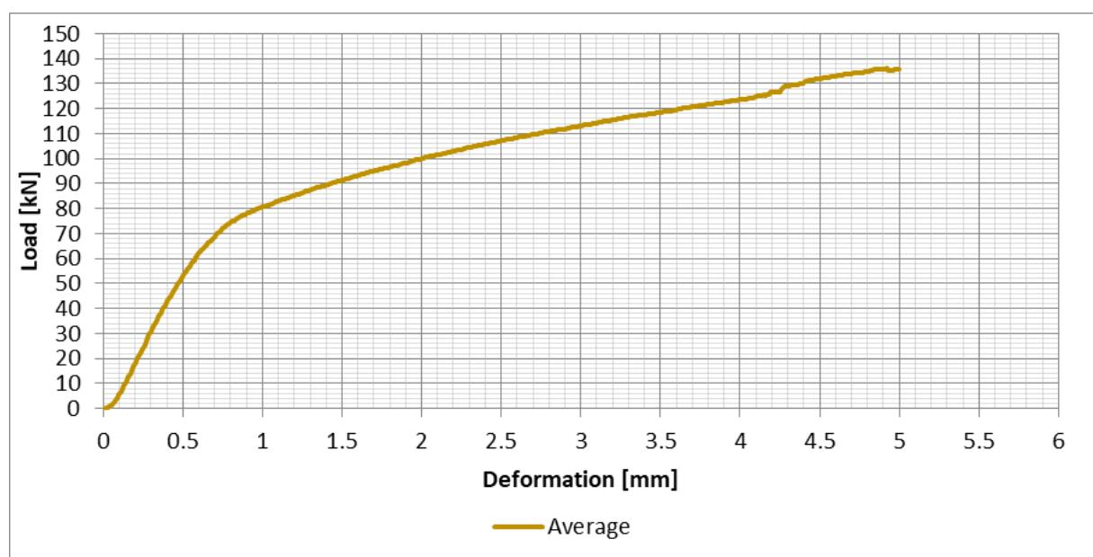
Figure 56: Jarrah (H4), Average of all test results – Perpendicular to the grain bearing - Load/Deformation
