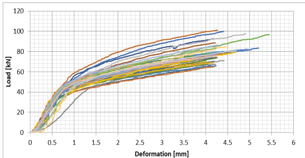
Figure 41: Radiata Pine (S7), All test results – Perpendicular to the grain bearing - Load/Deformation
