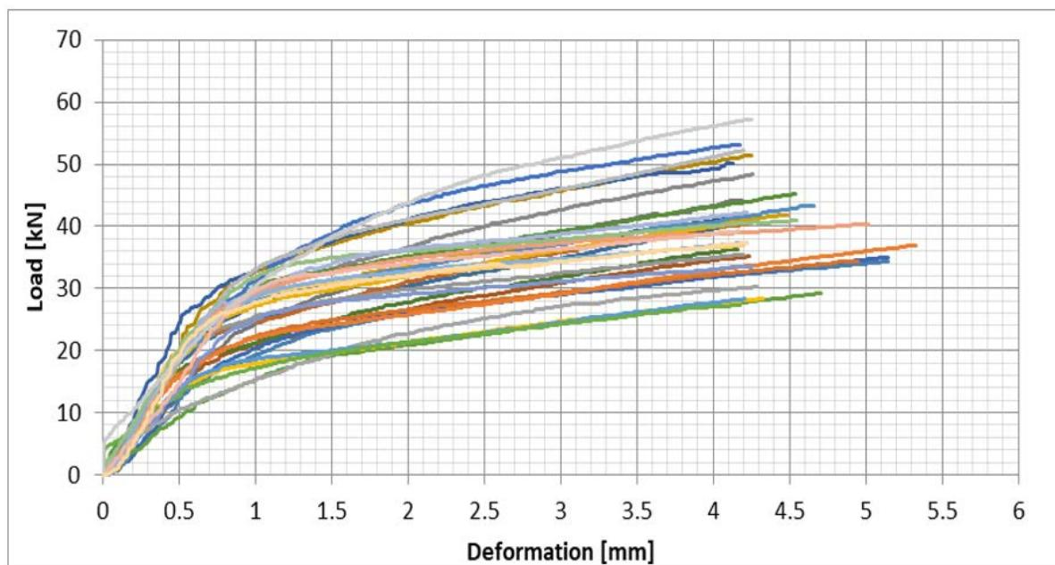
Figure 23: Douglas fir (New) (I4), All test results – Perpendicular to the grain bearing - Load/Deformation
