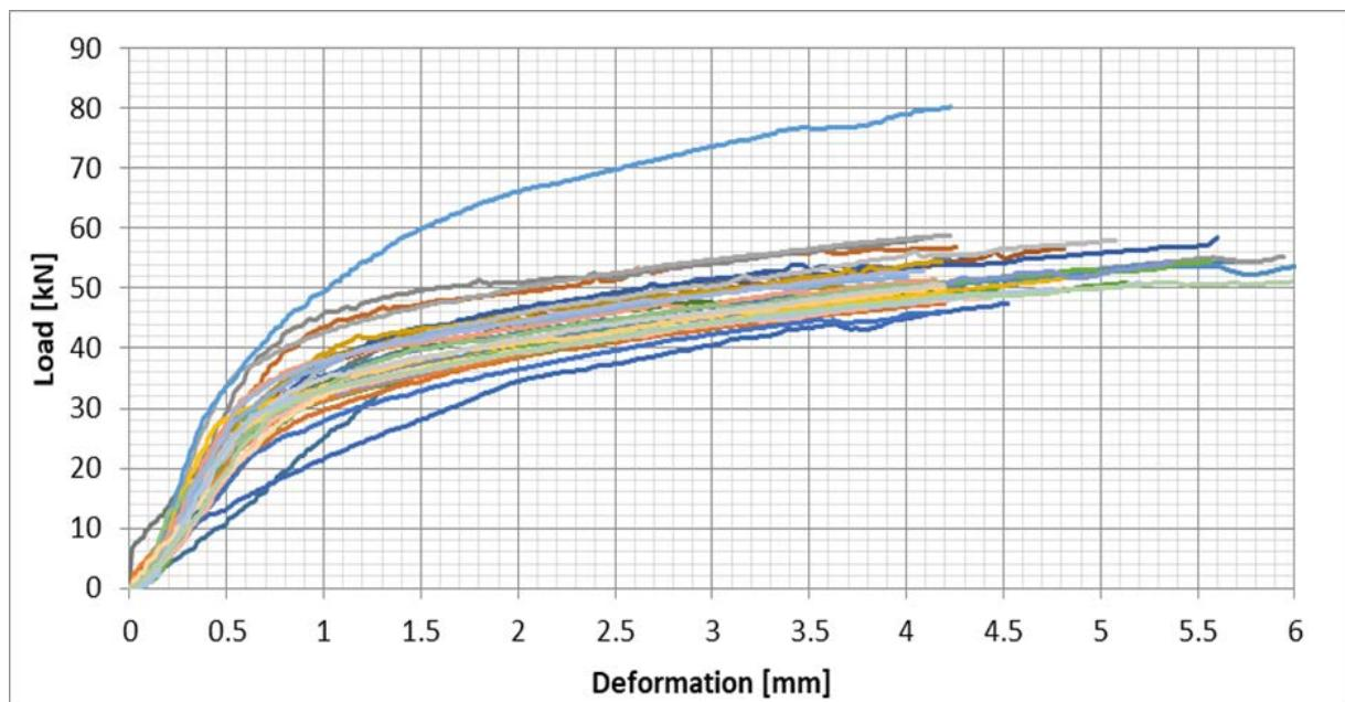
Figure 25: Douglas fir (old) (I5), All test results – Perpendicular to the grain bearing - Load/Deformation
