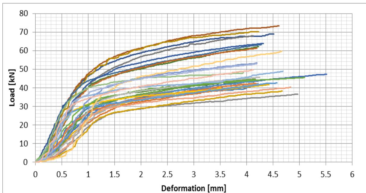
Figure 33: Radiata Pine (S3), All test results – Perpendicular to the grain bearing - Load/Deformation
