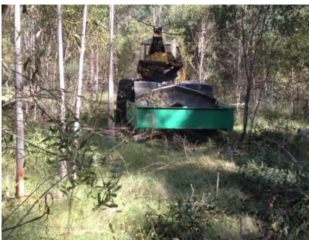
Photo 16-17. Chopper roller working between paint marked trees, note the delineation line between thinned and unthinned
