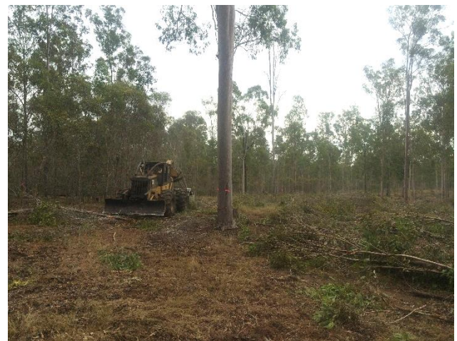
Photo 16-17. Chopper roller working between paint marked trees, note the delineation line between thinned and unthinned
