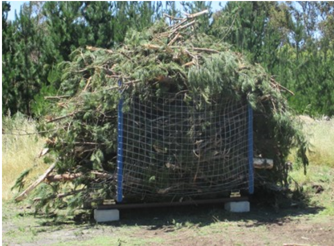
Figure 2. Automated weighing platform with mesh to retain loose radiata pine LR
