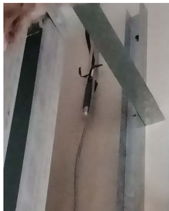
Figure 26: Relative Humidity and Temperature sensor behind a bathroom pod, Image Credit: TDA
