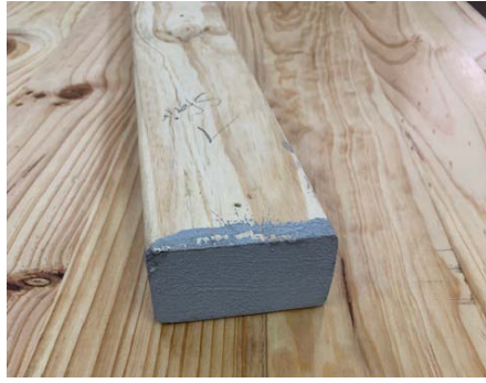
Figure 23: Dummy stud showing moisture-proof compound attached, Image Credit: TDA
