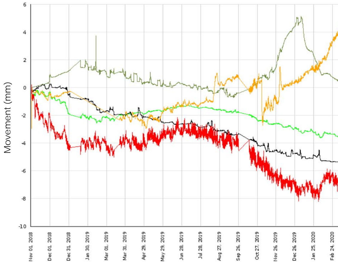
Figure 59: Vertical movement of each level measured in a wall close to the hallway – Position #2
