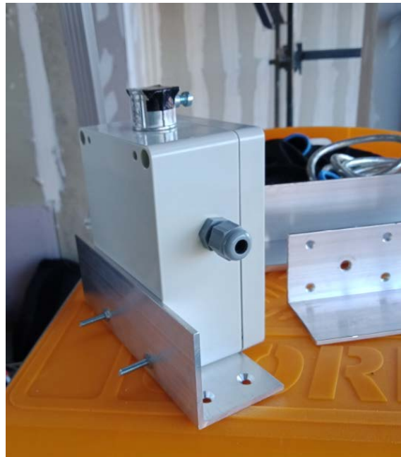
Figure 11: Aluminium Angle used to secure eye bolt and String Pot Box, Image Credit: TDA
