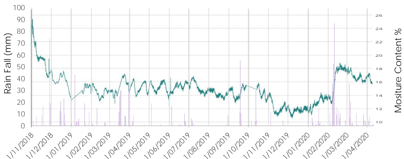
Figure 67: Rainfall data overlaid onto the moisture content of a wall stud in a corridor – Position LV1 #2
