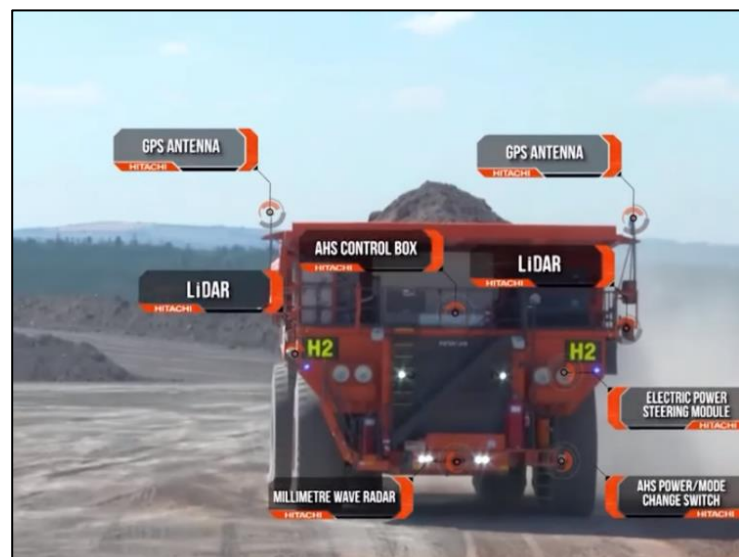
Figure 21: Hitachi autonomous haulage truck operating in an open-cast mine. (Image sourced from www.youtube.com/watch?v=c9_Os6Ha-Gk )
