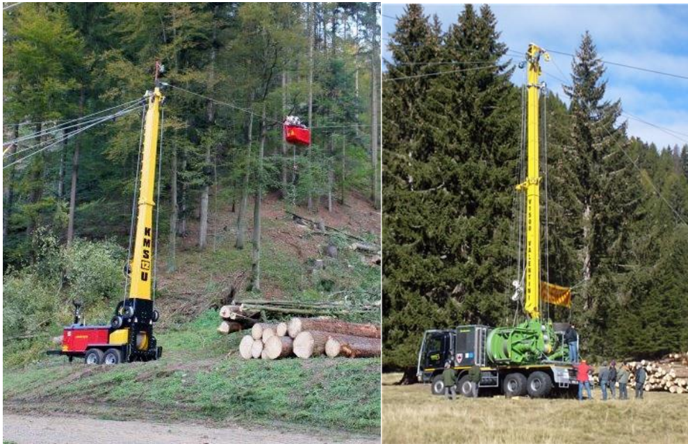
Figure 3: Left: KMS 12U is a radio-controlled cable crane. Right: the Valentini V1500 tower yarder. Both have automated carriage movement and can be remote controlled. (Photos: R. Spinelli).
