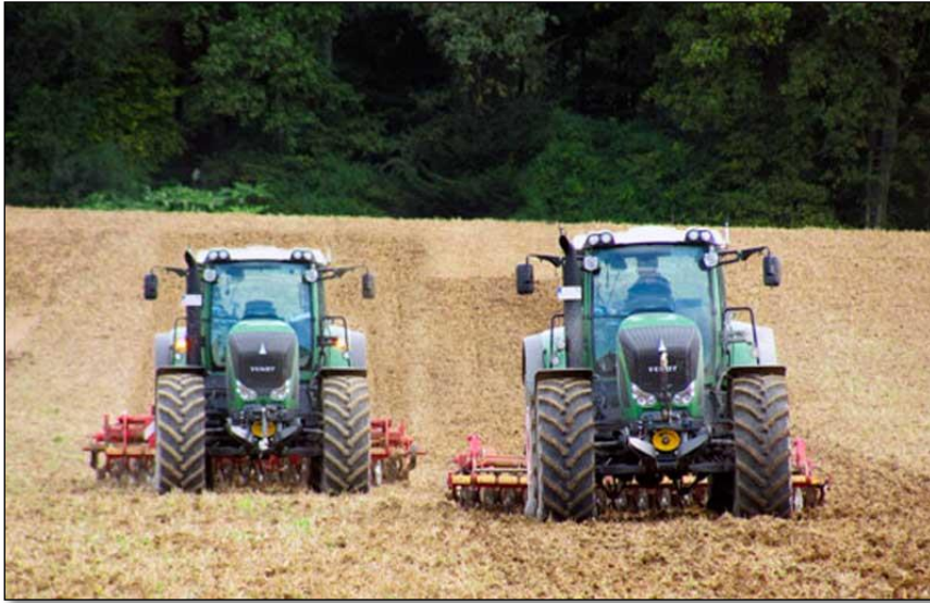
Figure 26: A manned tractor, partnered with an autonomous 'slave' tractor, scarifying the soil. (Image sourced from www.interempresas.net/Agricola/Articulos/61084-Fendt-inunda-FIMA-de-innovaciones-tecnicas-a-bordo-de-su-nueva-serie-700-SCR.html ).
