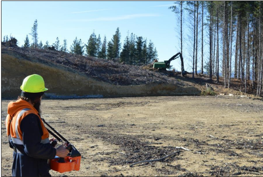
Figure 13: Remotely controlled felling machine developed within the scope of FGR, with the operator in line of sight. (Photo: FGR / ATL)
