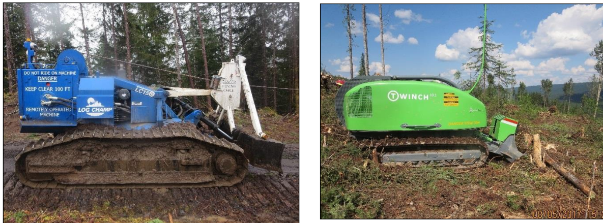
Figure 17: Both the T-Mar LogChamp150 and T-Winch winch-assist machines are constructed without a cab and can only be operated remotely. (Photos: J. Hunt)
