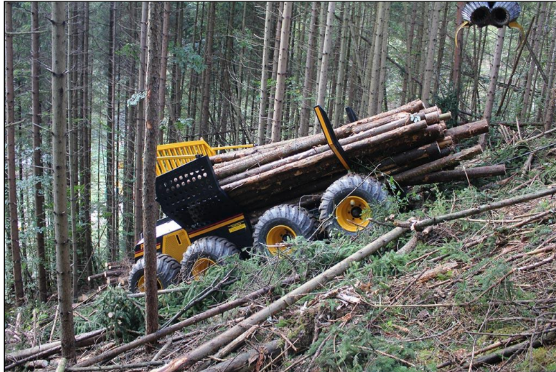
Figure 8: Konrad 'Pully' system that takes logs from the steep terrain harvester down to the roadside guided by a wire rope (photo R. Visser).
