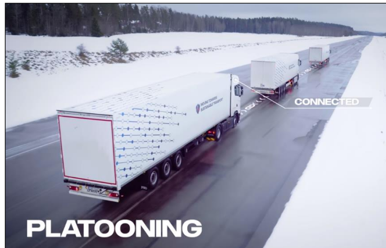
Figure 22: Concept of platooning with sensors simply keeping the following (slave) trucks at a specific distance. (Image sourced from www.scania.com/group/en/gearing-up-for-platooning )
