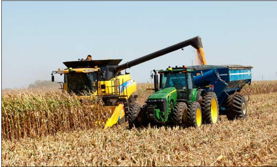
Figure 5: Autonomous carts (tractor-pulled trailers) – they move between a geo-spatially fixed unloading area and GPS tracker on the harvester.
