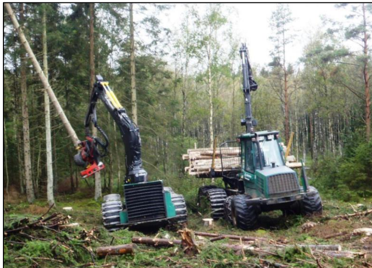
Figure 24: The 'Besten' harvester, shown on the right being operated by the harvester operator, was the first remote controlled tree felling system (photo: R. Visser).
