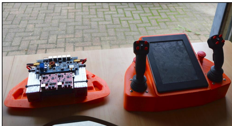
Figure 12: Purpose built remote control design that includes live video feed (Photo: P. Millikan)
