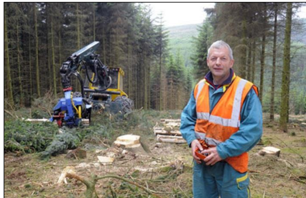
Figure 11: Operator with controls to remotely operate the skidder.
