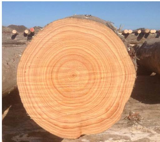
7. Log length was measured and HM200 acoustic velocity obtained. (This included a measure of the resonance spectrum from the HM200 for each log)
