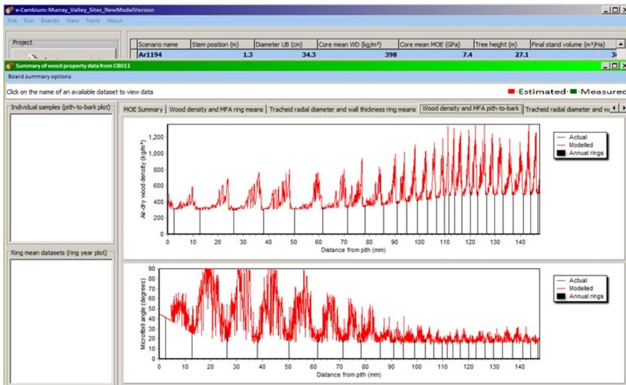
**Figure 60. Graphical output of predicted pith-to-bark variation in wood density and microfibril angle.**
