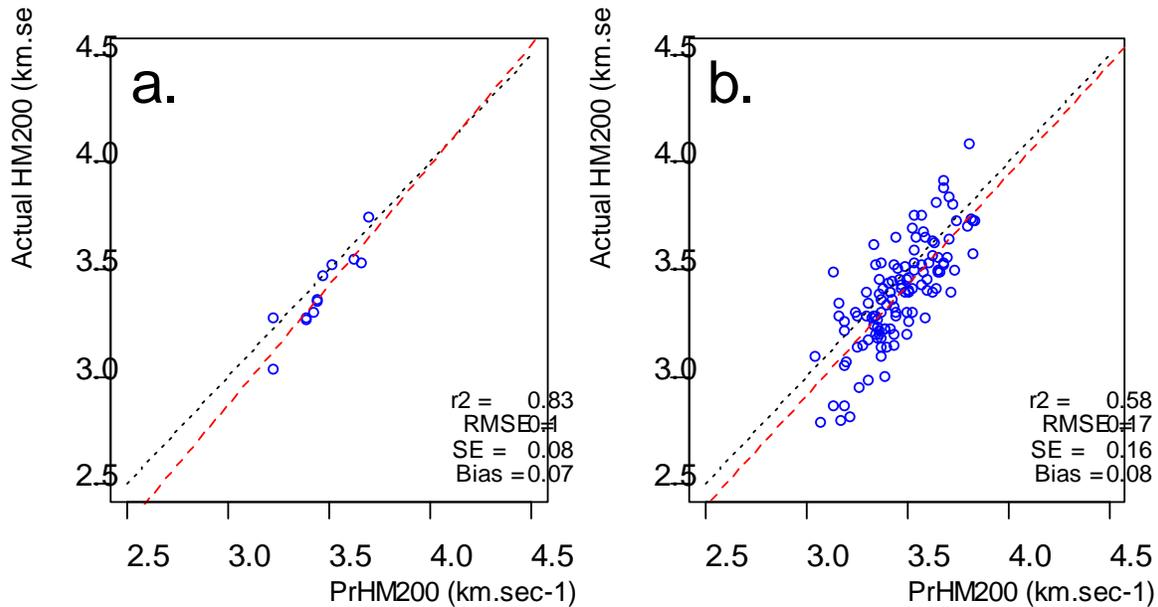
**Figure 28. Predicted versus actual HM200 values. (a) Site-average and (b) individual tree predictions respectively based on a fitted relationship between Actual HM200 values and RESI data from this study**
