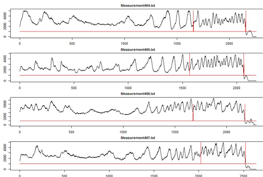
**Figure 24. Four RESI traces, indicating the region over which mean and maximum OWR values were calculated.**
