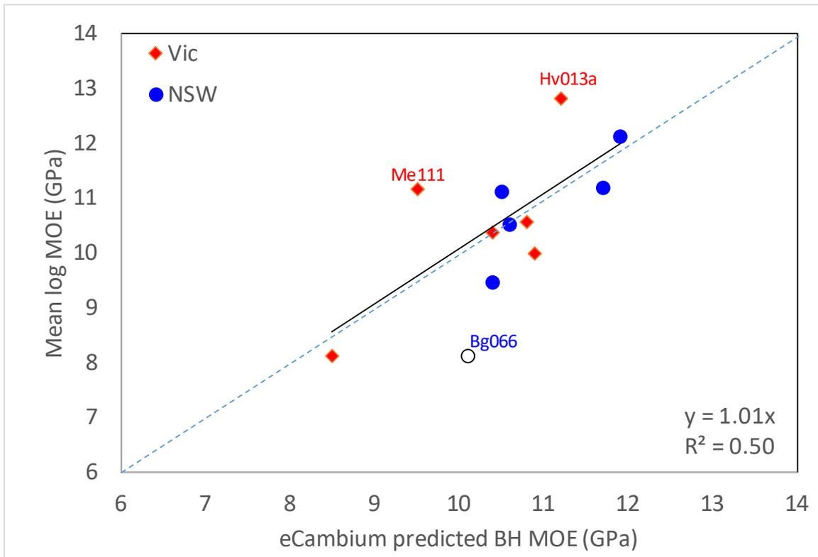
**Figure 35. Predicted vs actual log MOE. Log MOE is the site average calculated from the Hm200 and green log density values, measured on individual logs in the log yard.**
