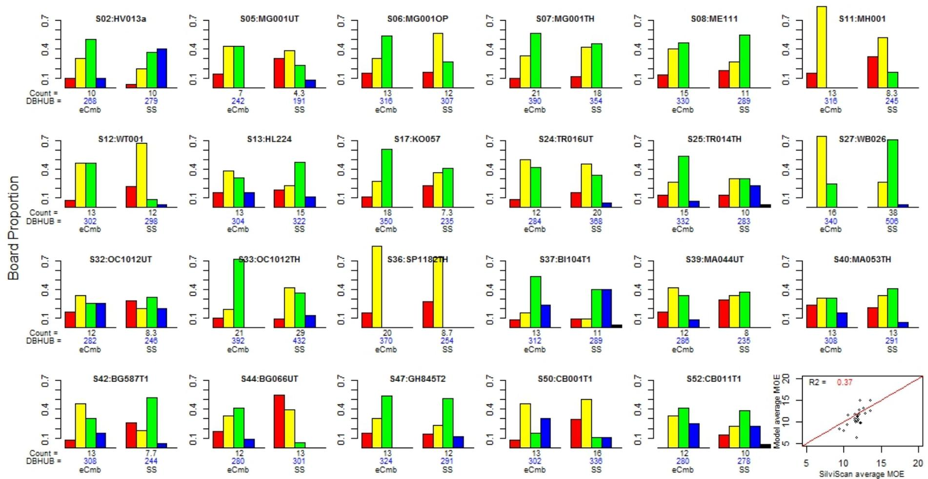
Figure 22. Comparison between SilviScan and eCambium profiles sawn board production. Predicted DBH and board counts are recorded beneath each histogram.
