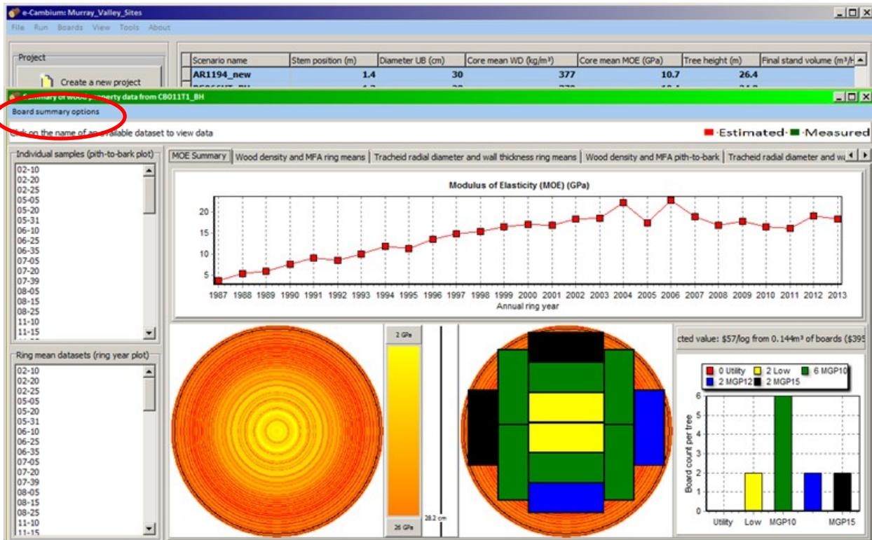
**Figure 57. Graphical output of predicted ring average MOE and hypothetical potential board quality**
