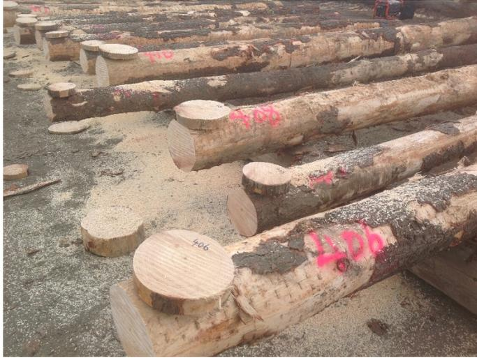
5. The end of each log was cleaned and squared with a fresh chainsaw cut to both ends. The log number was written at the top of the SE end and a 40 mm cross-sectional disc taken. This upper end marking helps to align the disc image with the log barcode during processing, with the DiscBot data. This needed to be as clean and square as possible to minimise preparation time for the DiscBot system at SCION.
