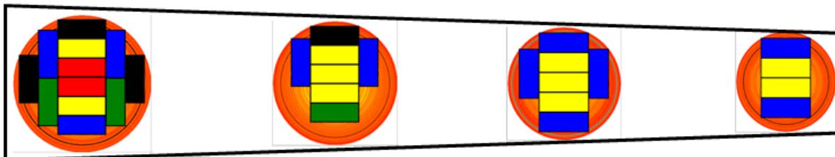
**Figure 12. Representation of a log from breast height (1.3 m) to 7m with predicted boards at 1.3 m, 3m, 5m and 7m.**
