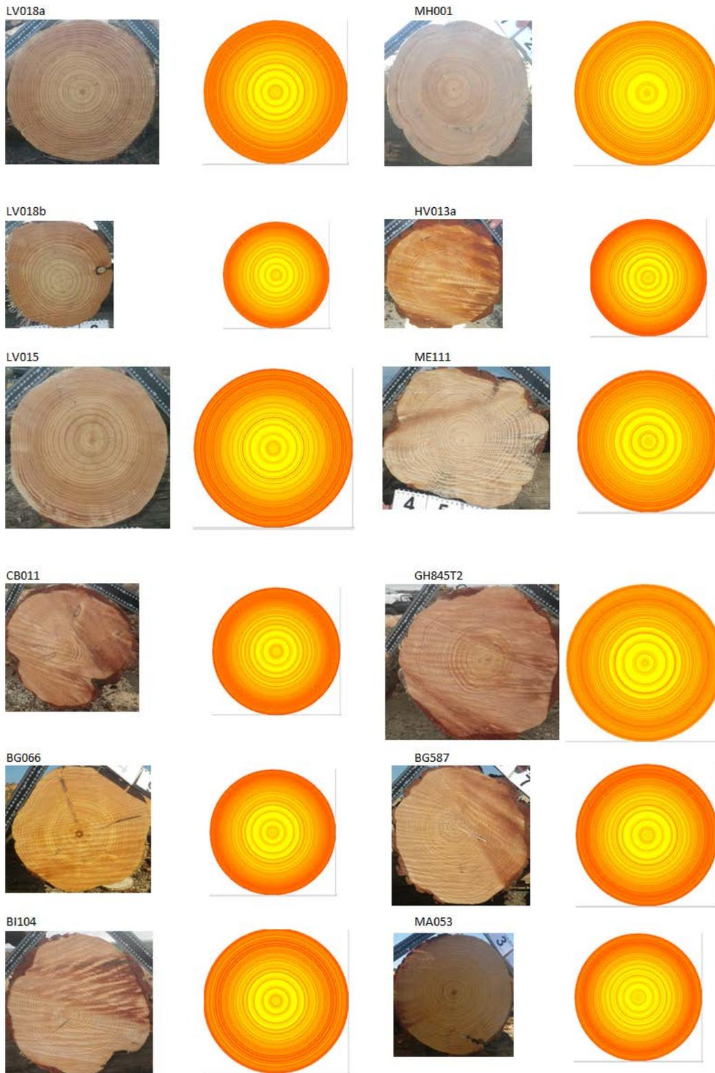
**Figure 39: Images of actual and simulated log ends. The actual ends were chosen to match the simulated tree sizes, and images are scaled relative to each other. Yellow indicates low MOE and red indicates high MOE in the simulated images.**
