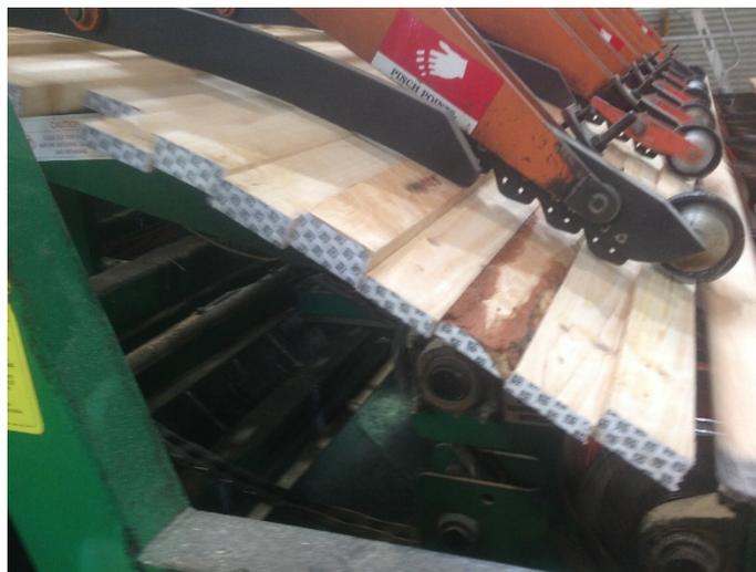
22. There were a couple of log breakages, which resulted in some boards coming through without barcodes, and therefore unable to be identified. Barcoded boards were
