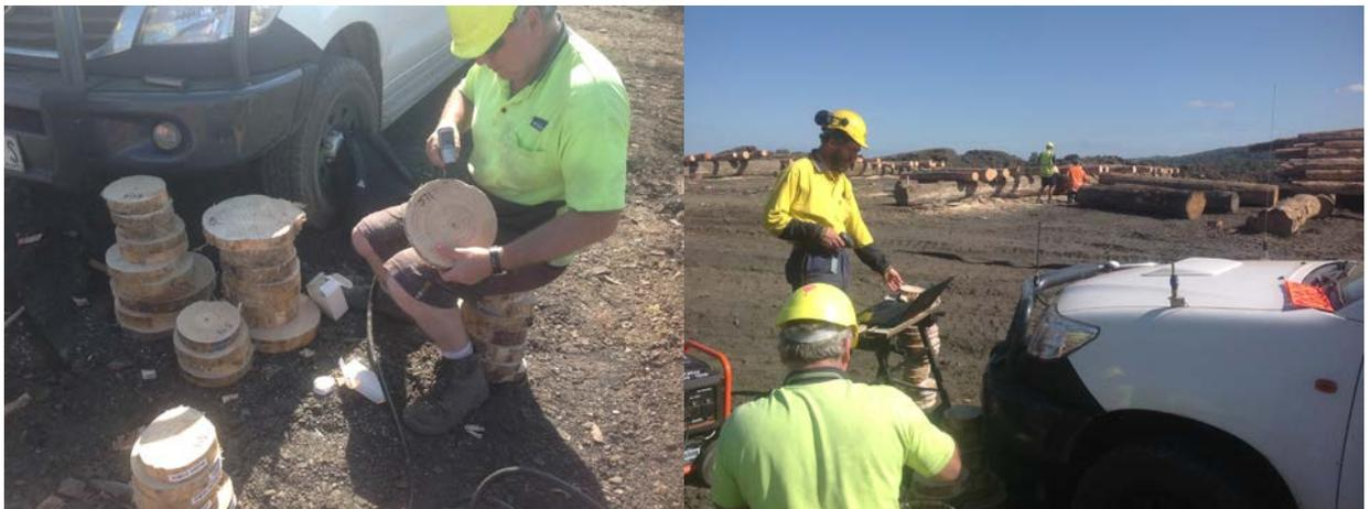
11. Glue was applied to the large end of each log (compressed air driven glue gun, powered by compressor powered by petrol generator), allowing a minute before applying the barcode sheet such that 'North' was towards the top of the log and the centre of the sheet was aligned with the pith. The glue was sourced by Scion who had undertaken various studies to identify the optimal glue to minimize the loss of barcode during the
