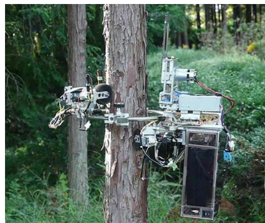
Tree pruning robot prototype. (Image sourced from: www.electronicproducts.com/Electromechanical_Components/Remote-controlled_tree_climbing_chainsaw-welding_robot.aspx )
