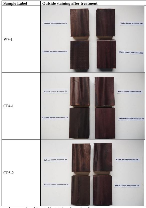
Figure 4. – examples of the outside staining of samples after treatment
