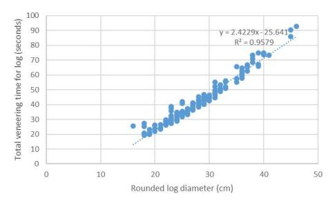
**Figure 5.4**. Total veneering time by rounded log diameter for 3.2 mm thick veneer peeled at 40 lm per minute
