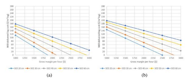
**Figure 5.10.** Sensitivity of maximum mill-delivered log cost to lathe utilisation rate *Notes*: (a) lathe utilisation rate is 60%; and (b) lathe utilisation rate is 80%
