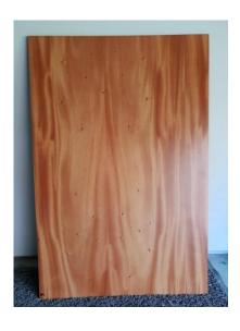
Image 8 b: Veneer panels produced from the Elderslie flitches that were sent to Tasmania
