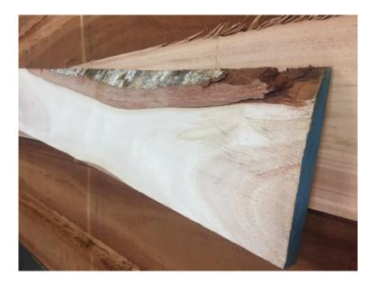
**Figure 6.15.** Example of a wane on a board edge
