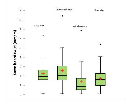
Figure 6.18. Sawn board twist
