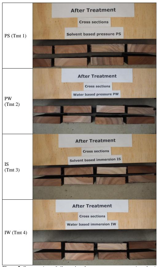
**Figure 5.** Cross sections of all samples after treatment; no penetration of stain observable; samples are positioned in the same order as in Figure 2.
