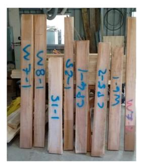
**Figure 1.** - Wood slabs as received and chosen for sample cutting, including their labelling
