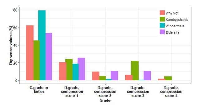
**Figure 6.12.** Dry veneer volume recovery assessed on the basis of veneer compression severity (ignoring all other defects in the veneer sheets)
