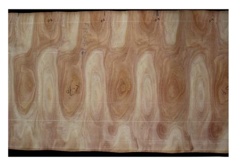
**Figure 6.14.** Veneer containing variable wood resulting from processing logs with non-uniformity (especially taper and sweep)
