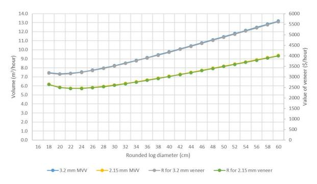
**Figure 5.5.** Veneer volume and value per hour of 2.15 mm and 3.2 mm veneer produced from 2.6 m logs
