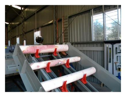
Figure 7.4. Debarked and rounded billets ready for veneer processing
