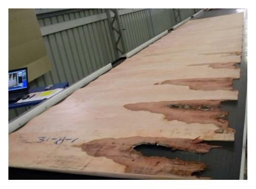
Figure 6.11. Veneer with wane resulting from areas of natural log surface remaining after round-up
