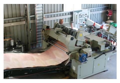
**Figure 7.3**. African mahogany veneer produced from a semi-industrial scale spindleless veneer lathe
