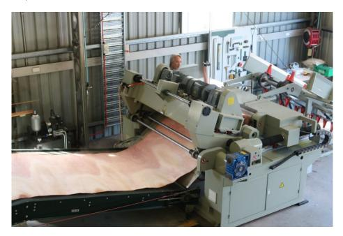
**Figure 6.3**. African mahogany veneer produced from a semi-industrial scale spindleless veneer lathe
