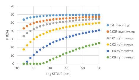
Figure 5.2. Net recovery of marketable veneer from 2.6 m logs by SEDUB and sweep
