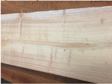
Figure 6.17. Example of pith in a sawn board
