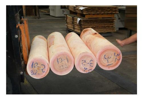
Figure 6.4. Debarked and rounded billets ready for veneer processing
