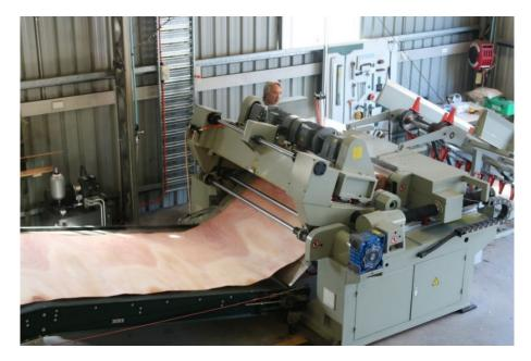
**Figure 7.3**. African mahogany veneer produced from a semi-industrial scale spindleless veneer lathe
