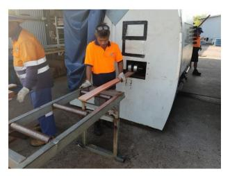
Image 2: Log being milled on the Woodmiser mill at Katherine
