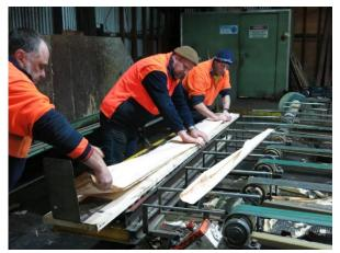
**Image 8 a: Veneer panels produced from the Elderslie flitches**
