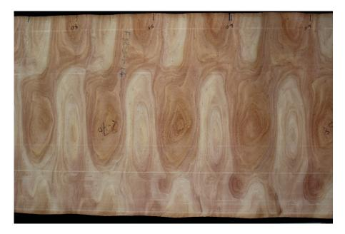
**Figure 6.14.** Veneer containing variable wood resulting from processing logs with nonuniformity (especially taper and sweep)
