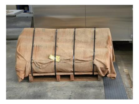
**Figure 7.1.** Logs were end-sealed and wrapped in wet hessian to minimise degrade during transportation
