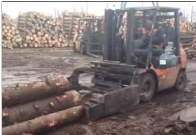
Figure 8. Forklift with a pincer attachment being used to load multiple logs into a container resting on the ground.
