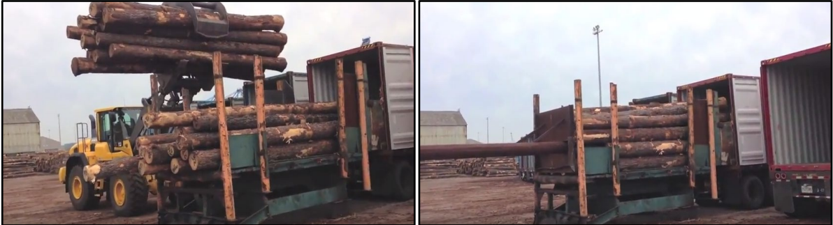
Figure 12. Logs being loaded by a front-end loader into a cradle positioned in front of a container on the back of a waiting truck (left). Logs from the loaded cradle are then pushed into the container by a front-end loader with a pusher plate (right).
