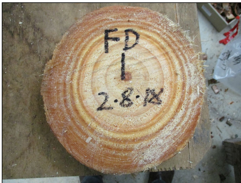
Figure 6. Radiata pine disk, collected on 2 August 2018, and uniquely numbered (F=Forest Cover [referred to as SHADE in this report], D=Debarked, 1=Disk #1).
