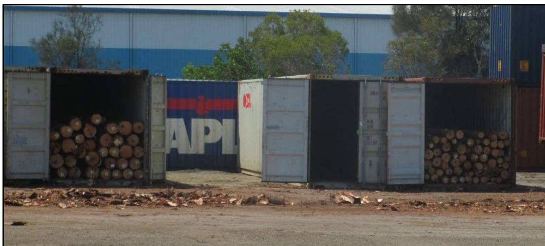
Figure 2. The two containers on the left and right of the photo are “full”, having reached their maximum allowable weight limit. The photo was taken in a log yard in Queensland.
