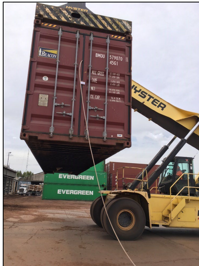
Figure 23. Full containers are moved to a fumigation area by a container handler.
