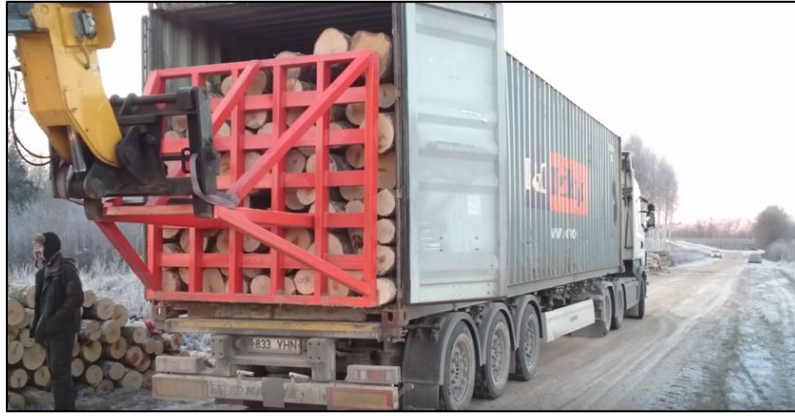
Figure 4. A pusher plate on the end of a boom loader being used to push protruding logs into a container.
