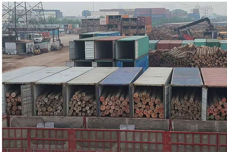
Figure 9. Huangdao Container Terminal in China showing containers that are ¾ “full” due to 25 metric ton weight restrictions. (Source: tptforests.com)
