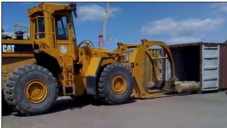
Figure 3. A rubber tyred front-end loader pushes protruding logs the rest of the way into the container using its loading forks.
