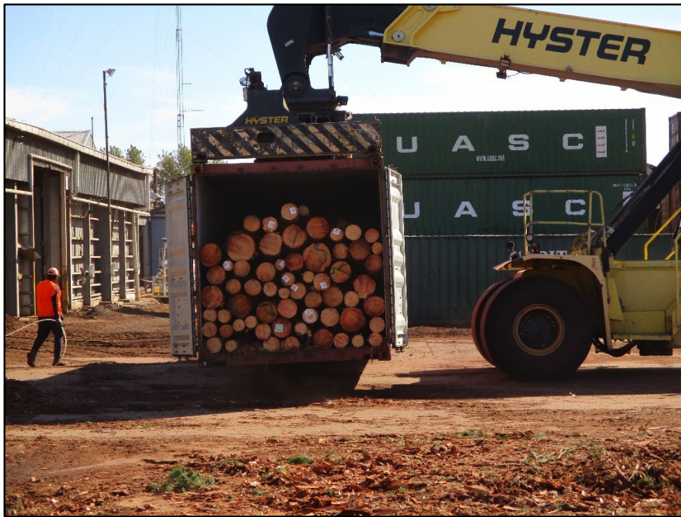
Figure 24. Containers reach their weight limit before space in the container is fully occupied.
