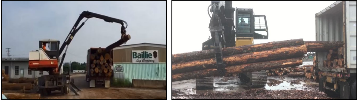
Figure 1. Loading of single logs with a truck-mounted boom loader (left) and multiple logs with an excavator loader (right) into containers on the back of waiting trucks.
