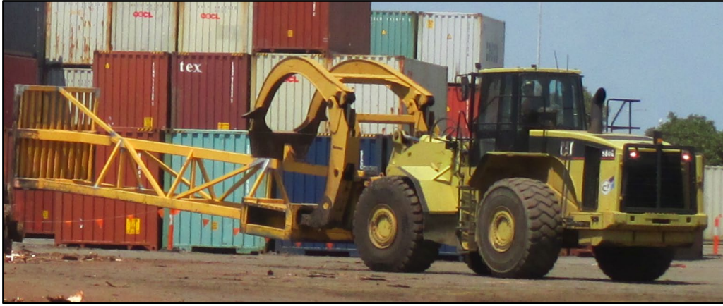
Figure 16. A front-end rubber loader with a detachable pusher plate that are used to push logs into a container resting on the ground.
