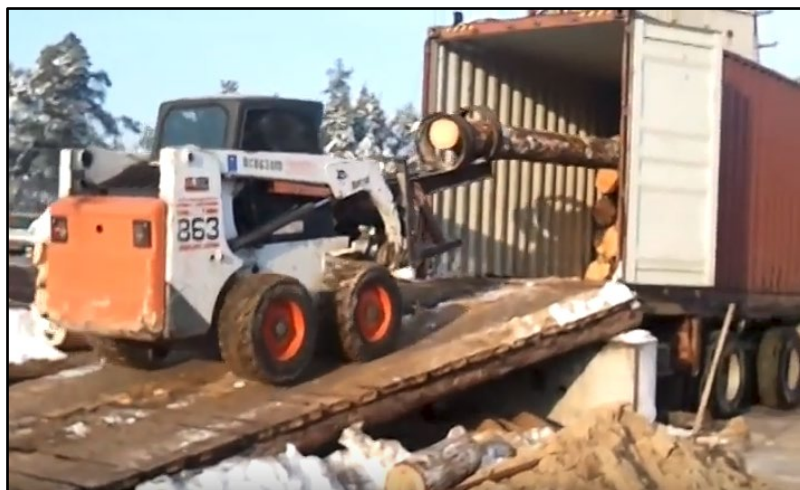
Figure 9. Forklift with a ring attachment being used to load logs into a container on the back of a waiting truck.
