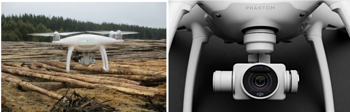
Figure 11. UAV (Phantom 4) and camera used to collect the photographs from Semitrailers
