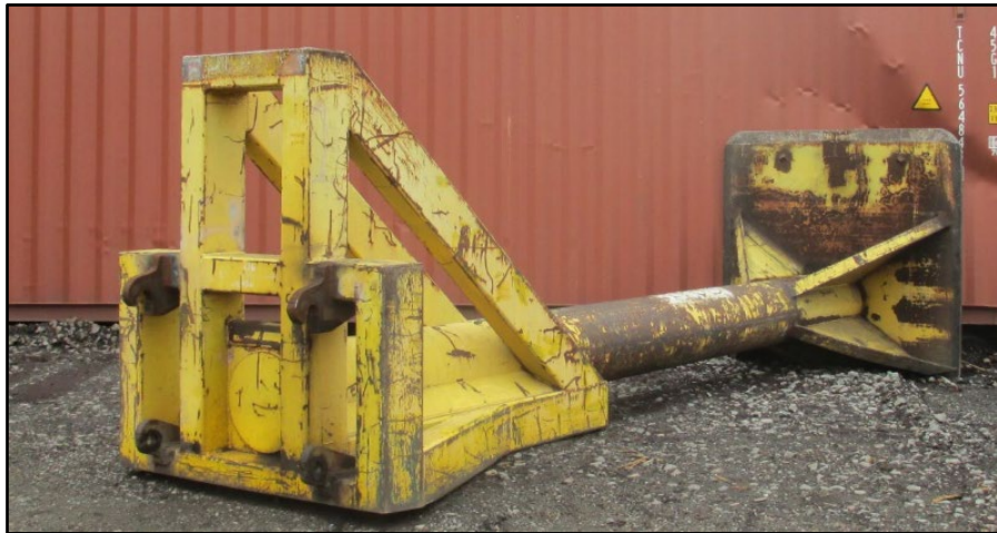
Figure 20. Detachable pusher plate used to push logs from the cradle into containers.
