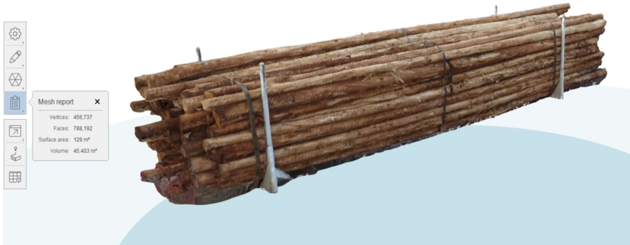
Figure 14. 3D model and mesh report provided by Autodesk Remake™
