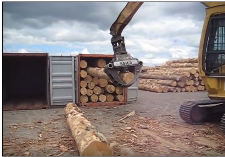
Figure 2. Loading of single logs into a container resting on the ground with an excavator loader.
