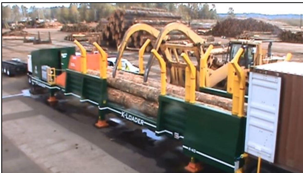
Figure 13. Logs being loaded into a loading frame which contains a pusher plate to transfer the logs into the container on the back of a waiting truck.
