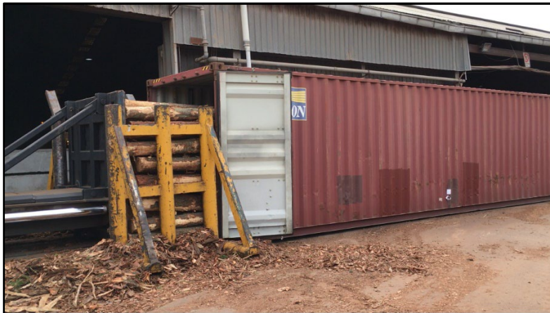
Figure 22. Logs being pushed from the cradle into the container by the hydraulic ram.
