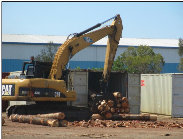
Figure 15. Logs being partially loaded into a container with an excavator loader.
