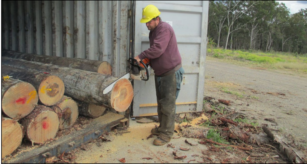
Figure 5. Preparing to collect wood disk from debarked and non-debarked hoop pine logs stored inside a container near Beerburrum, Queensland.
