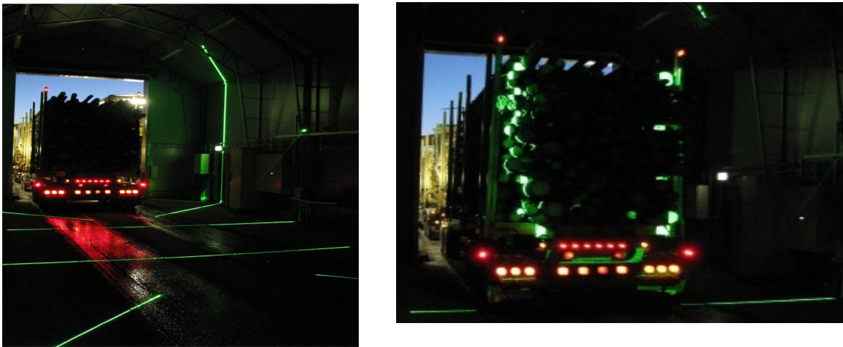
Figure 4. The Mabema GPV® laser scanning system for volumetric measurements (Source: www.mabema.se )
