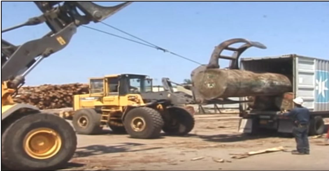
Figure 14. A large log being dragged out of a container by one front-end loader while another front-end loader supports the log.
