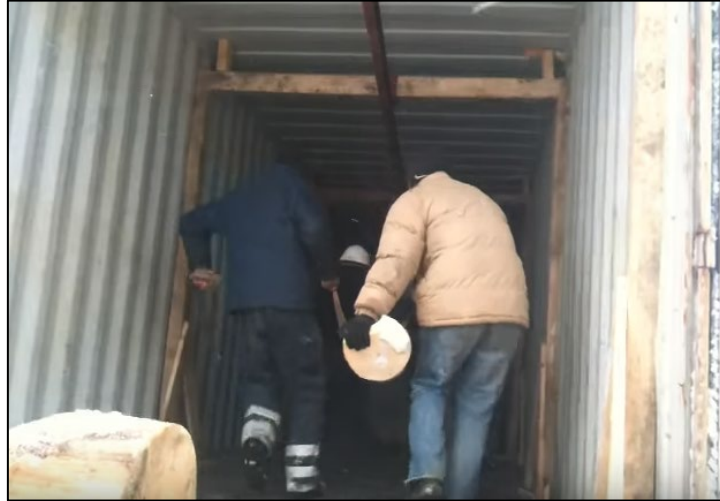
Figure 6. Manual pushing of a single log suspended from a temporarily erected overhead gantry inside a container.
