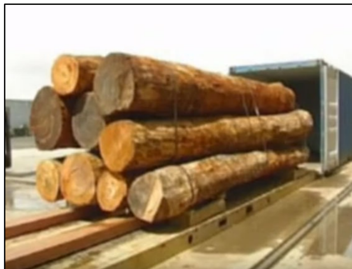
Figure 11. Pre-bundled logs on pallets being loaded with a forklift into a container resting on the ground.
