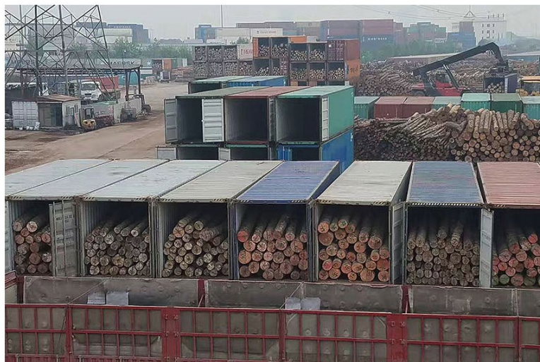
Figure 1. Huangdao Container Terminal in China showing containers that are \frac{3}{4} “full” due to 25 metric ton weight restrictions. (Source: tptforests.com)
