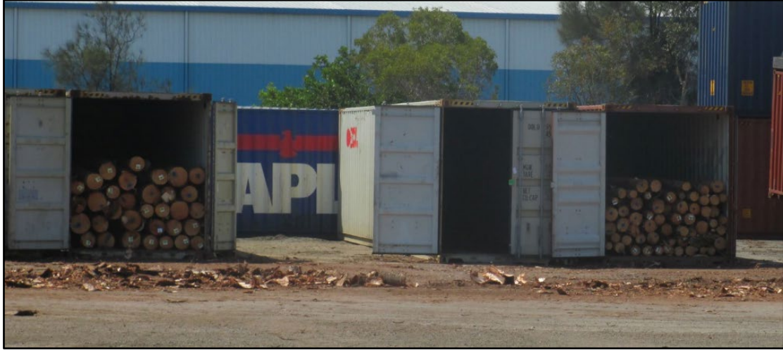
Figure 10. The two containers on the left and right of the photo are “full”, having reached their maximum allowable weight limit.
