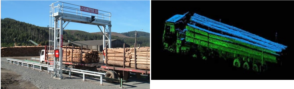
Figure 2. Logmeter laser scanning system developed by Woodtech (Source: www.woodtechms.com )
