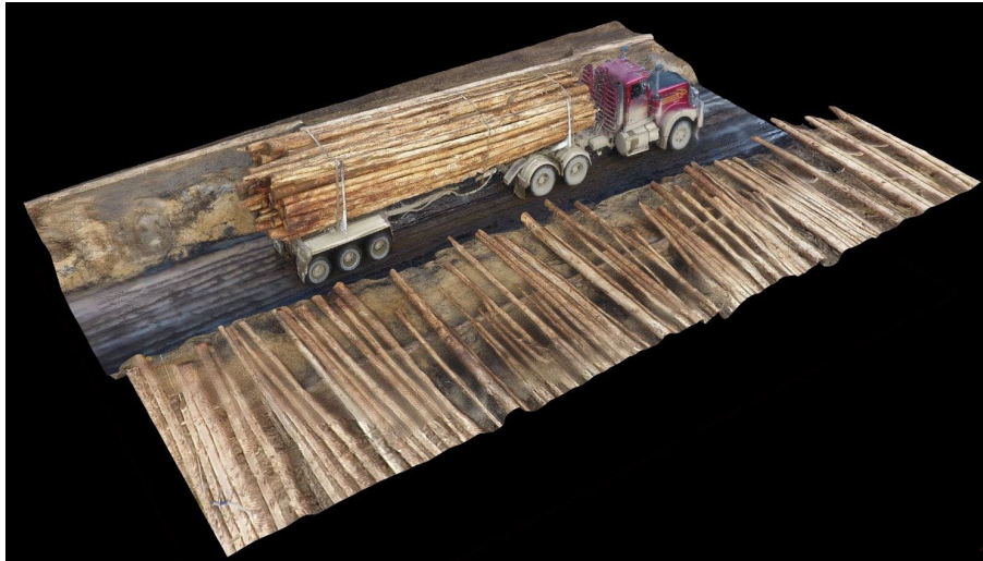
Figure 18. Tile model generated with Agisoft PhotoScan™
