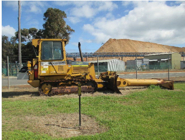
A D4 tractor that is lowered into a ship hold to move and compact woodchips
