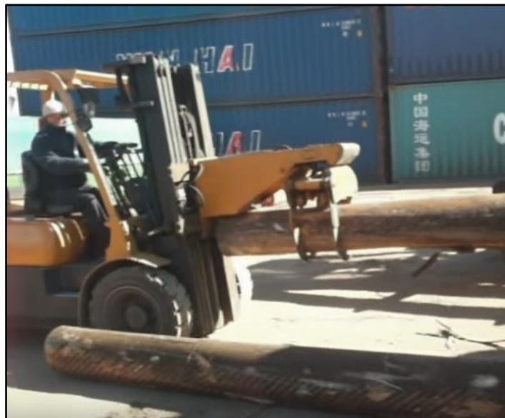
Figure 7. Forklift with a grapple attachment loading single logs into a container resting on the ground.
