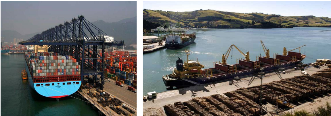
Figure 5. The number of cranes loading or unloading a ship can affect the vessel load rate. On the left is a very large container ship being unloaded simultaneously by eleven on-port cranes. On the right is a bulk cargo ship being loaded by four on-ship cranes. The number of cranes used is generally a function of the ship type and the port infrastructure.
