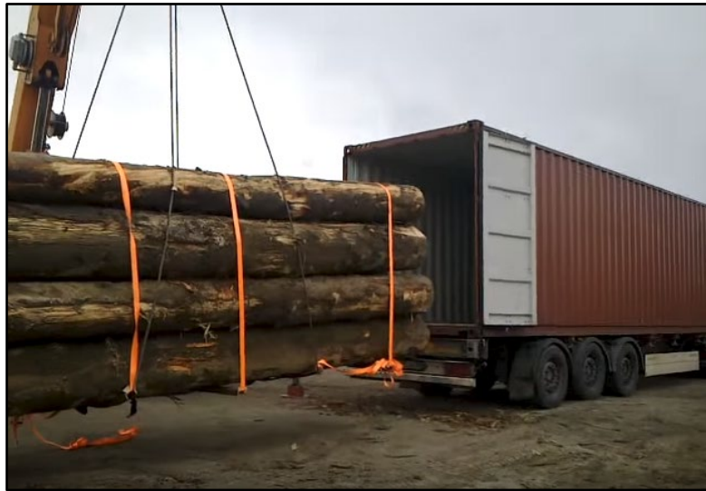
Figure 10. Pre-bundled logs, suspended from a crane, being loaded into a container on the back of a waiting truck.
