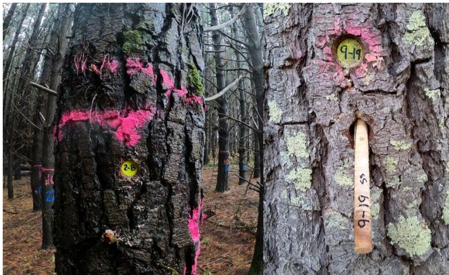
D3 Figure 2. Twenty trees were selected as sawlogs. Plugs were inserted in the core sampling hole to assist in identifying individual butt logs in the log yard, and on three trees per site full radius cores were taken for SilviScan analyses.
