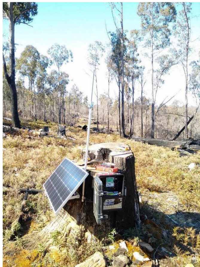
Figure 16: A field deployed stand-alone Gateway (London Lakes) with solar and battery power supply.
