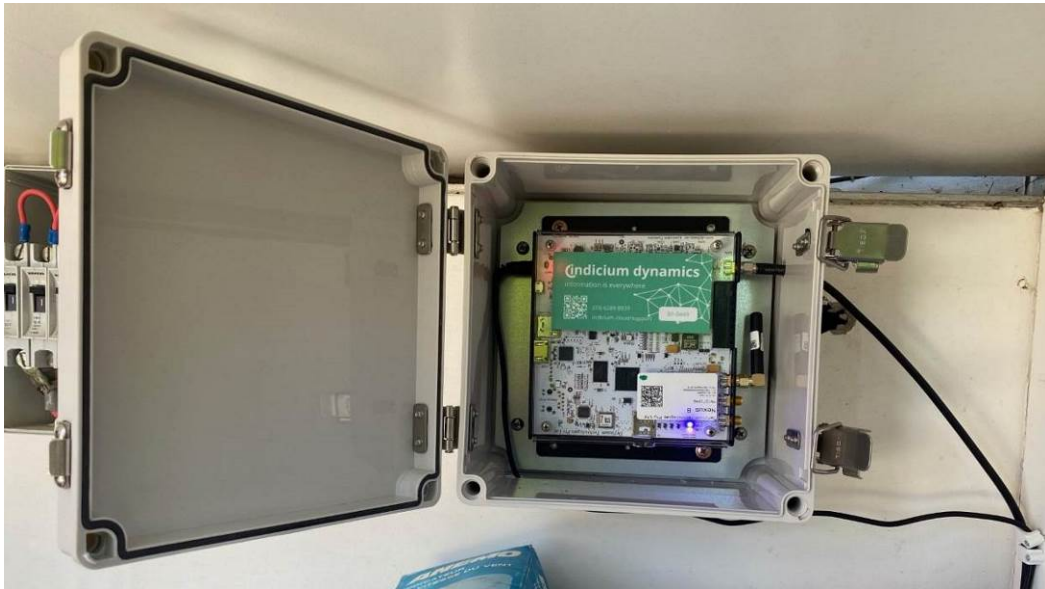
Figure 15: A Gateway installed on a fire tower and powered from 240 volts via a transformer.
