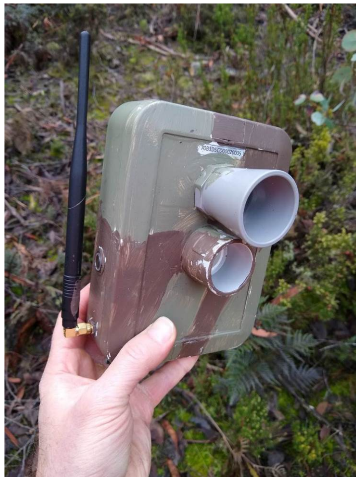
Figure 5: An example of the sensor and node package used in the project. The upper cone on the front of the housing leads to the PIR sensor lens, the lower cone surrounds the transceiver of the US sensor. The units were mounted to the tree so that the sensors aimed at the upper surface of the nest.
