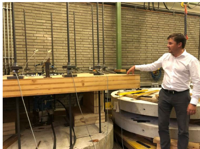
Figure 8: Dr Maderebner explaining the testing of a Spider connection (Image credit: TDA)
