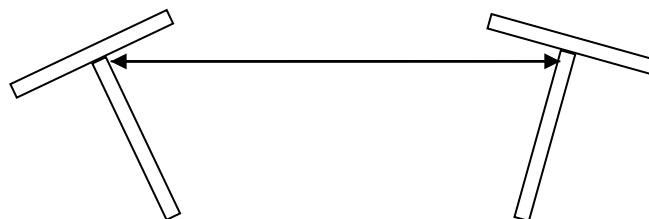
Figure 26: Temporarily prop T-sections a part
