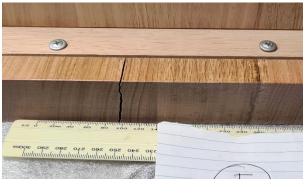
Figure 5: Splitting in a bedside tabletop.
