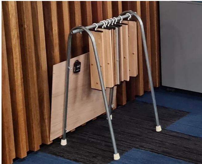
Figure 1: An internal static sensor and sample unit.
