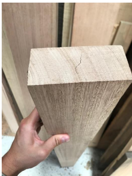
Figure 1: Board with MC-induced end splits
