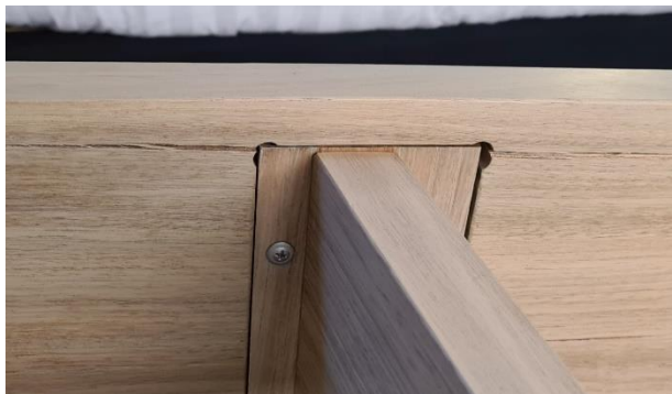
Figure 6: Splitting in a desktop
