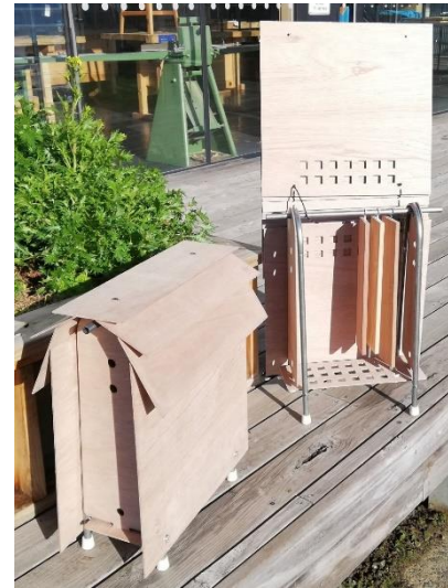
Figure 2: A weather-protected static sensor and sample unit.
