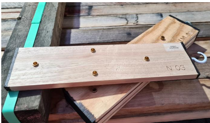
Figure 3: Pins fixed to the labelled sample's face.
