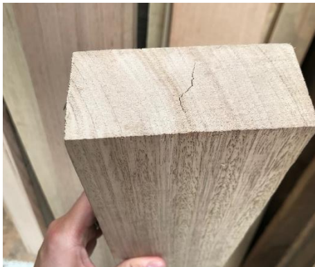
Board with MC-induced end splits
