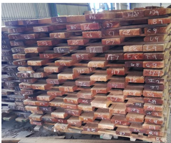
Figure 4: Board numbering in preparation for rack breakdown and data collection
