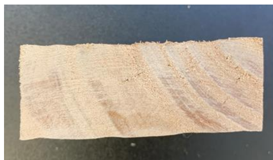
Figure 21. Example of internal collapse in 35 mm thick shining gum boards, several months after SCF impregnation. Photo: Kyra Wood.
