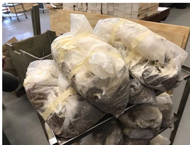
Figure 39. Plastic bags used to inoculate the samples in moist vermiculite for six months. Photo: Jeffrey Morrell.
