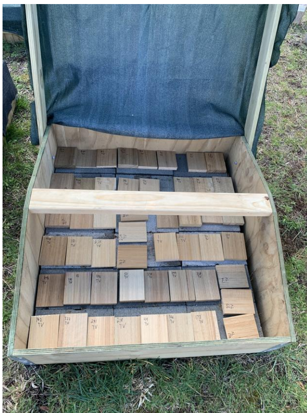
Figure 9. ACQ treated material of varying thicknesses in ground proximity array at Upper Castra, Tasmania. Photo: Kyra Wood.
