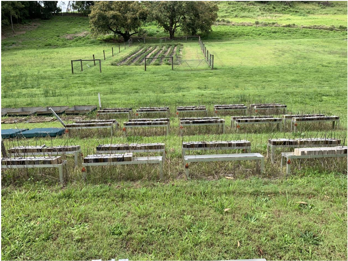
Figure 13. Densified material, and MCA, ACQ, LOSP, and Kop-Coat treated material in sandwich arrays at Nambour, Queensland. Photo: Kyra Wood.
