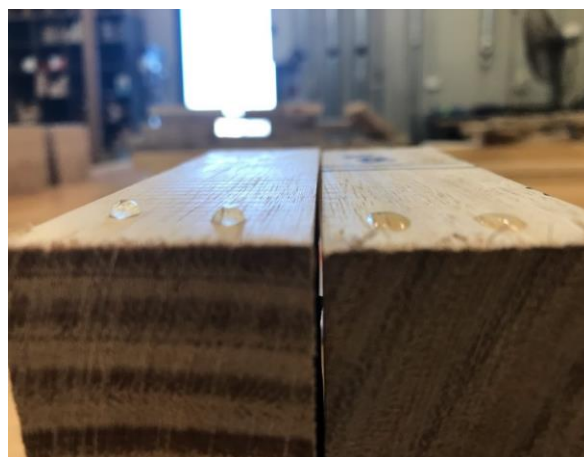
Figure 25. Examples of water droplet behaviour on the surfaces of two E. globulus samples. The sample on the left is untreated, while the one on the right was dipped in water repellent for 3 minutes. Droplets on the untreated sample were rated a 1 while those on the treated sample were rated 3 and 4. Photo: Jeffrey Morrell.
