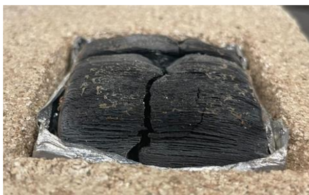
Figure 34. Example of the charring produced with an unrestrained densified shining gum sample. Photo: Wenxuan Wu.
