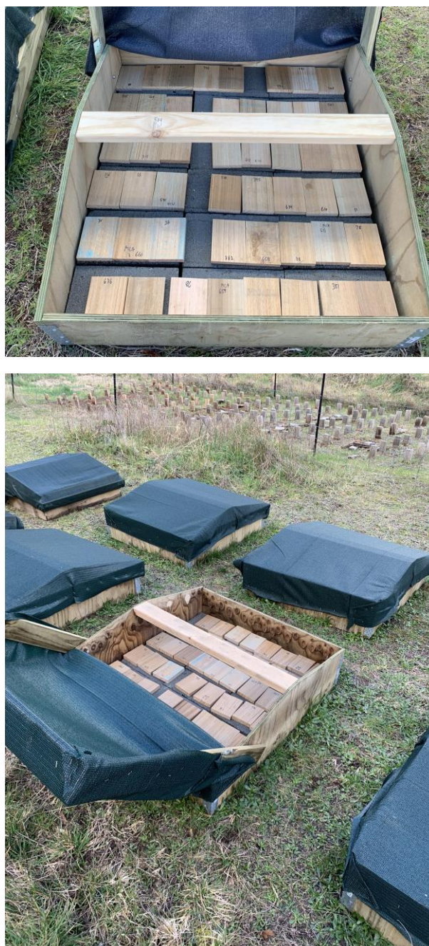
Figure 10. (Top and Bottom) Densified material, and MCA, ACQ, LOSP, and Kop-Coat treated material in ground proximity arrays at Upper Castra, Tasmania. Photo: Kyra Wood.
