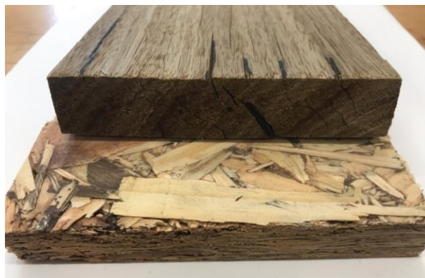
Figure 30. Cross section of a 19 mm thick ACQ treated shining gum sample after 10 wet/dry cycles showing small end splits. Photo: Babar
