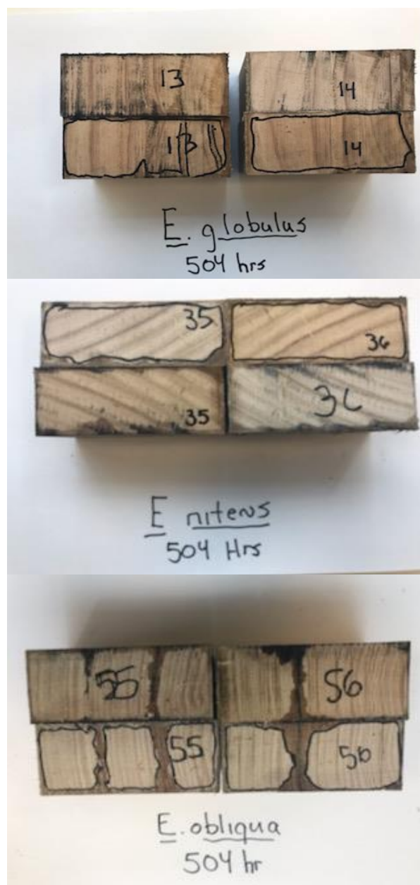
Figure 24. Cross-sections cut from the middle of 90 x 35 mm samples after 504 hours of water immersion. The permanent marker delineates the area of visibly wet wood. Samples correspond to E. globulus (13 untreated/14 treated), E. nitens (35 untreated/36 treated) and E. obliqua (55 untreated/56 treated). Photo: Jeffrey Morrell.
