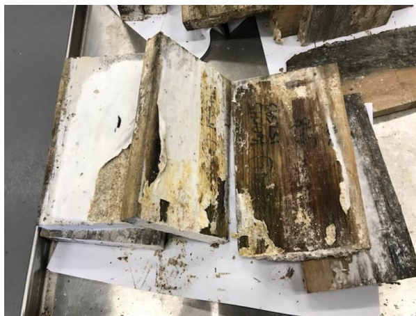
Figure 41. Example of ACQ treated blocks covered with an extensive mycelial mat and showing evidence of darkening and surface cracking at the end of the incubation period. Photo: Jeffrey Morrell.
