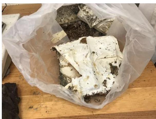
Figure 40. Examples of samples covered in thick mycelial mat in a freshly opened bag. Photo: Jeffrey Morrell.
