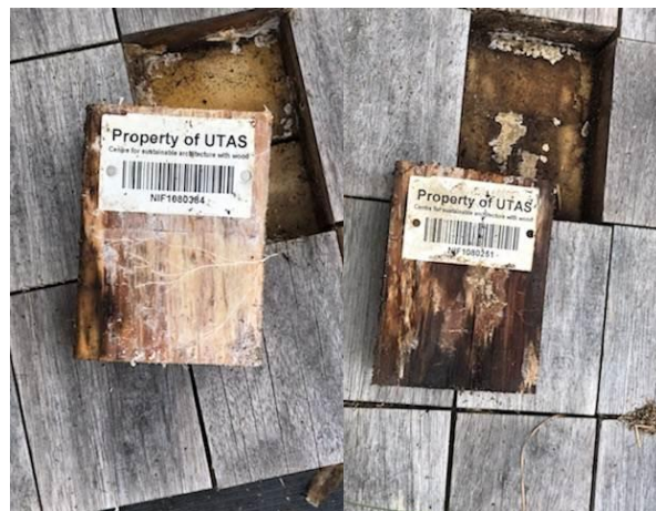
Figure 5. Example of two blocks from the ground proximity array at Nambour, Queensland, with the aggressive fungus showing white rot attack. Photo: Jeffrey Morrell.
