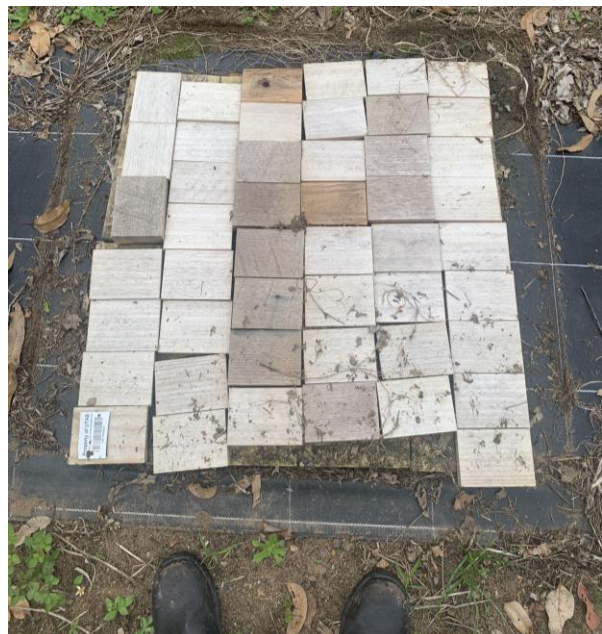
Figure 7. SCF (and some other) treated material in ground proximity array at Nambour, Queensland. Photo: Kyra Wood.
