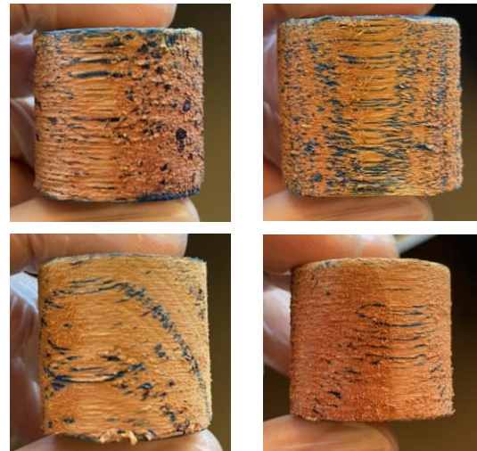
Figure 36. Plugs cut from ACQ treated E. nitens and sprayed with copper indicator showing extremely shallow and inconsistent barrier and core treatment. Photo: Juan Roberto Vargas.
