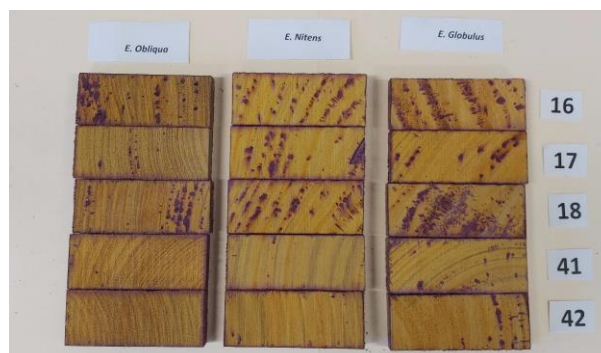
Figure 17. E. obliqua , E. nitens , E. globulus (left to right) Charge 6 board cross sections treated with ACQ showing extremely minimal penetration, even using the more sensitive PAN indicator spray. Photo: Stuart Meldrum.
