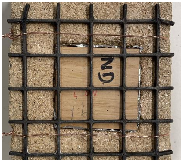
Figure 33. Example of grid used to restrain the compressed samples during cone calorimeter testing. Photo: Wenxuan Wu.
