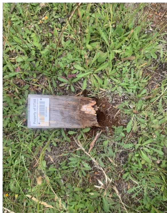
Figure 4. Example of complete failure of a P. radiata stake after one year in the ground at Upper Castra. Photo: Kyra Wood.
