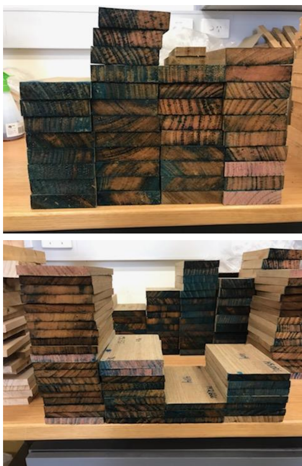
Figure 28. Examples of cross sections of ACQ treated E. nitens and E. obliqua samples of varying thicknesses showing the differences in degree of preservative penetration for 12 mm (bottom) and 25 mm (top) thick samples. Photo: Jeffrey Morrell.
