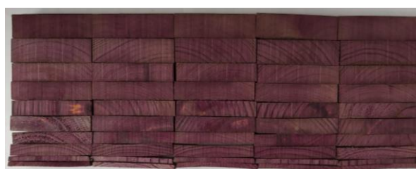
Figure 20. Southern pine cross sections from boards VPI treated with ACQ, and sprayed with PAN indicator spray, charges 1 – 5 from left to right. Thicknesses ranging from 25 mm thick boards (top) to 5 mm thick boards (bottom). Photos: Stuart Meldrum.
