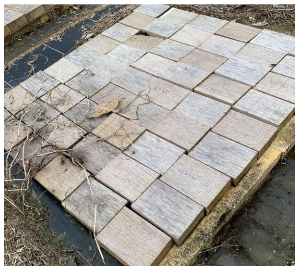
Figure 8. Boron and copper naphthenate treated material in ground proximity array at Nambour, Queensland. Photo: Kyra Wood.
