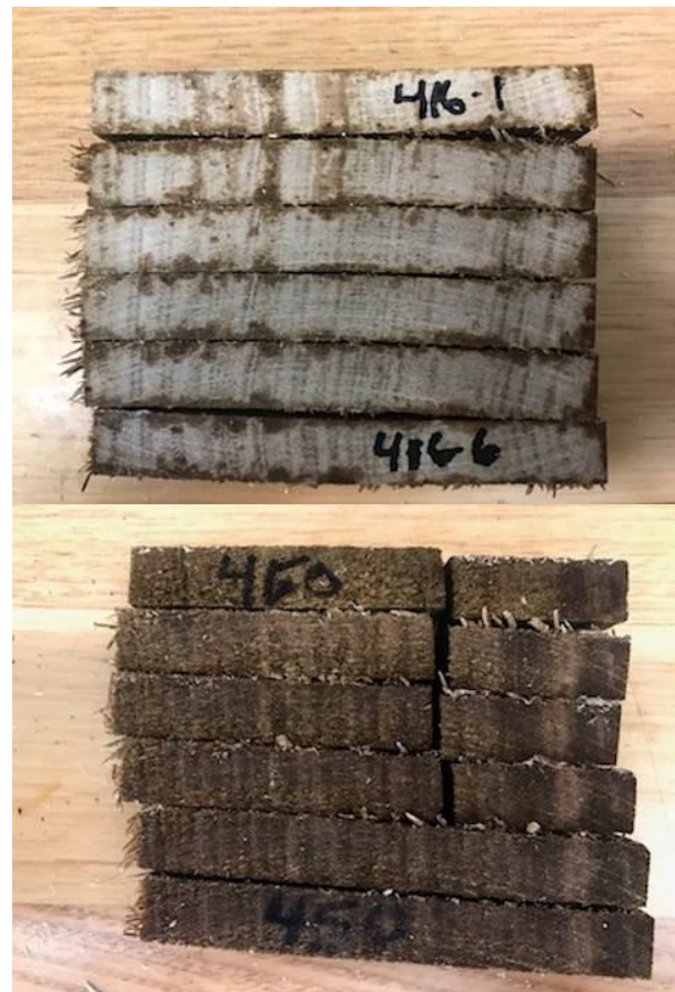
Figure 32. Examples of the sequential 20 mm thick cross cuts from 12 mm thick ACQ treated shining gum samples after the final wetting cycle showing minimal wetting on the upper sample and complete soaking on the lower one. Note the lower, wetted sample also experienced more deformation and cracking. Photo: Jeffrey Morrell.
