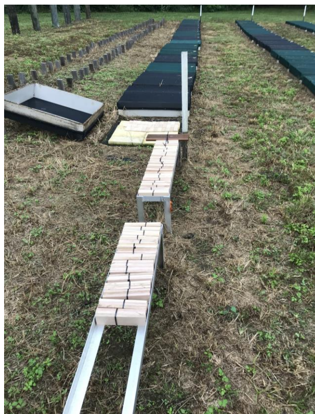
Figure 12. Thermo-mechanically densified material in sandwich arrays at Nambour, Queensland. Photo: Jeffrey Morrell.
