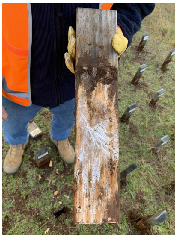
Figure 3. Mycelial growth on an in-ground stake at Upper Castra, Tasmania. Photo: Kyra Wood.
