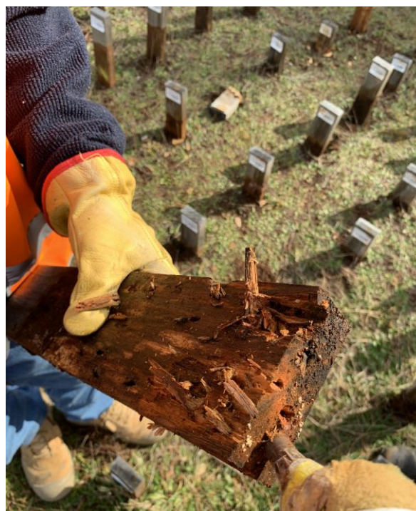
Figure 2. Pick/splinter test showing screwdriver buried in P. radiata stake after one year in the ground at Upper Castra. Photo: Kyra Wood.
