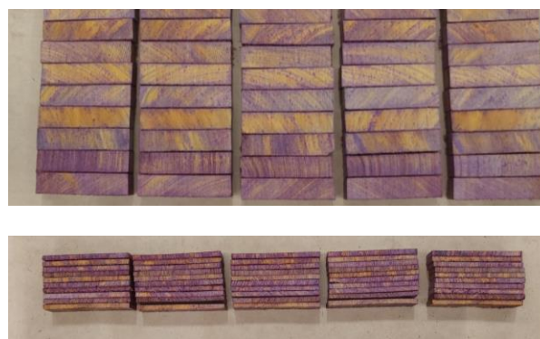
Figure 18. Shining gum cross sections from boards VPI treated with ACQ, and sprayed with PAN indicator spray, charges 1 – 5 from left to right. 25 mm thick boards (top) and 5 mm thick boards (bottom). Photos: Stuart Meldrum.
