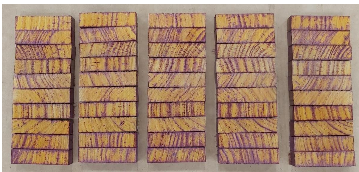
Figure 27. Example of 'candy-stripping' effect in ACQ treated shining gum sprayed with a PAN indicator spray. Photo: Stuart Meldrum.
