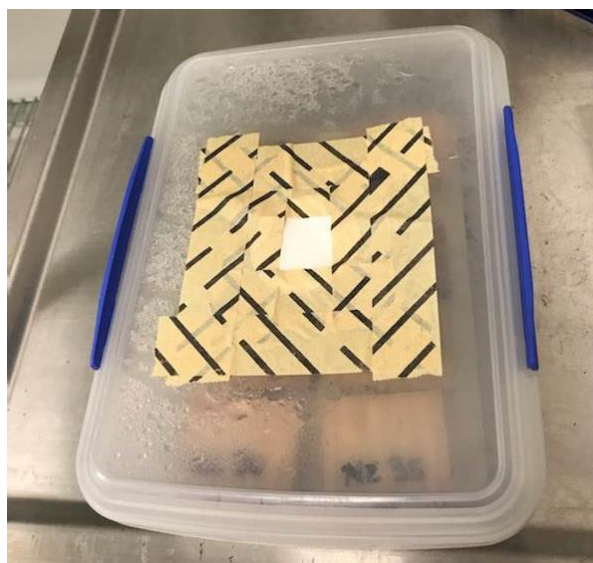
Figure 32. Agar block test using densified material. Photo: Jeffrey Morrell.
