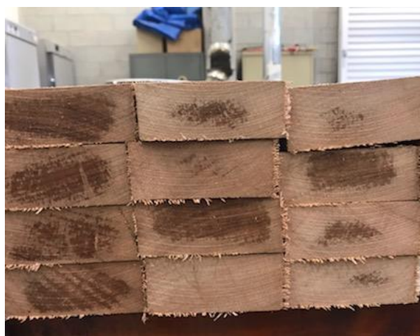
Figure 26. Solid piled boron treated F. brayleyana with substantial moisture still evident in the core of the boards after a twelve week diffusion period. Photo: Jeffrey Morrell.
