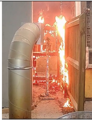
t=34 min fire spread and opening up of west end of north fence with minor burn through by central post
