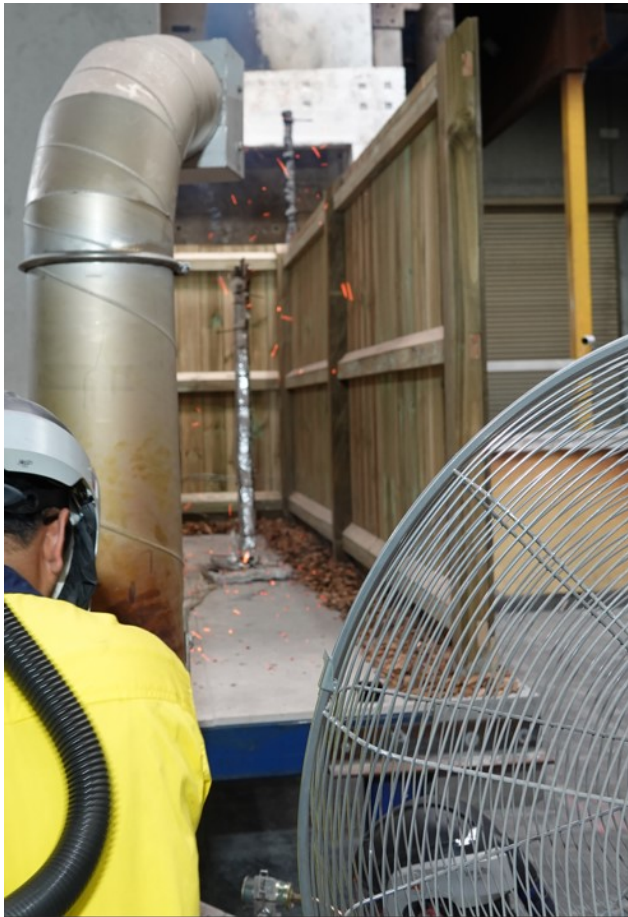
Figure 53 Ember generator and fan during test 1
