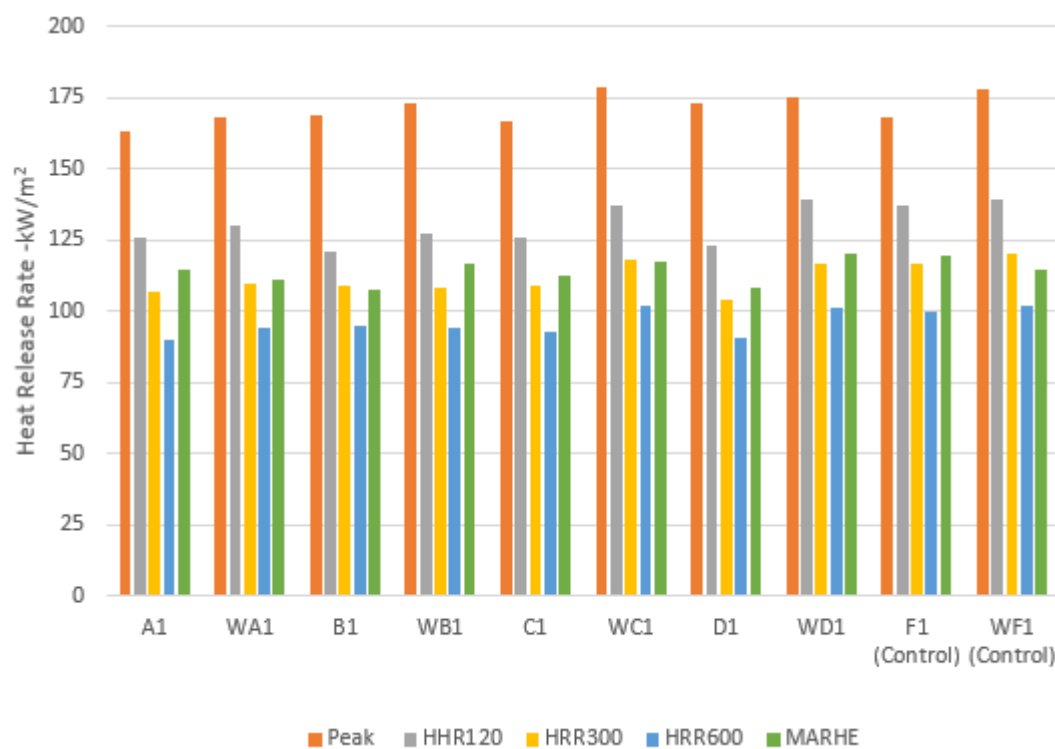
Figure 5 Comparison of HRR data for all specimens of nominal 41mm thickness, exposed to 50kW/m 2 irradiance
