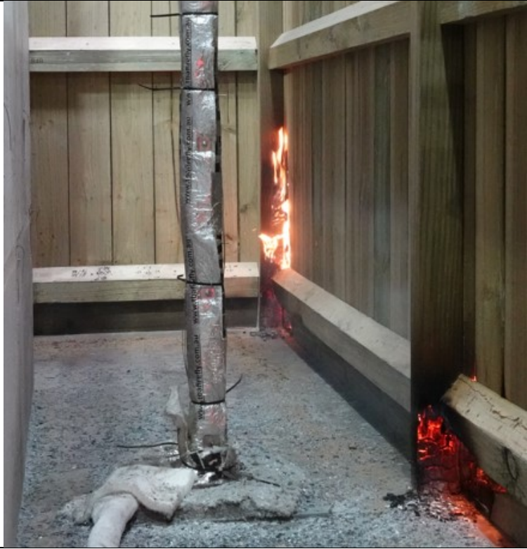
Transition to flaming of posts at interface with palings on side facing simulated building, approximately 87 minutes after commencement of data logging
