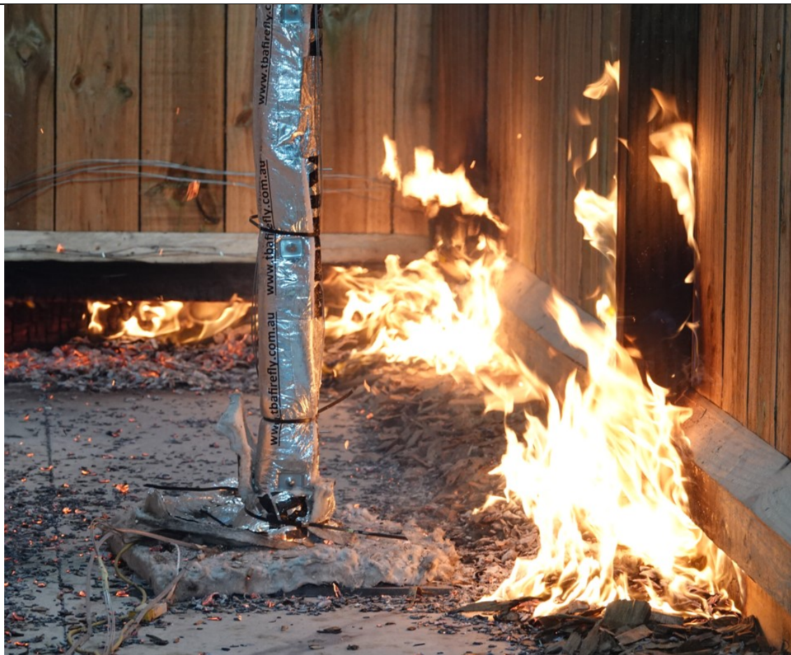
t=21 min–fire spread beyond lower rail at NW corner post and central north intermediate post.
