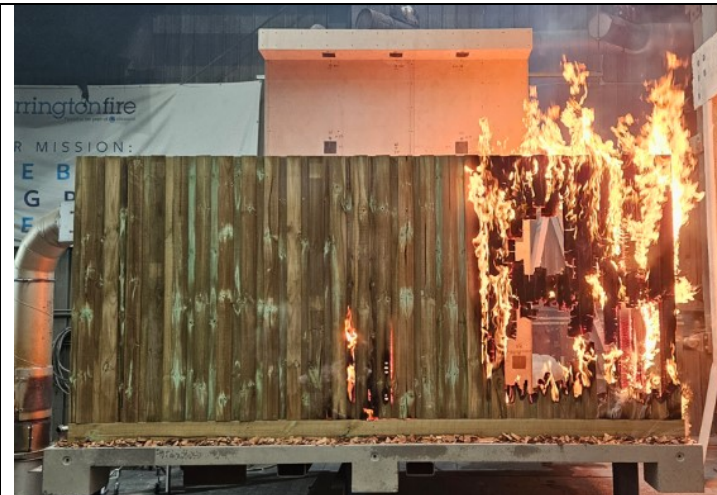
t=34 min fire spread and opening up of west end of north fence with minor burn through by central post
