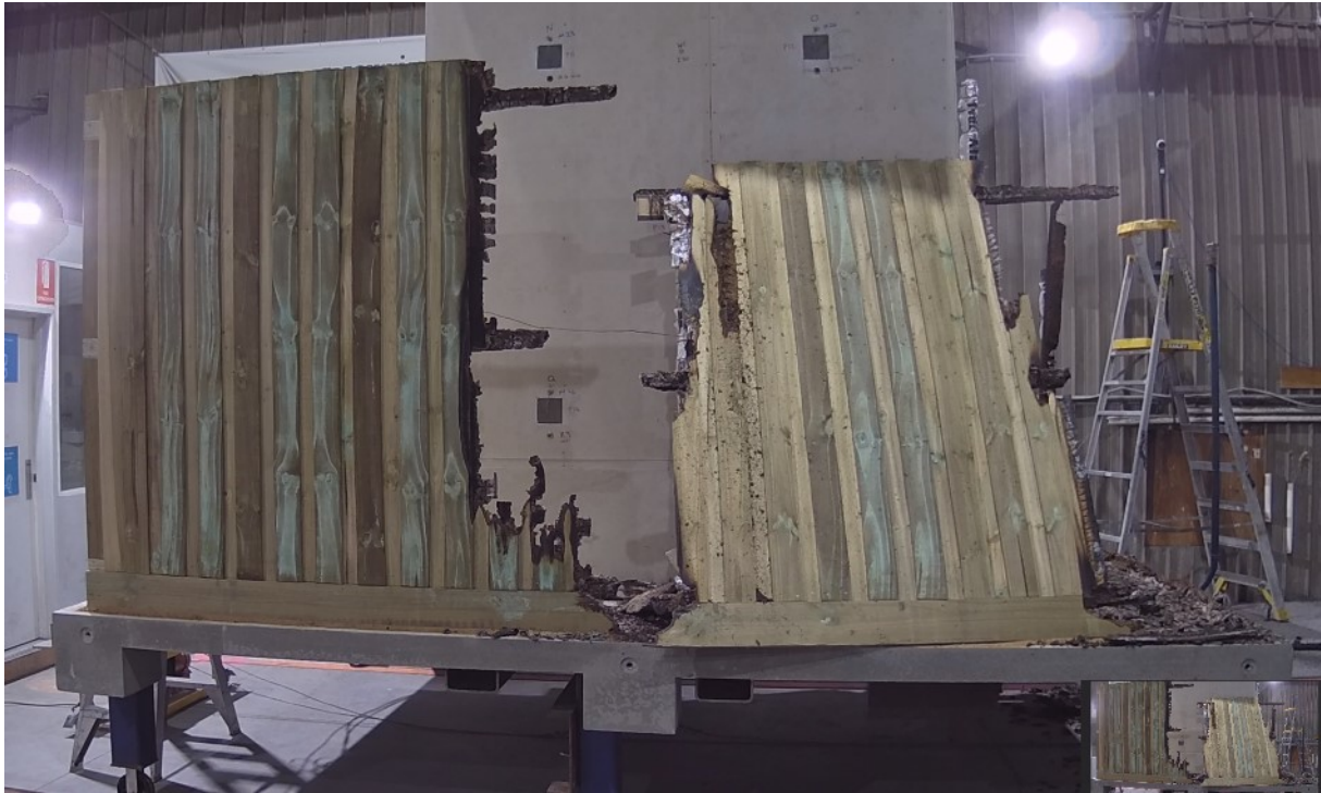
Figure 36 North wall 15.5 hours after commencement with no evidence of ongoing combustion
