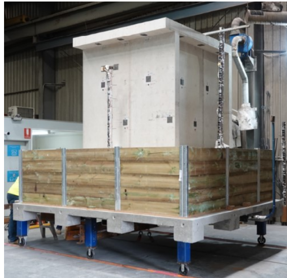
Figure 19 General view of test configuration for sleepers supporting a pathway around a house
