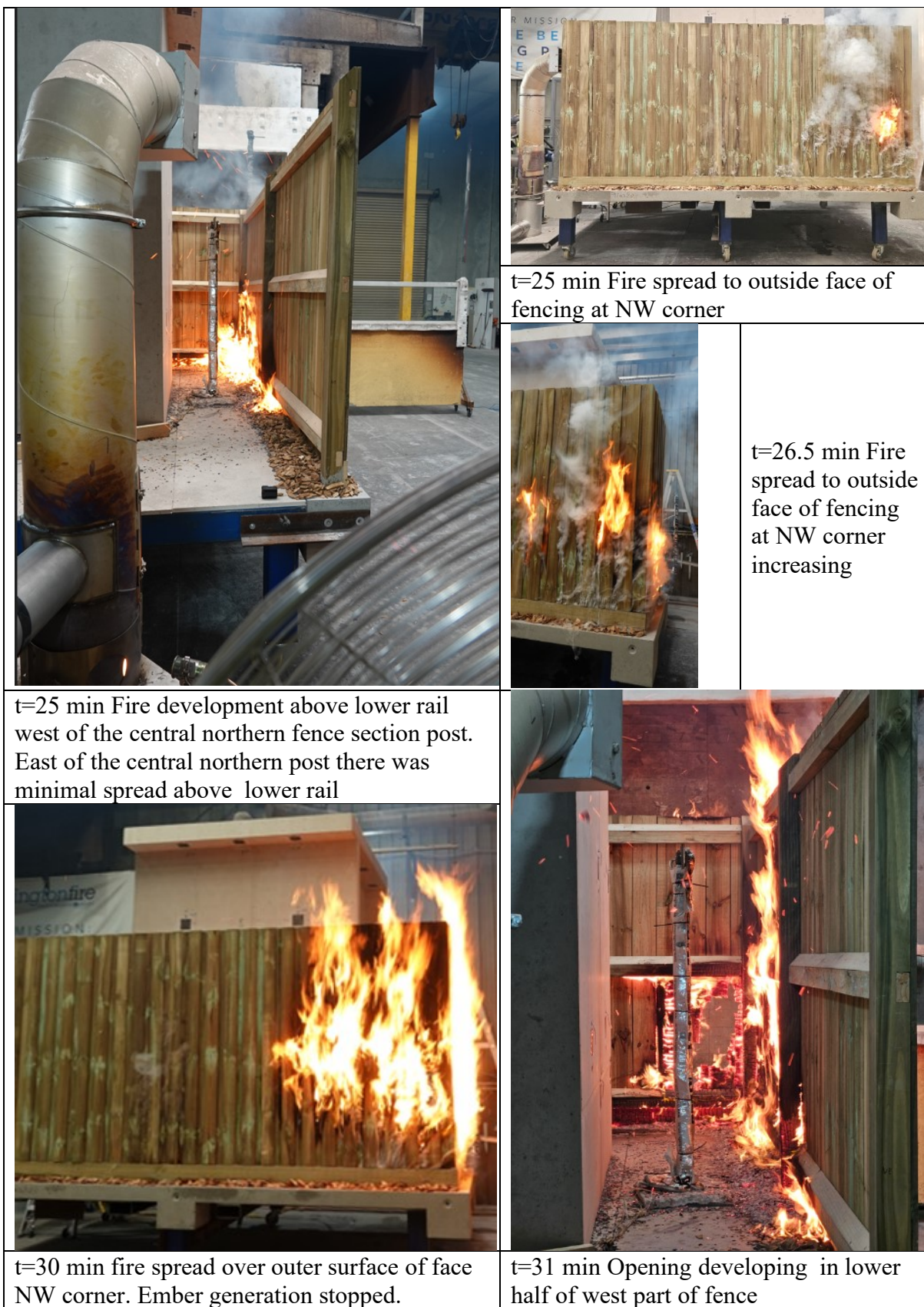
Figure 58 Fire test 1 observations 25-31 minutes
