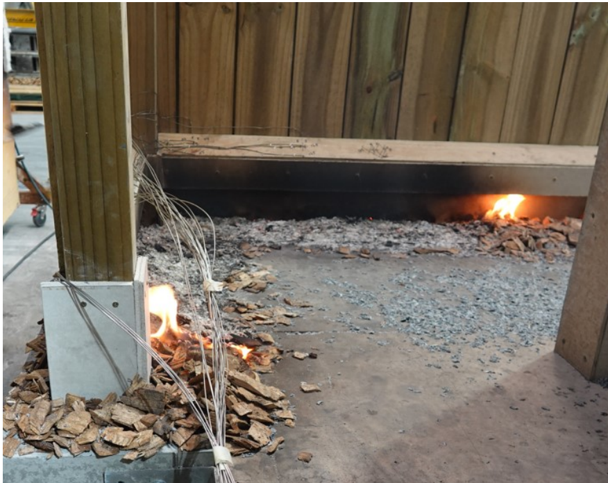
Figure 72 t=112\text{min} fire spread from NW Corner along west and north fences approximately 1m with no ignition of timber fencing.
