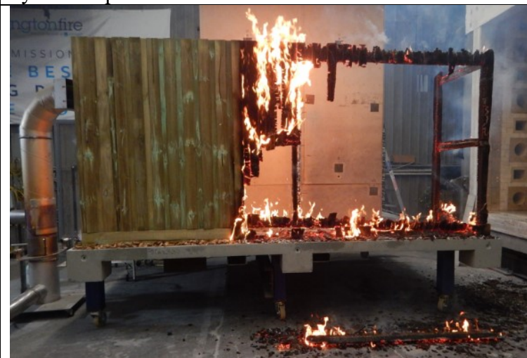
t=50 min air flow terminated - palings on west fence and western end of north fence consumed and central rail at western end of north fence fallen away.
