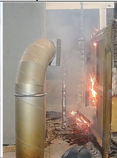
t=62 min test terminated (note northwest corner post and top and bottom rails on north face of specimen collapsed after approximately 58- 60 minutes exposure)
