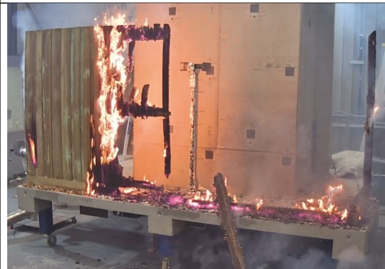
t=62 min test terminated (note northwest corner post and top and bottom rails on north face of specimen collapsed after approximately 58- 60 minutes exposure)
