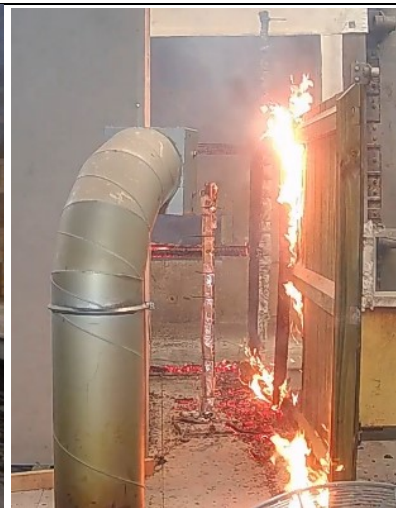
t=50 min air flow terminated - palings on west fence and western end of north fence consumed and central rail at western end of north fence fallen away.
