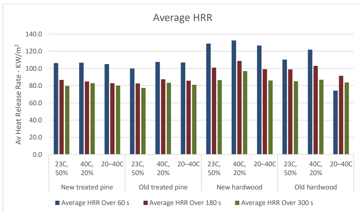
Figure 3 Average HRR for timber palings for periods after ignition when exposed to 25kW/m² - derived from data presented in (Leonard, Blanchi et al. 2006)
