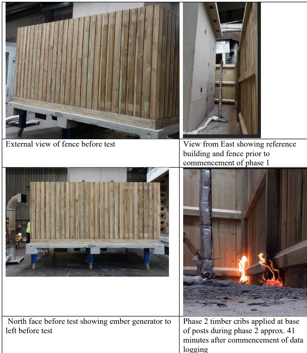
Figure 79 General Arrangement of test 3 paling fence before test.
