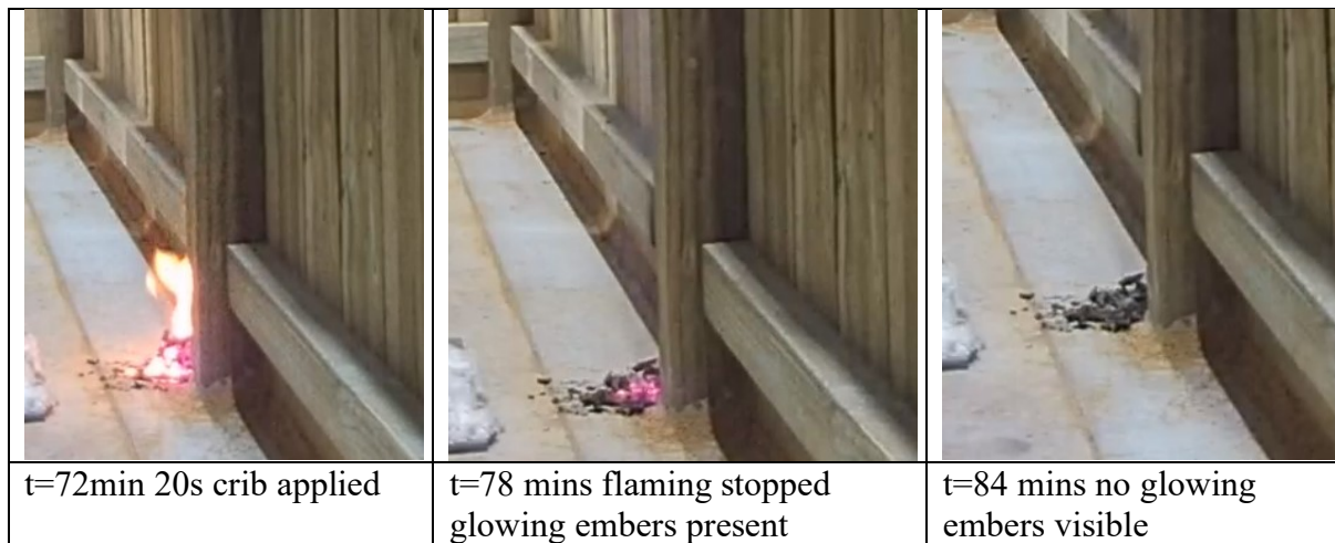
Figure 41 Application of crib to northern fence
