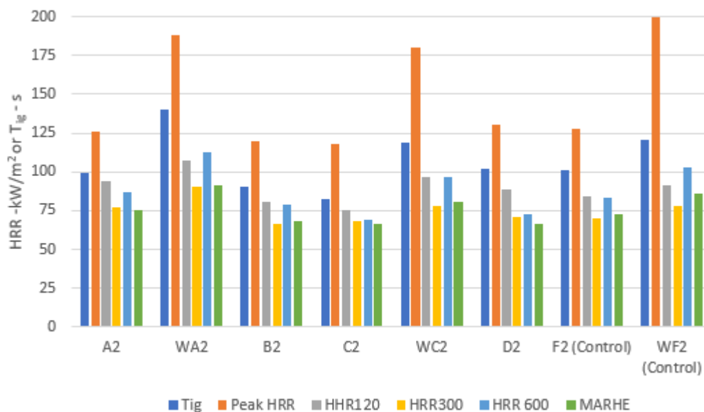
Figure 6 Comparison of HRR data and piloted ignition time for specimens of nominal 12mm thickness, exposed to 25kW/m 2 irradiance
