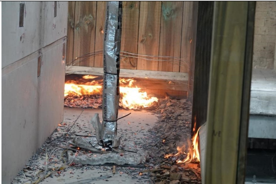
t=17.5 mins – background; involvement in flaming combustion of bottom rail of west fence section and right: involvement in flaming combustion of mid post and adjacent rail up to bottom rail
