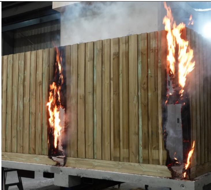
Flaming on outer face of fence approx. 106 minutes after commencement of data logging
