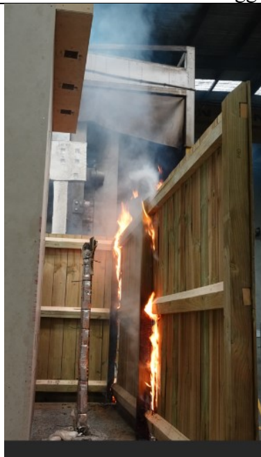
Flaming on side of fence facing the simulated building approx. 106 minutes after commencement of data logging
