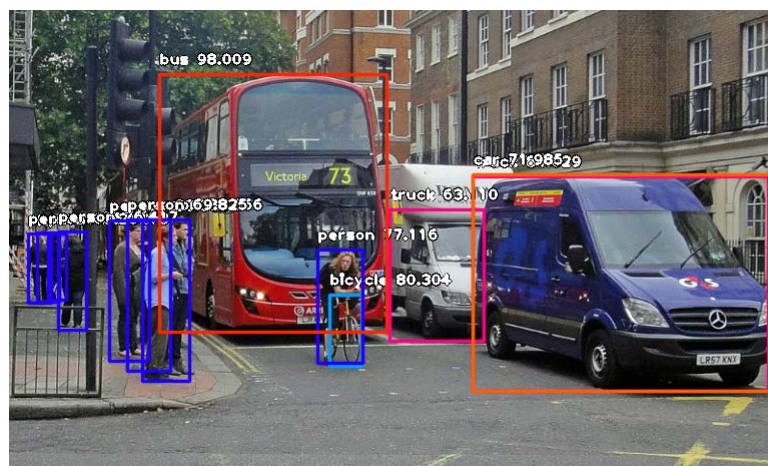
Figure 2: Example of vehicle and human detection
