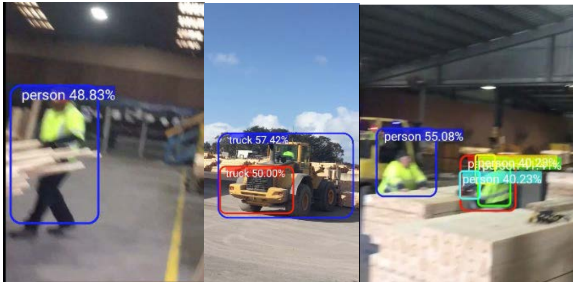
Figure 1: An illustration of object detection system for a single image indicating the % detection threshold.
