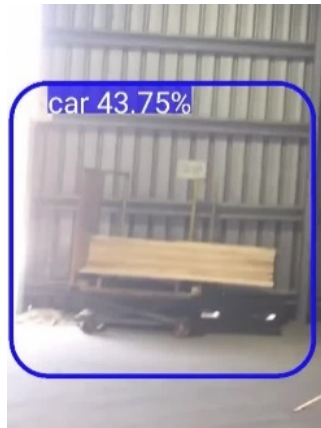
Figure 5: Error – A mobile trolley is recognised as a vehicle
