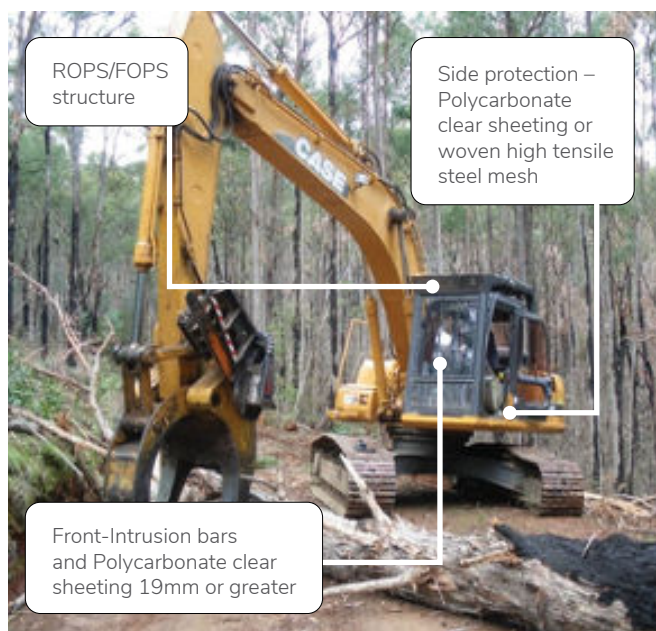
Figure 6: Excavator – timber processing working off the landing fitted with a hydraulic powered saw, fitted with a harvesting or processing head – in an “uncontrolled” environment
