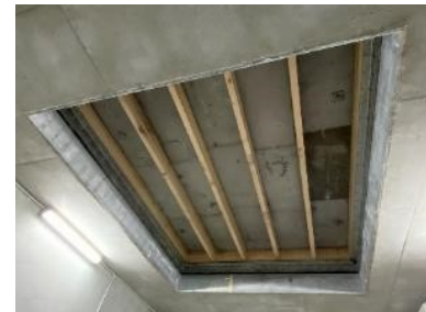
Figure 17 – ATC Floor System Installation (CSIRO Test Facility)
