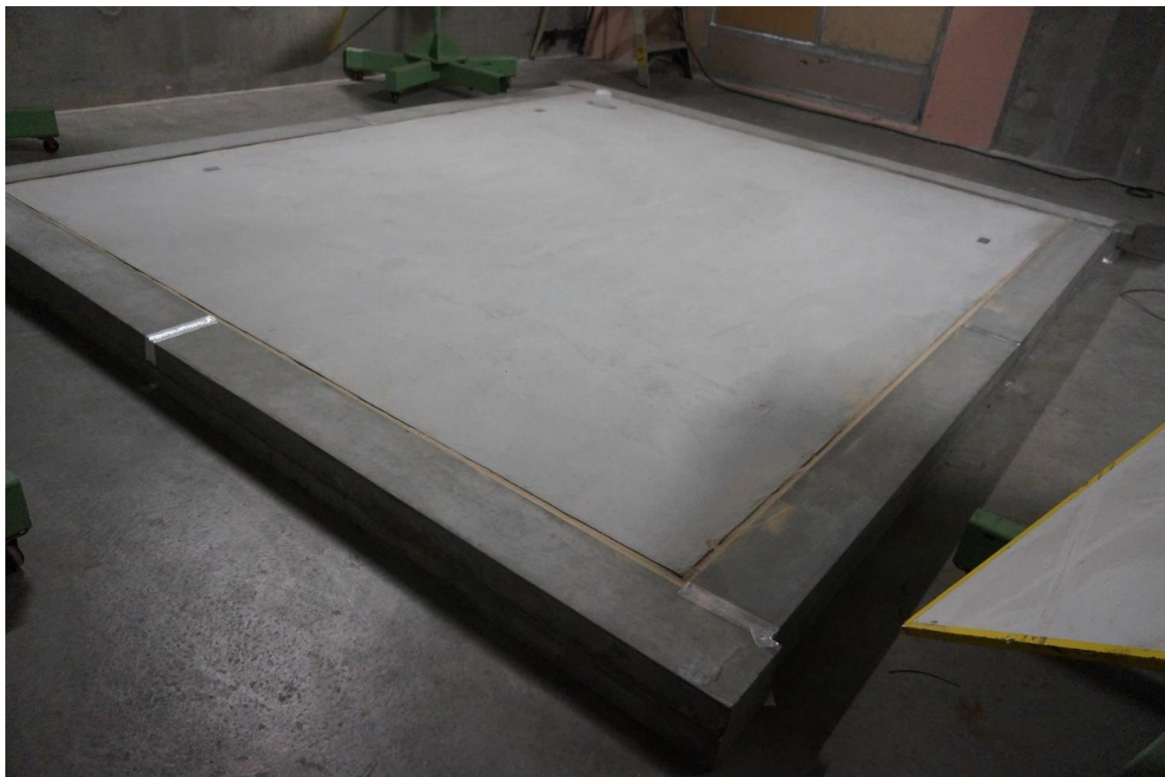
ATC Composite Panel, installed in laboratory, with concrete sleeper skirting
