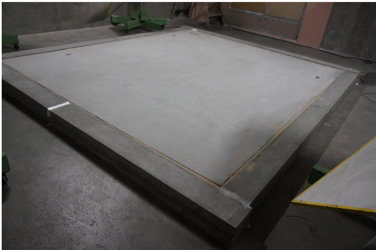
ATC Composite Panel, installed in laboratory, with concrete sleeper skirting (as tested)
