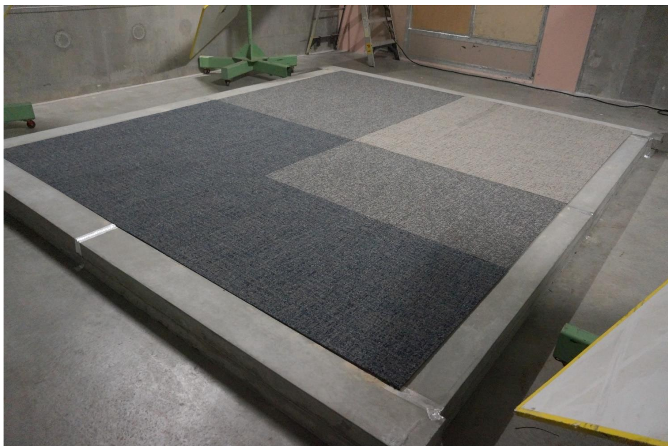
Carpet on top of ATC Composite Panel (as tested)
