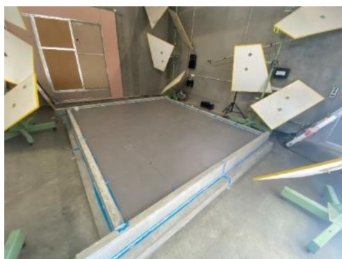
Sleepers with Acoustic Sealant Treatment
