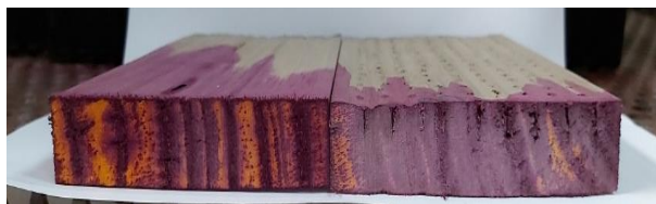
Figure 23. Penetration images of laser incision patterns following treatment. Photo: Rhianna Robinson.
