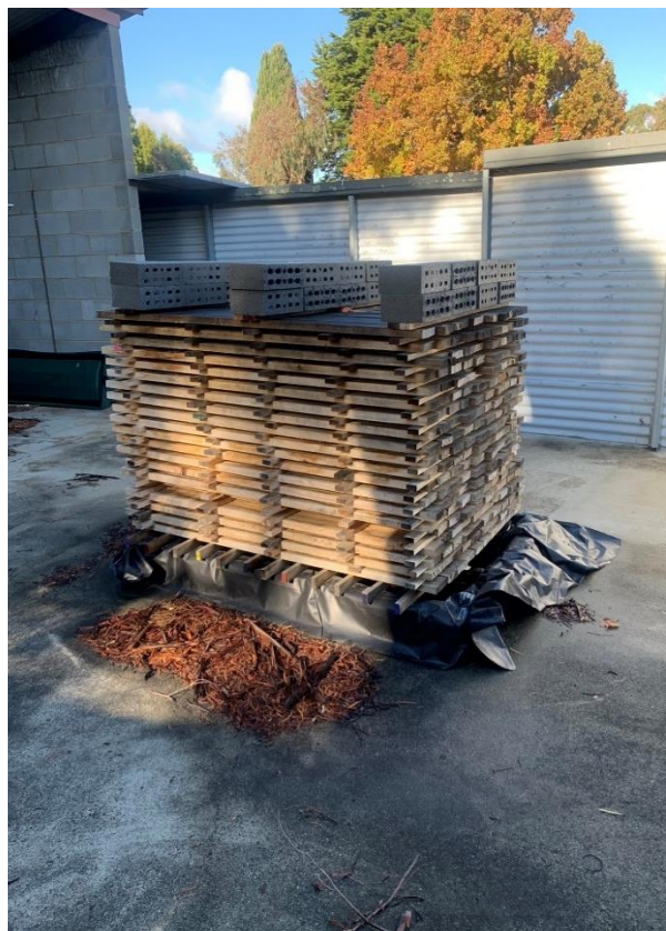
Figure 6. Unsheltered rack of boron treated shining gum boards air drying at T40, with leachate collection set up underneath. Photo: Kyra Wood.
