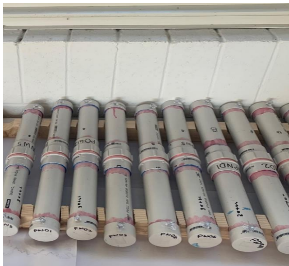
Figure 4. Diffusion cup apparatus. Photo: Kyra Wood.
