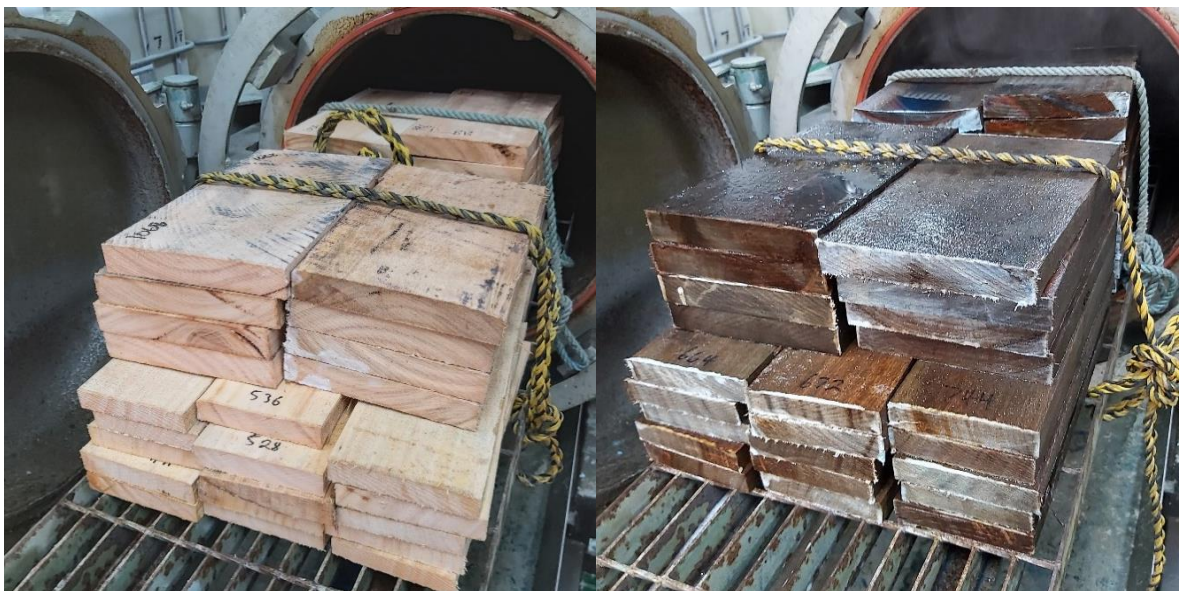
Figure 10. Samples before treatment (left) and after treatment (right). Photo: Stuart Meldrum.
