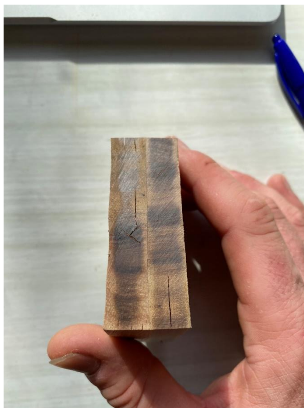
Figure 53. Eucalyptus nitens sample following the delamination test (Compression ratio: 37%; pressing temperature: 150°C; pressing time: 20 min; total delamination 0.0%). Photo: Benoit Belleville.
