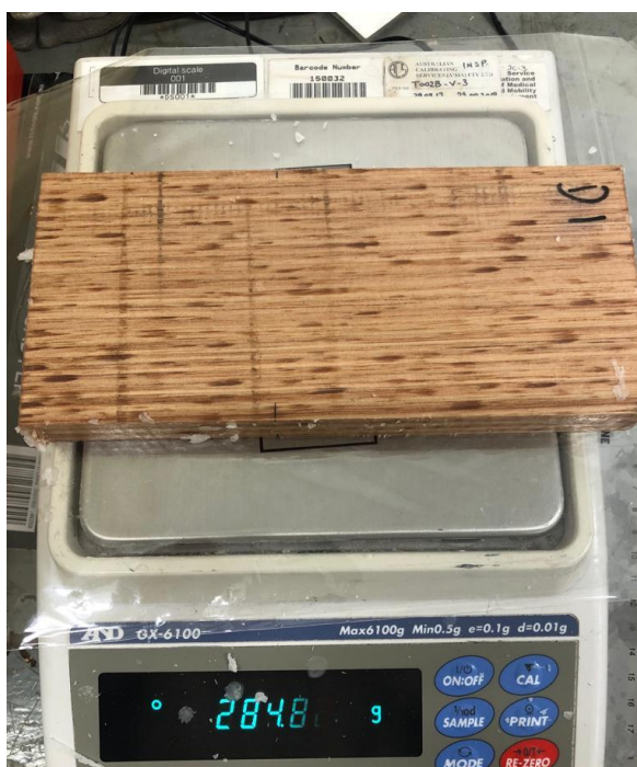
Figure 2. Samples being weighed after dipping. Photo: Ros Ghani
