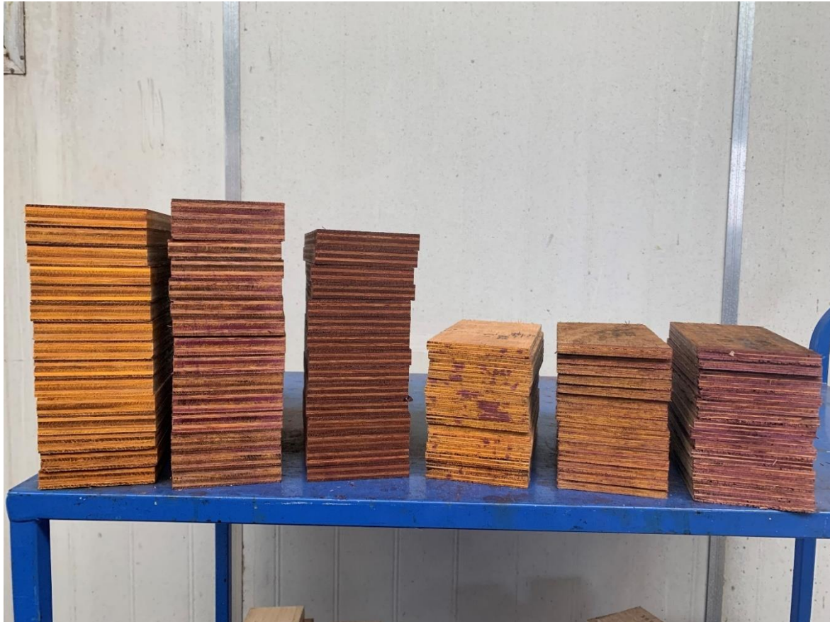
Figure 17. Penetration images of veneer-based samples following treatment with charge 1 + MCA + V spotted gum plywood; treated spotted gum plywood; veneer treated spotted gum; untreated Tasmanian oak plywood; treated Tasmanian oak plywood; and veneer treated shining gum. Photo: Rhianna Robinson.
