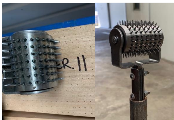
Figure 20. Spiked roller incision set-up. Photo: Rhianna Robinson.
