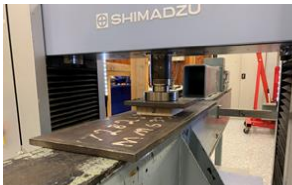
Figure 26. Static compression tests. Photo: Rhianna Robinson.
