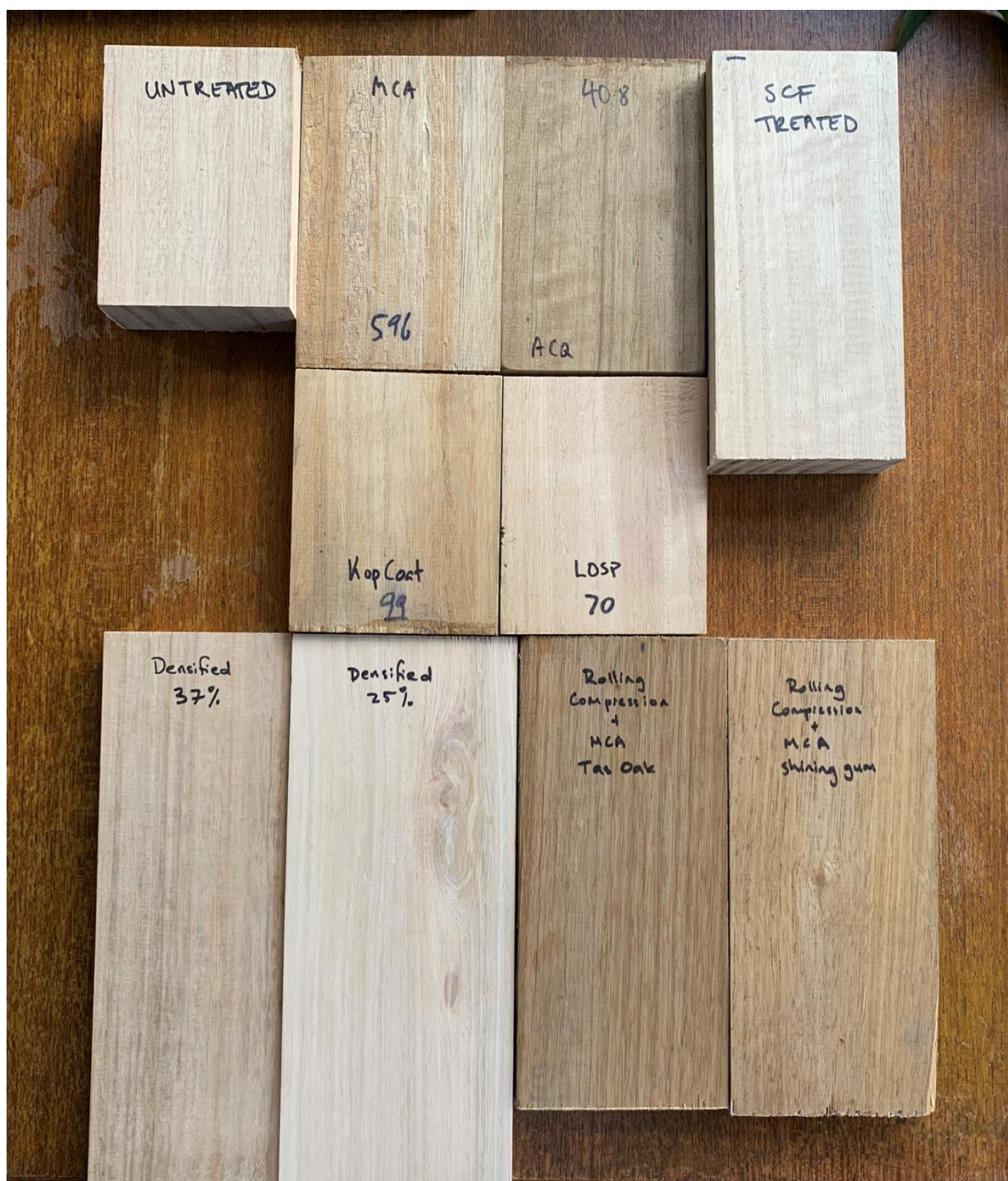
Figure 66. Treated and modified samples next to each other for comparison. From top left to bottom right: untreated shining gum; MCA treated shining gum; ACQ treated shining gum; supercritical fluids treated shining gum (see NT047/NIF108 for more detail on SCF treatment); Kop-Coat treated shining gum; LOSP treated shining gum; 37% compression ratio TM densified shining gum; 25% compression ratio TM densified shining gum; rolling compression + charge 3 + MCA + adjuvant V treated Tasmanian oak; and rolling compression + charge 3 + MCA + adjuvant V treated shining gum. Photo: Kyra Wood.
