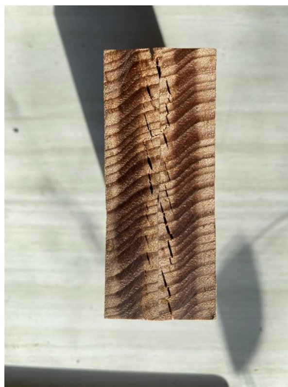
Figure 52. Eucalyptus delegatensis sample following the delamination test (Compression ratio: 37%; pressing temperature: 150°C; pressing time: 10 min; total delamination: 13.0%). Photo: Benoit Belleville.
