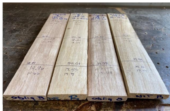
Figure 46. Example of spring back from preliminary trial. Photo: Benoit Belleville.
