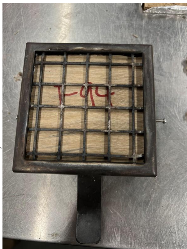
Figure 55. Grid used to prevent sample from delaminating during cone calorimeter test. Photo: Wenxuan Wu.
