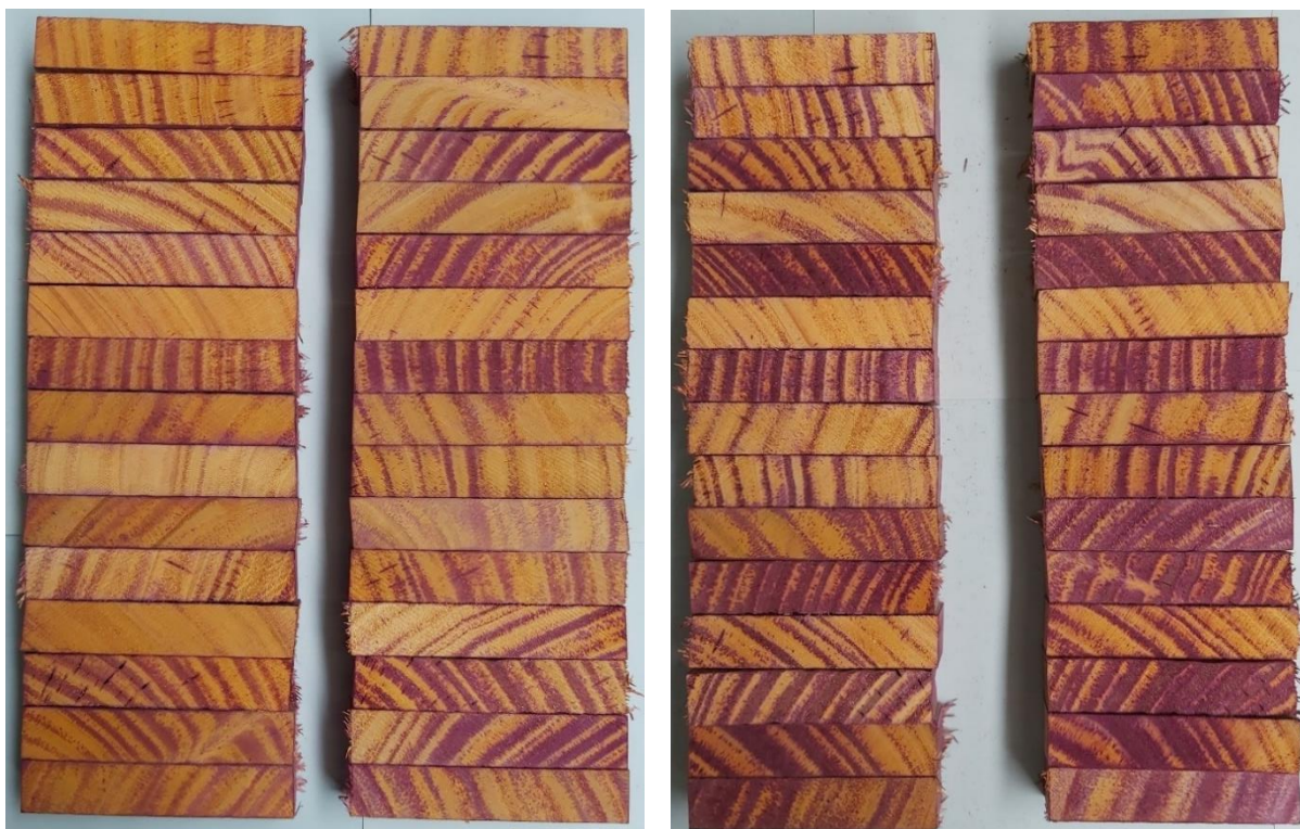
Figure 13. Penetration images of treated shinning gum from charge 3+MCA+adjuvants, left to right, showing copper penetration of MCA, MCA + B, MCA + S and MCA + V. Photo: Stuart Meldrum.
