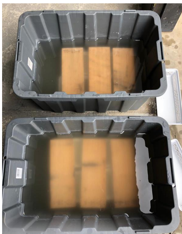
Figure 1. Samples being dipped in a boron-based preservative solution. Photo: Ros Ghani
