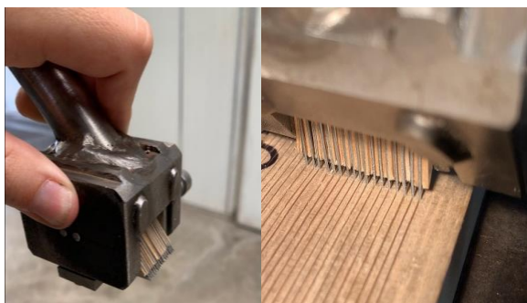
Figure 18. Blade incision set-up. Photo: Rhianna Robinson.
