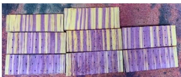
Figure 24. Penetration images of laser incision patterns following treatment. Photo: Rhianna Robinson.
