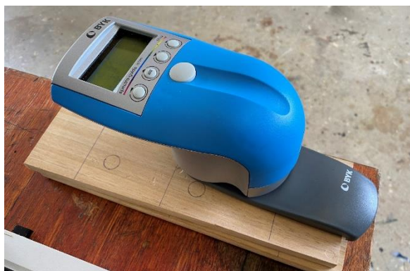
Figure 42. BYK-Gardner digital colour apparatus Photo: Benoit Belleville.
