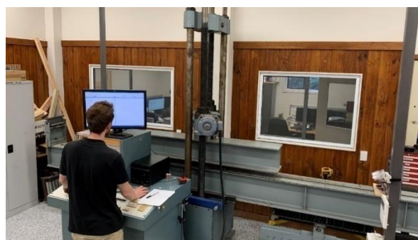
Figure 27. Static compression set up. Photo: Rhianna Robinson.
