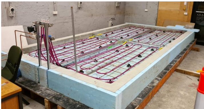
Figure 23: Heated slab with insulated forma, and hydronic heating coils attached to the reinforcement.
