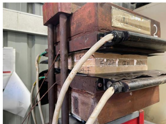
Figure 8. CLT parent billets in the press.
