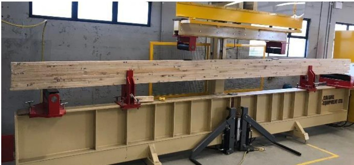
Figure 5. Elevation view of the tested beam (a), Bending test of a combined glulam sample (b)
