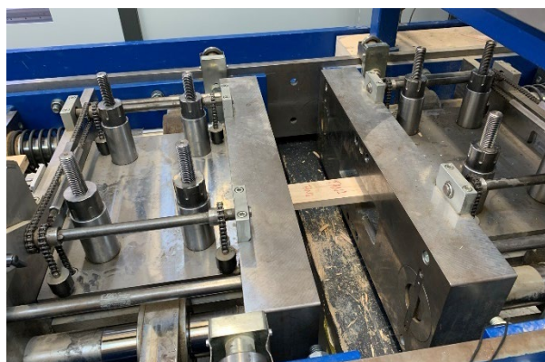
Figure 2: Specimen in the tension testing machine
