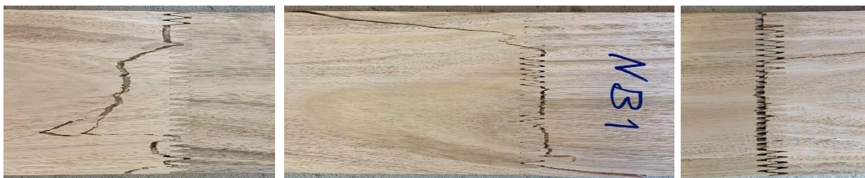
Figure 10. Typical failure of the finger joints in series one and two
