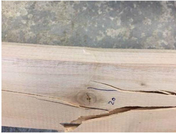
Figure 2 Failure mode of the E. nitens boards in bending
