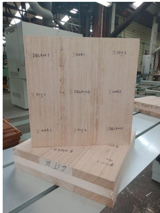
Figure 7. CLT parent billets.
