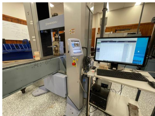
Figure 9. CLT and GLT blocks were block shear tested in both wet and dry condition, using a universal testing machine.
