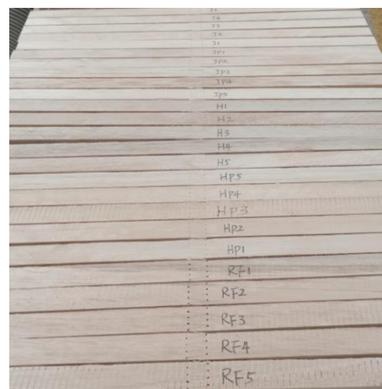
Figure 5. CLT cut into blocks for shear test.
