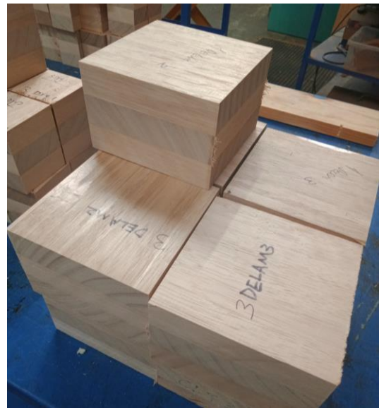
Figure 5. CLT cut into blocks for shear test.
