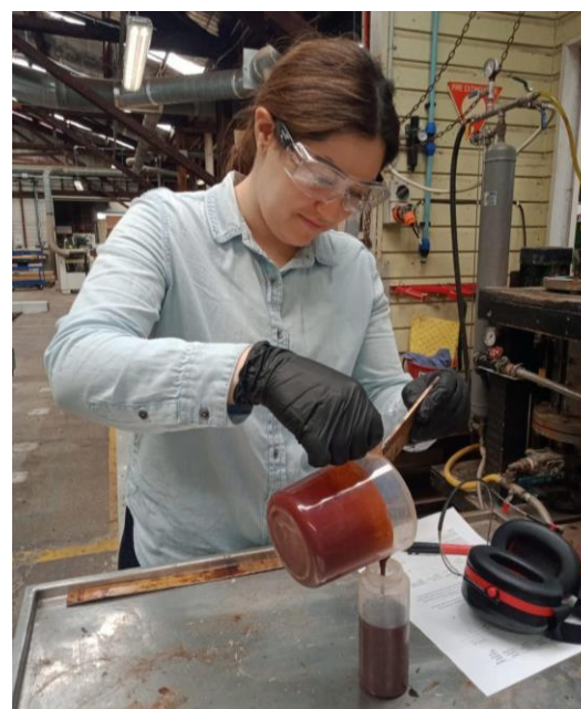
Figure 2. Azin mixing RF glue for the sample production at DAF research facility.
