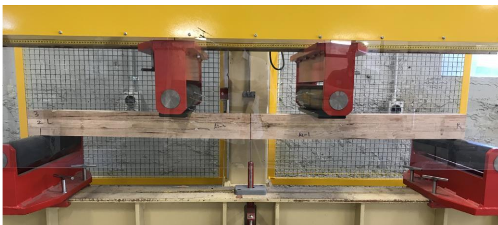
Figure 1: Four-point bending test setup (Sample ref. A-1)
