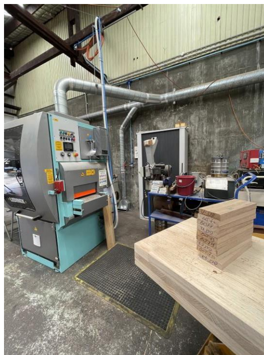
Figure 3. Face milling equipment at the DAF research facility, with some of our E. nitens sample boards waiting to be milled.
