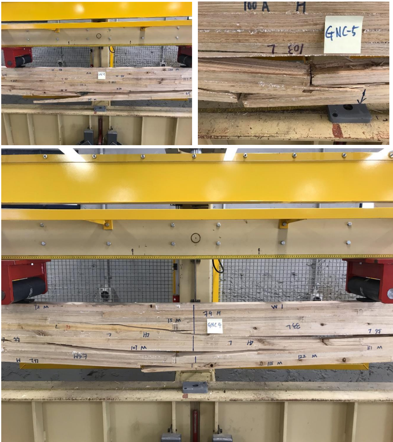
Figure 4: Failure mode of the glulam samples
