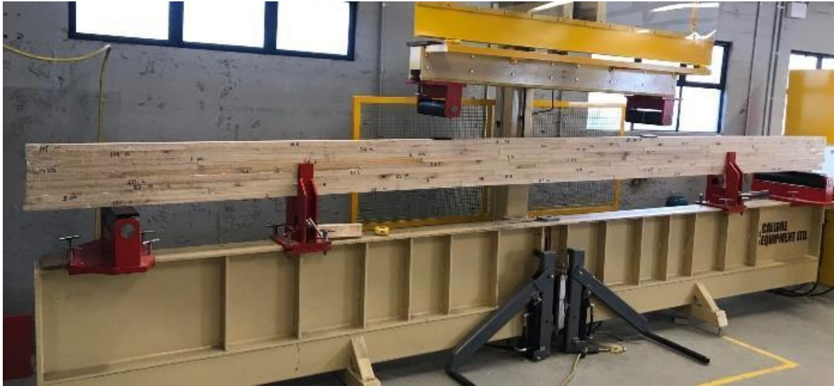
Figure 2: Bending test of a combined glulam sample
