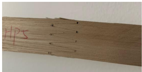
Figure 13. (Top) 10mm finger joint samples after 3 point bending test showing signs of rupture.
