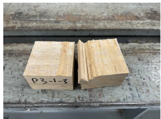
Figure 11. CLT block showing signs of delamination
