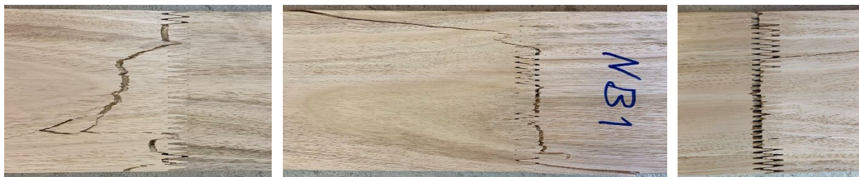
Figure 3; Typical failure of the finger joints in series one and two
