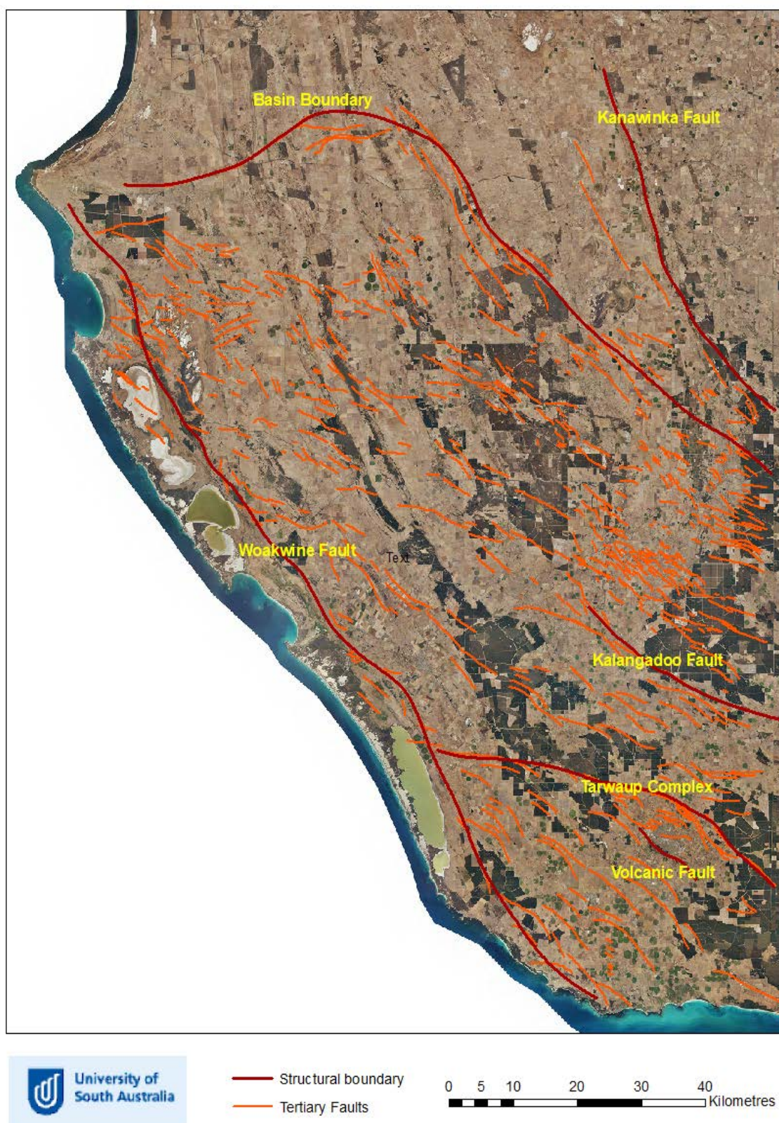
Figure 3: Tertiary surface faults and the major structural faults within the Gambier Basin
