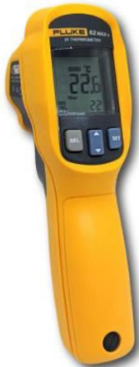
Figure 3.8 – Photo of the thermometer (model: FLUKE-62-MAX)
