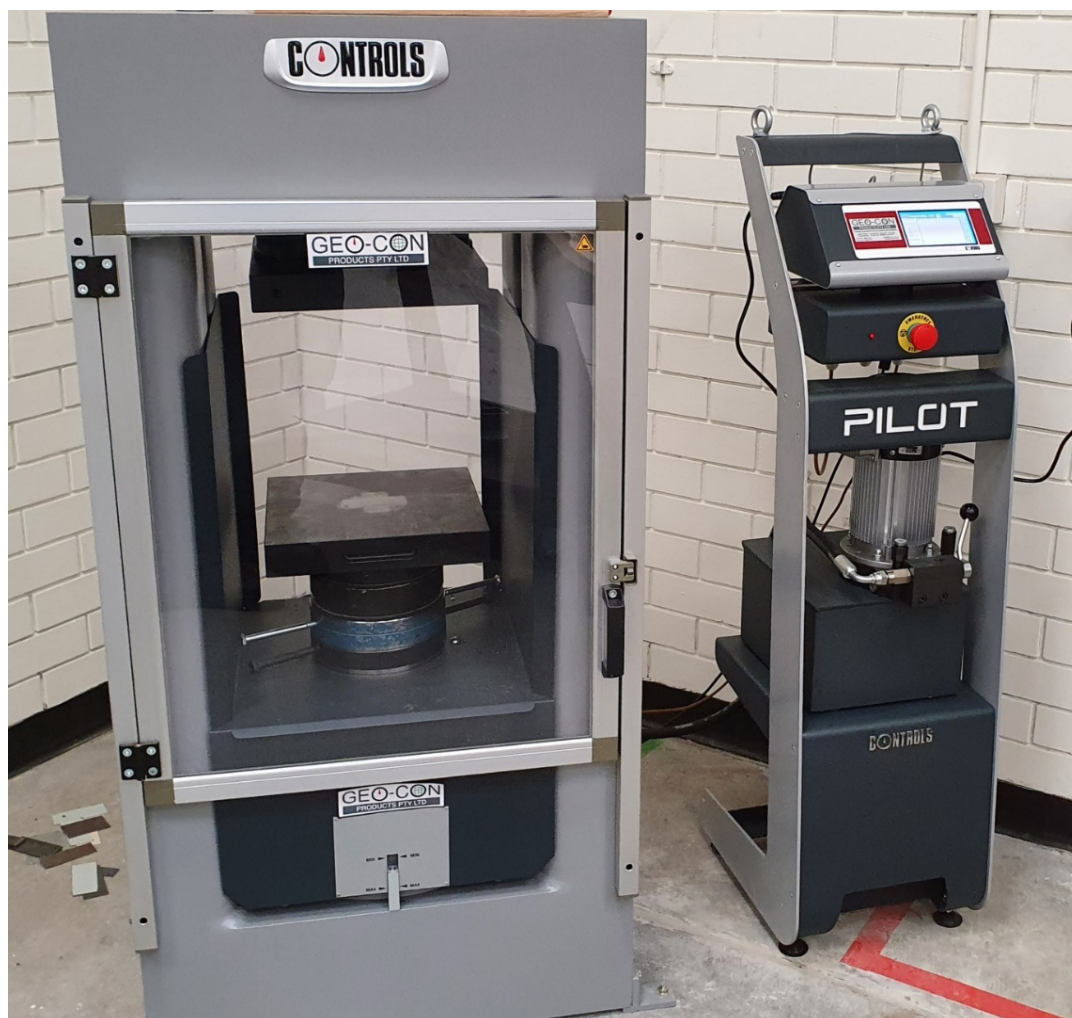
Figure 3.2 – Photo of the compression testing machine (CONTROLS Compression Tester, Model PILOT SMART-Line)
