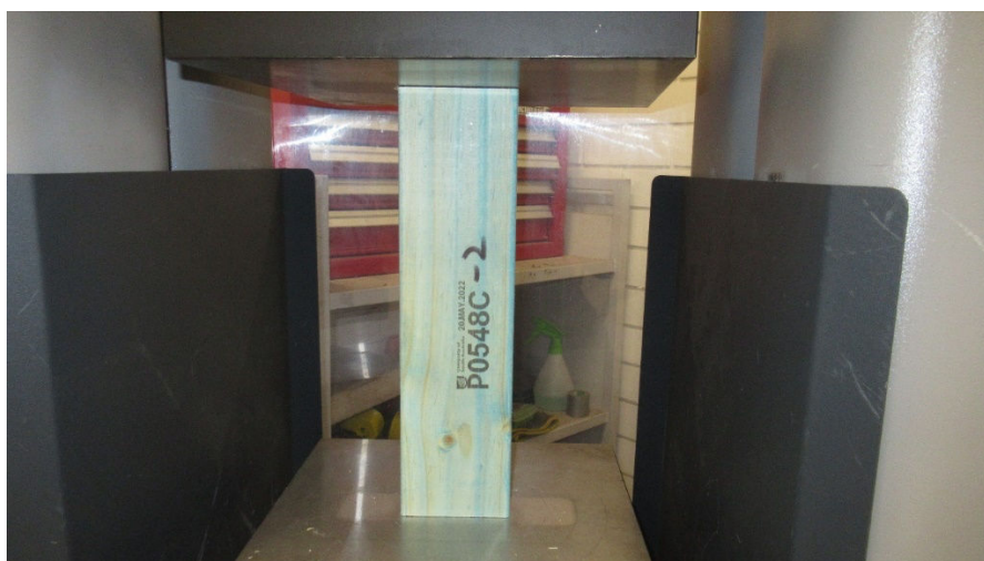
Figure 3.23 – Test setup for measuring compression strength parallel to grain (90x35 mm specimen)
