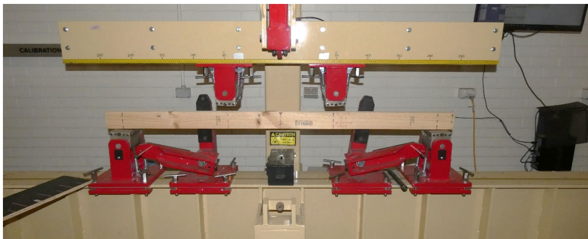
Figure 3.9 – Test set-up for measuring the apparent modulus of elasticity and the bending strength (90x35 mm specimen)
