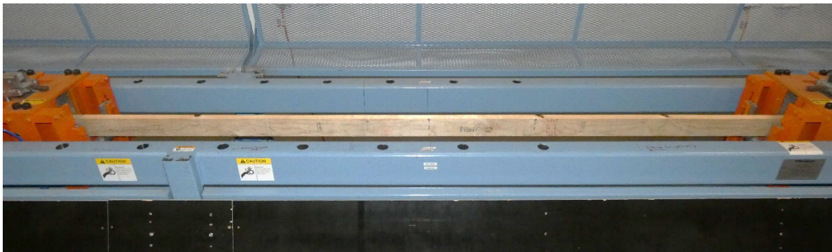
Figure 3.17 – Test set-up for measuring the tension strength parallel to grain (90x35 mm specimen)
