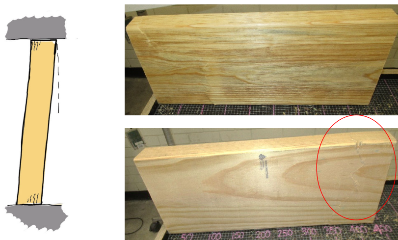
Figure 3.28 – Compression test failure by rotation of specimen
