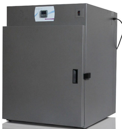
Figure 3.7 – Photo of the oven (model: Steridium DG-160)
