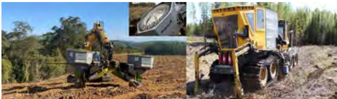
Figure 7 Two currently available commercial tree planting machines. Bracke P22.b planter with seedling carousel (left); PlantMax automated planter (right).
