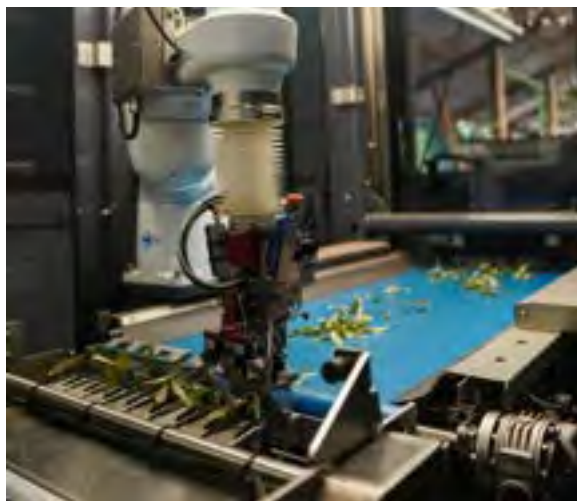
Figure 21 TTA-ISO CuttingEdge automated cutting planting machine on eucalyptus
