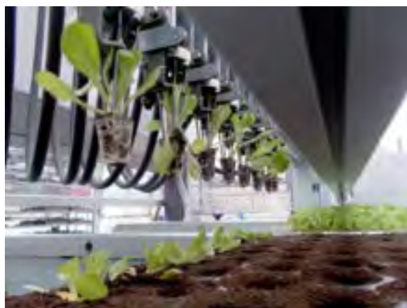
Figure 20 Atlantic Man Multi-Grip Automatic Transplanting Machine (TPA)
