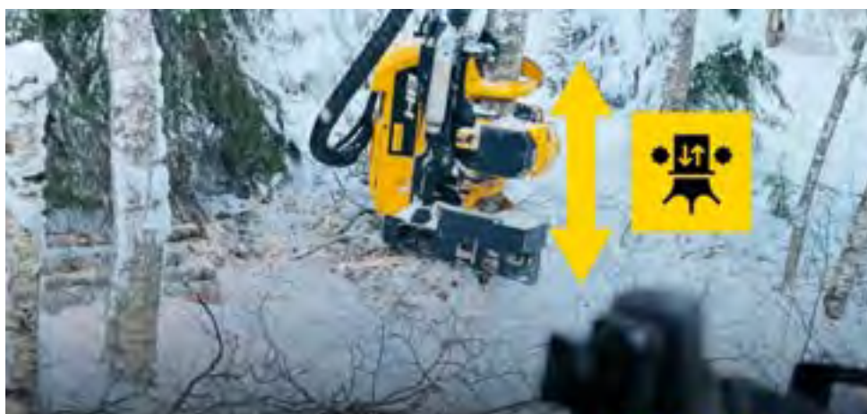
Figure 15 Ponsse OptiFelling automated assistant and control system improves cutting precision and operator safety by managing pre-tensioning during the cut.
