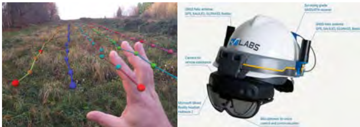
Figure 4 (Left) AR projection of planting lines & seedling positions (de Miguel-Diez & Purfurst, 2025); (Right) V-Labs Augmented Reality helmet.
