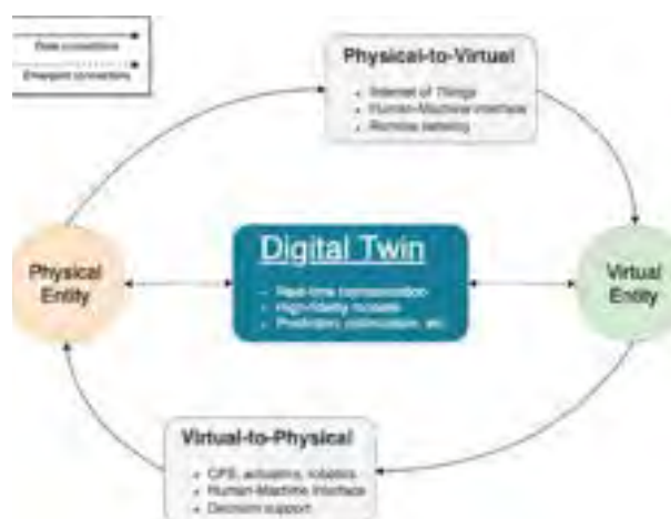
Figure 11 Digital Twin - Architecture overview (Purcell and Neubauer, 2023)
