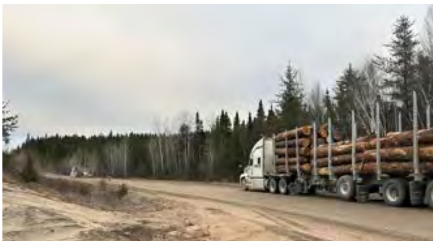
Figure 19 Kratos Unmanned Systems self-driving trucks platooning in Canada, 2025, in conjunction with FPInnovations.
