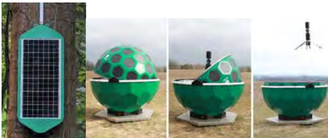
Figure 13 Silvanet fire sensor on a tree (left); a Dryad Networks UAV takes off from its solar-powered “hangar” (right).
