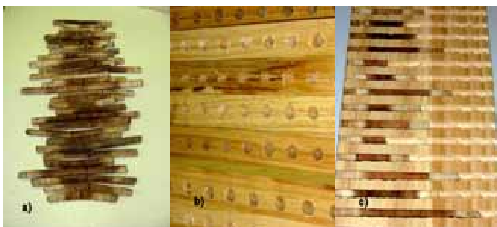
Figure 1. a) oven-dry blackwood cores, b) drilled pine boards ready for cores, and c) dressed boards with blackwood cores ready for colour measurement
