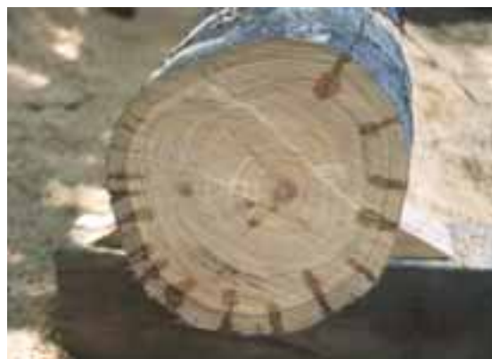
Fig. 3.29(two pictures): End sections of log that was allowed to dry and then re-wet. The watermarks indicate the extent of surface cracking.
