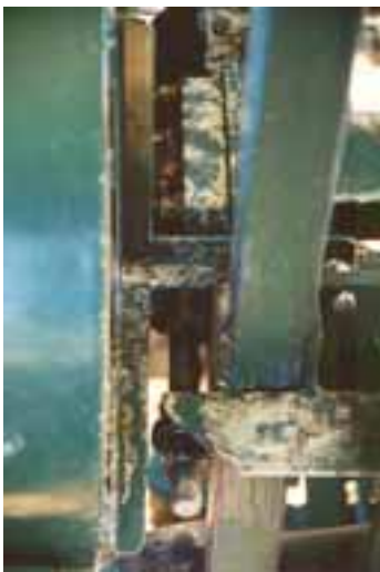
Fig. 6.1 (left): Thread, nut and bearing plates that require lubrication.
