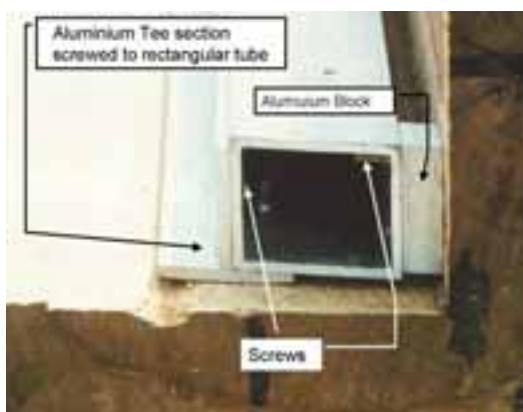
Fig. 3.14 (left): End section of straightedge with spacer block to clear log.
