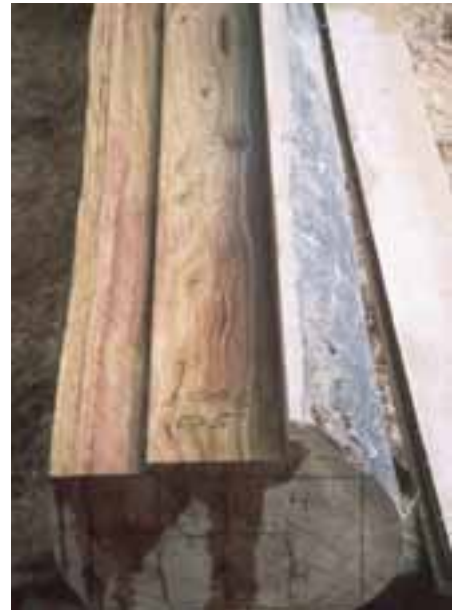
Fig. 3.24 (left): Log set up with the wedge to check any log stress movement.
