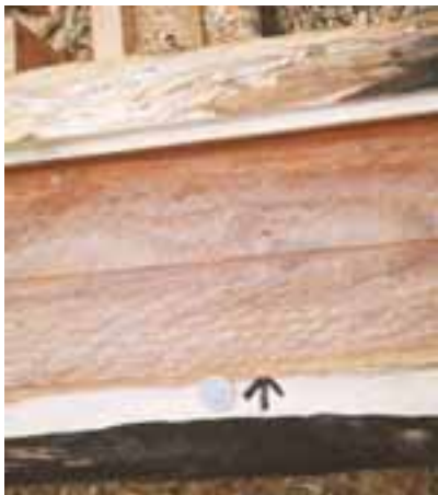
Fig. 5.10 (left): Sugar Gum log with double 100 mm wide horizontal cut showing a step in the face.
