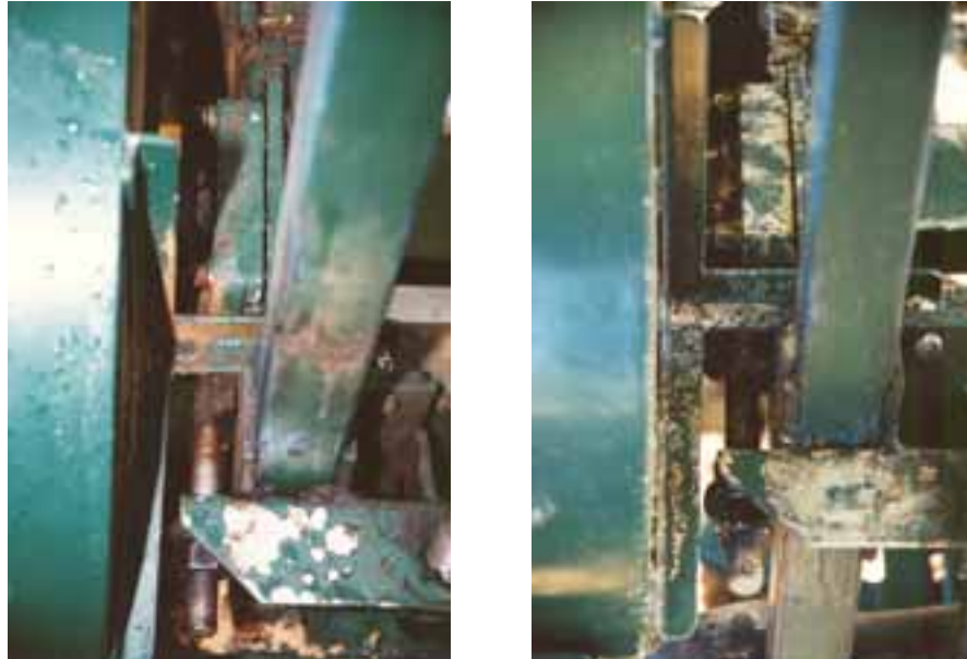
Fig. 3.12 (two pictures): Tension adjuster (viewed from above) on the front bearing behind the idler wheel of the Farmill.
