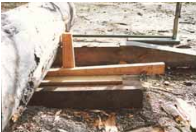
Fig. 3.24 (left): Log set up with the wedge to check any log stress movement.
