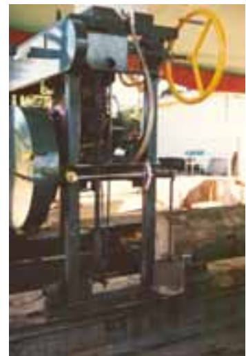
Fig. 6.1 (left): Thread, nut and bearing plates that require lubrication.
