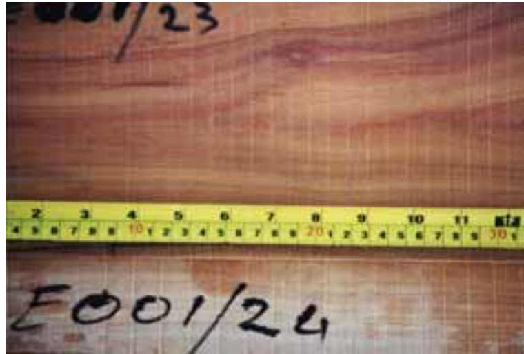
Fig. 7.12 (left): Tooth marks on boards cut with Carbide-tipped blades in Swamp Yate. Top board cut with 32 mm blades and bottom board cut with 50 mm blade.
