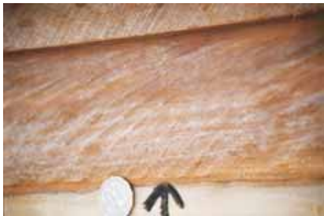
Fig. 5.10 (left): Sugar Gum log with double 100 mm wide horizontal cut showing a step in the face.
