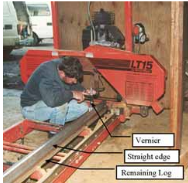
Fig. 3.16 (left): Calliper used as a depth gauge to measure the distance from the straightedge to the cut surface.
