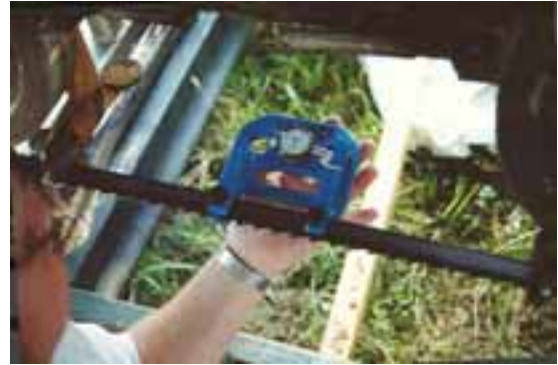
Fig. 3.18 (right): Load cell and weight indicator attached to the Laidlaw mill to measure the tension.
