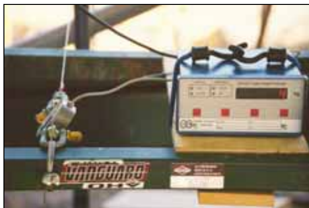
Fig. 8.3 (left): Power head and carriage attached to the constant feed-speed cable.
