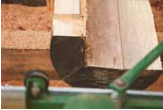
Fig. 5.16 (left): Second last cut of double depth sawing trial.
