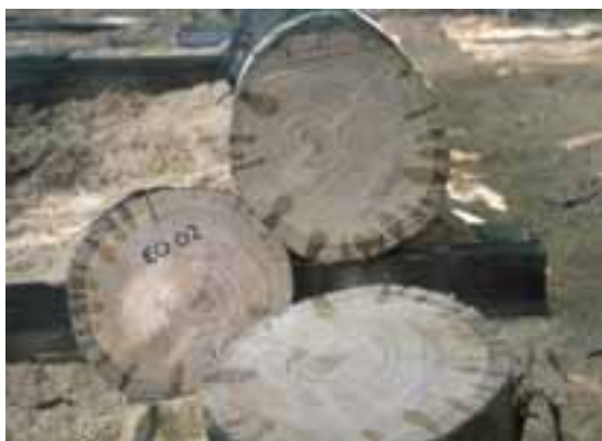
Fig. 3.29(two pictures): End sections of log that was allowed to dry and then re-wet. The watermarks indicate the extent of surface cracking.
