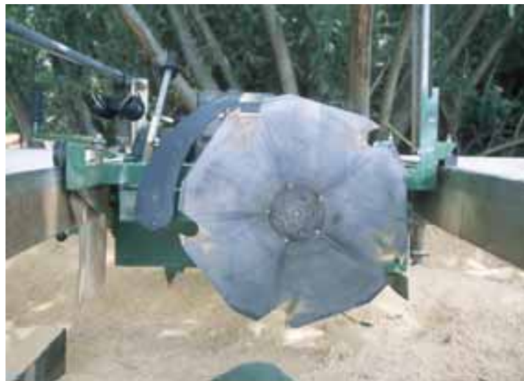
Fig. 3.8: Blade showing the direction of the water flow from the centre of the blade to the gullet and extensive build-up at the back and base of the gullet.
