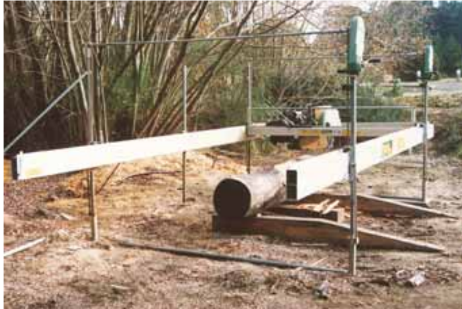
Fig. 3.1: Lucas Mill set up for sawing at the TTC, Creswick.
