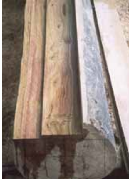
Fig. 5.1: A Swamp Yate log that has been sawn with horizontal cuts and is ready for measurement.
