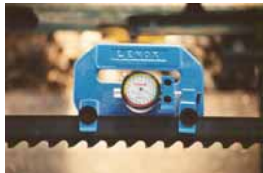
Fig.7.1 (left): Large Lenox tension meter being demonstrated by the Regional Sales Manager, Amercia Saw and Mfg Company.
