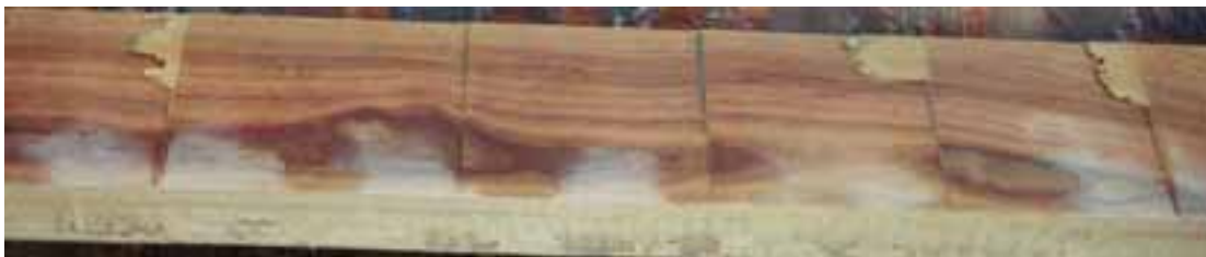
Fig. 7.11: Brown Mallet log sawn with the 50 mm Carbide-tipped blade showing positions along the log where the blade dived and the sawing head was reversed to recover cutting line.
