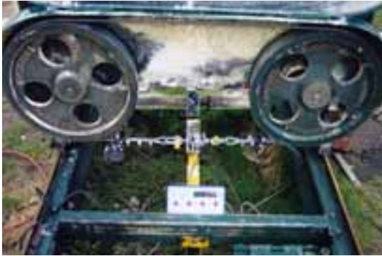
Fig. 3.18 (right): Load cell and weight indicator attached to the Laidlaw mill to measure the tension.
