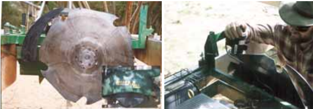
Fig. 3.4 (left): Lucas mill with the guard removed and the blade in the vertical position. (Insert shows the saw with the guard in place). NB: The saw should not be used without the guard in place.
