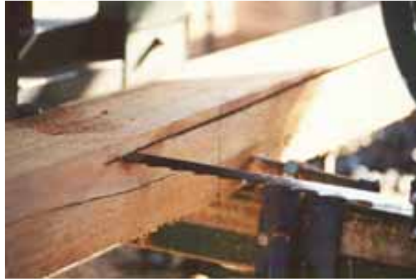
Fig. 8.25: Diving cut in Sugar Gum due to incorrect speed setting.
