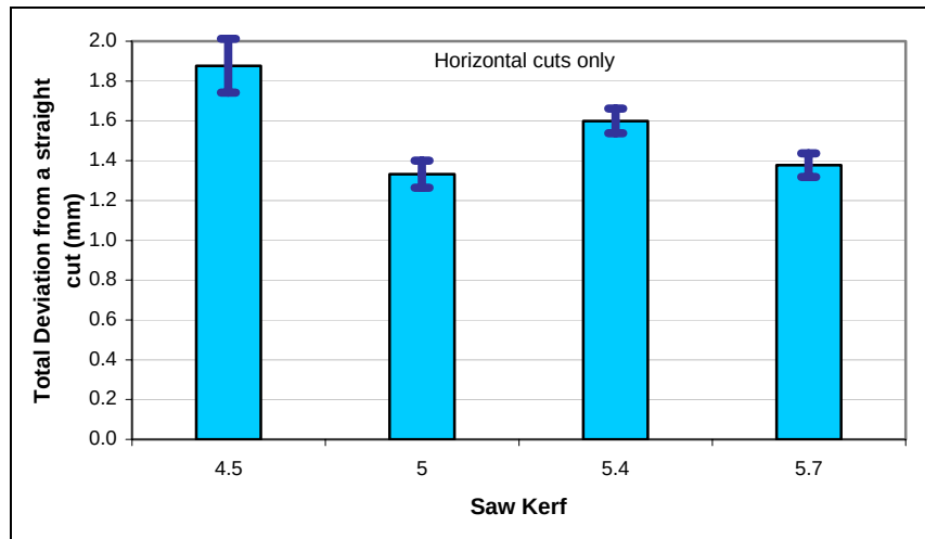
Fig. 5.8: Deviation from straight cut for cuts in the horizontal orientation by saw tip width (bars = S.E.).
