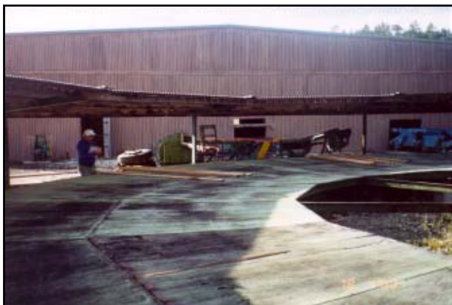
Figure 19: Appearance grading of green boards grouped by log on the round table as they come out from the re-saw.
