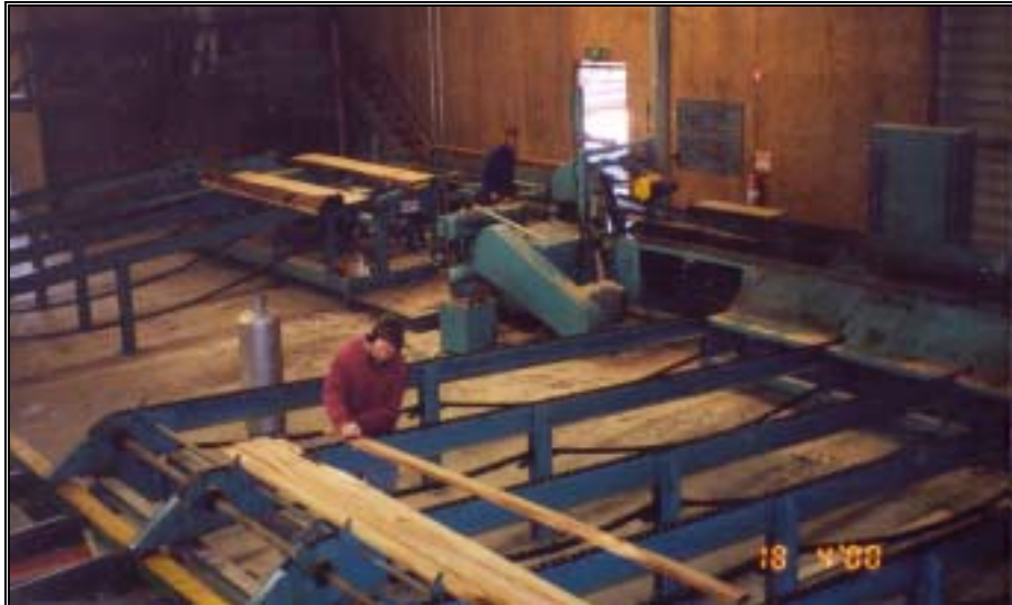
Figure 18: Application of log color, log number and sequential board numbers to boards grouped (by log) off the re-saw bench.
