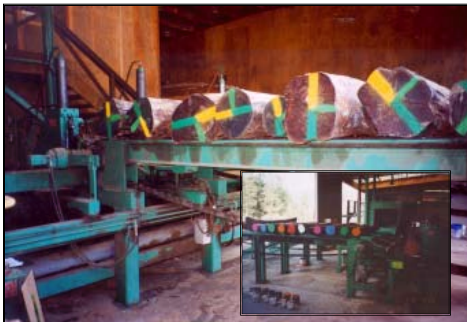
Figure 17: North, south and west are indicated on the large end of logs for sawyer to align central cant with the north-south orientation. They are painted different colours. Inset: Color sequence applied to small end to trace boards back to logs.
