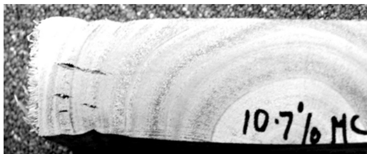
Figure 14. Collapse and internal checking in Eucalyptus nitens about 13-y old
