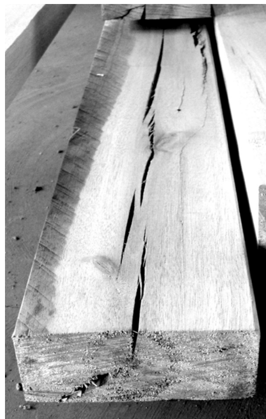
Figure 13. Heart checks in boards sawn heart-in (this example is 6-year-old Eucalyptus dunnii ).
