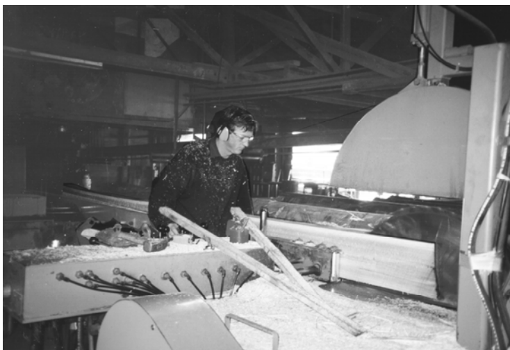
Figure 2. Conventional single-saw systems common in small sawmills in southern Australia, quarter-sawing plantation-grown Eucalyptus nitens
