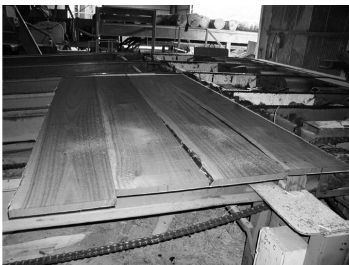
Figure 1. Knot-free slabs produced from 22-year-old pruned Eucalyptus globulus at the Auswest Timbers mill at Pemberton
