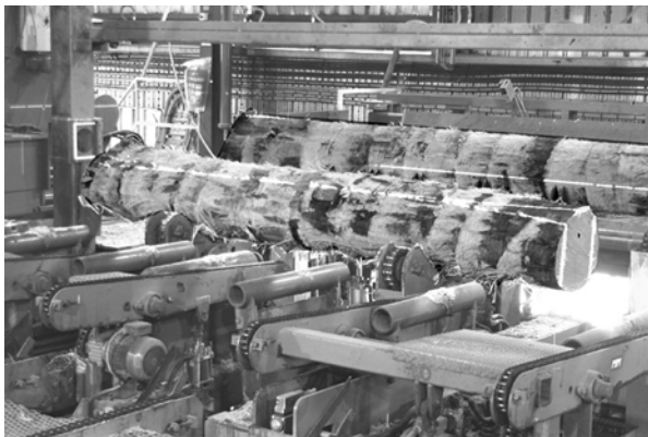
Figure 6. MEM twin-saw systems like this one at the Drouin West Sawmill can also be used for quarter-sawing
