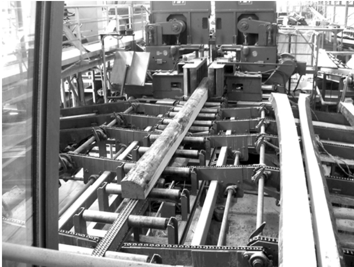
Figure 6. MEM twin-saw systems like this one at the Drouin West Sawmill can also be used for quarter-sawing
