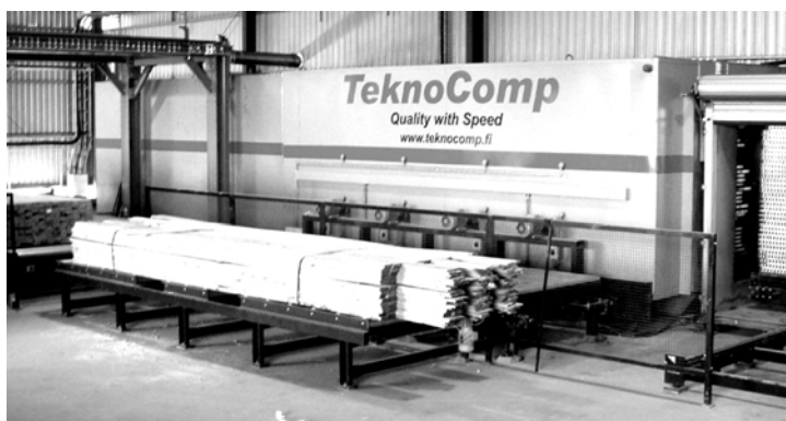
Figure 15. Compression kiln recently installed at Forest Enterprises Australia's Bell Bay sawmill for drying plantation-grown Eucalyptus nitens from green
