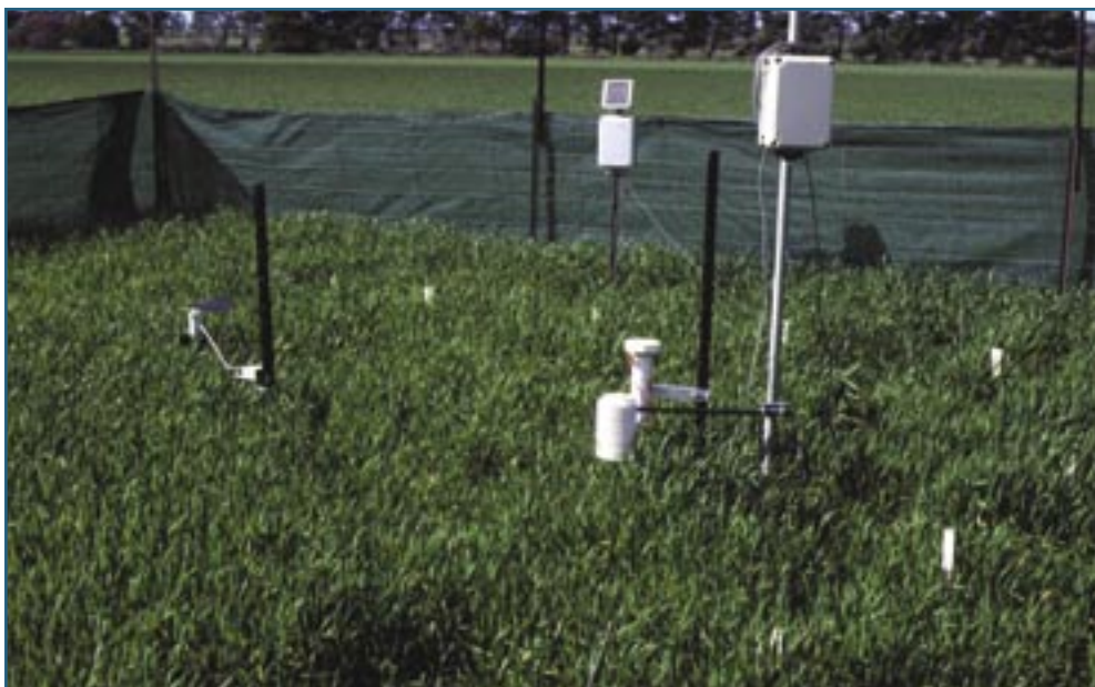
Measuring meteorological data at an artificial shelter at the Esperance, WA, field site.
