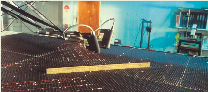
Figure 1.3 A different windbreak configuration used in the wind tunnel
