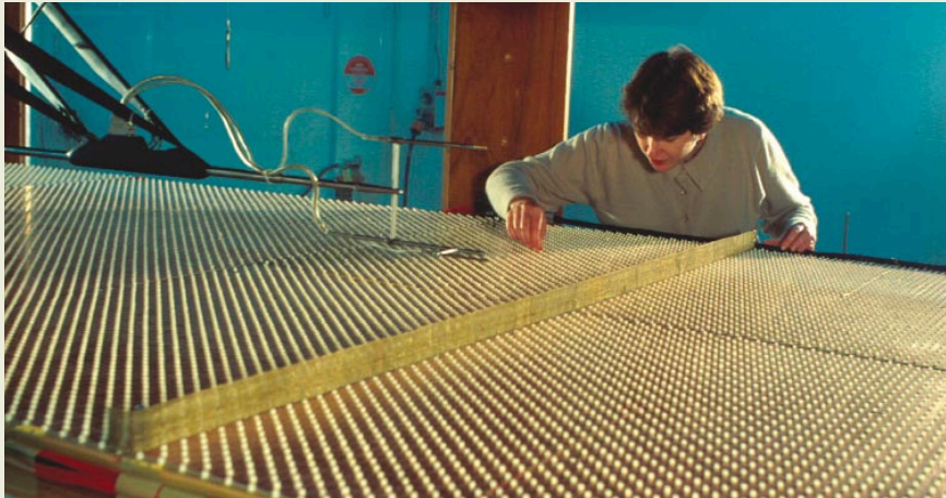
Figure 1.2 Scale model windbreak placed in CSIRO's wind tunnel. The floor is lined with a heated mat and pegs to mimic a warm, rough surface similar to tall grass.
