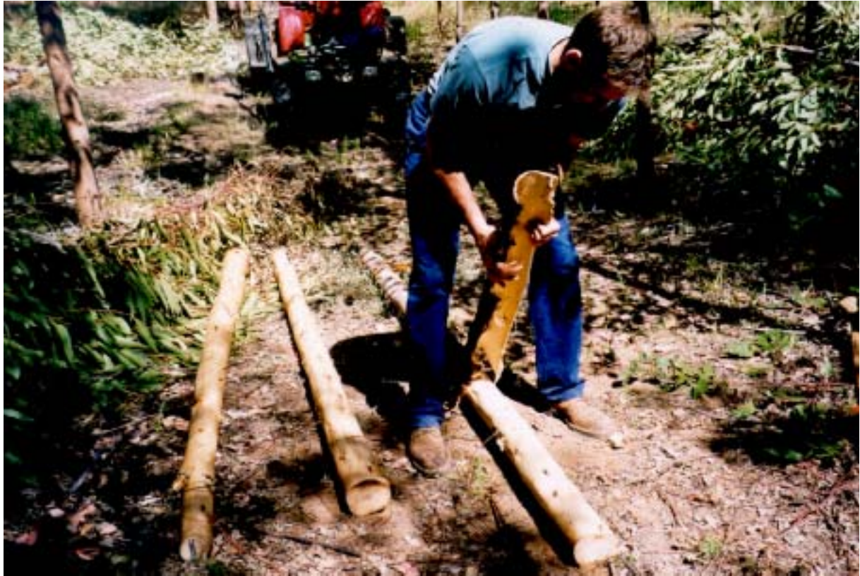
Figure 4. Debarking an E. grandis trellis post
