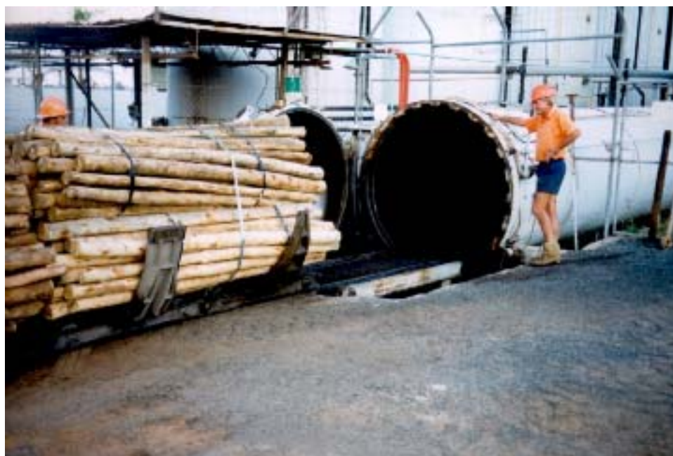
Figure 7. Untreated vineyard posts being loaded into the treatment cylinder at Koppers, Grafton
