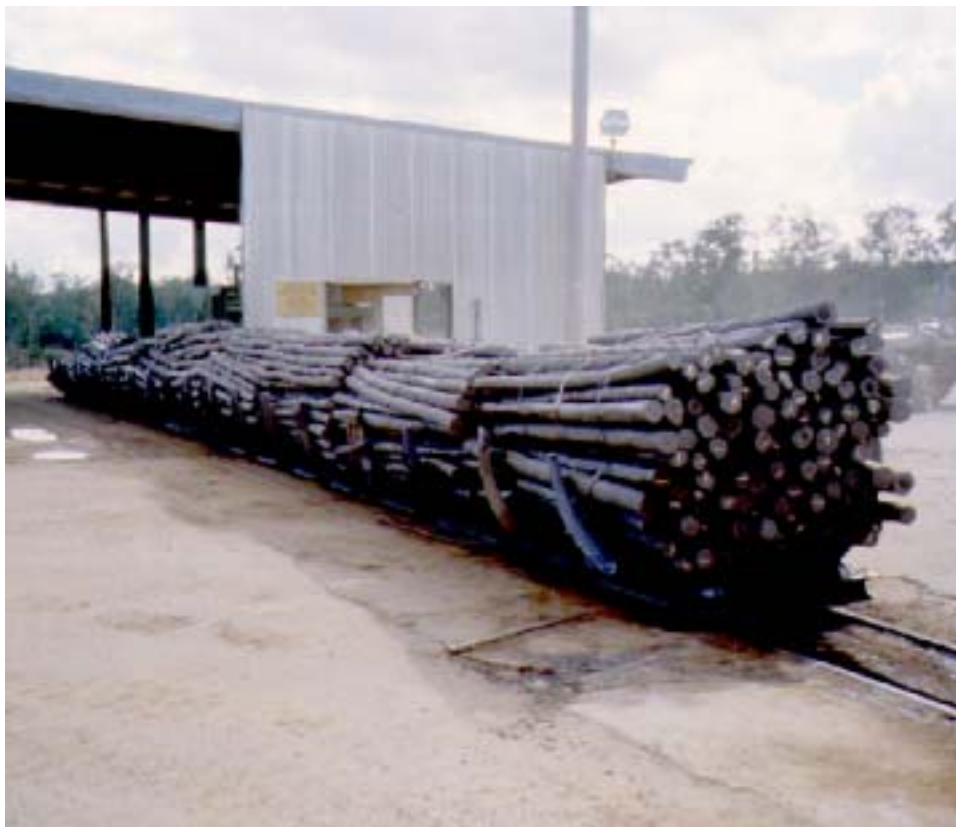
Figure 8. PEC-treated vineyard posts just after treatment
