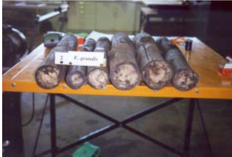
Figure 12. Transverse view of PEC penetration and distribution in E. grandis posts
