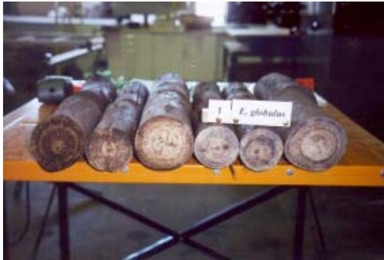
Figure 13. Transverse view of PEC penetration and distribution in E. globulus posts
