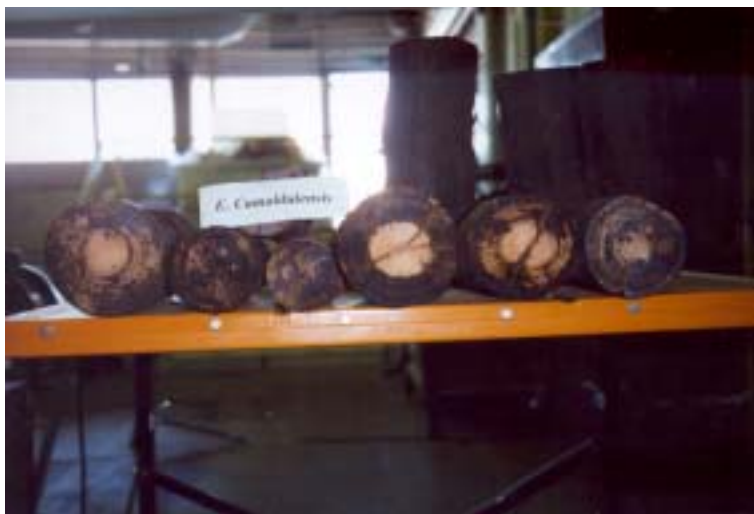
Figure 14. Transverse view of PEC penetration and distribution in E. camaldulensis posts
