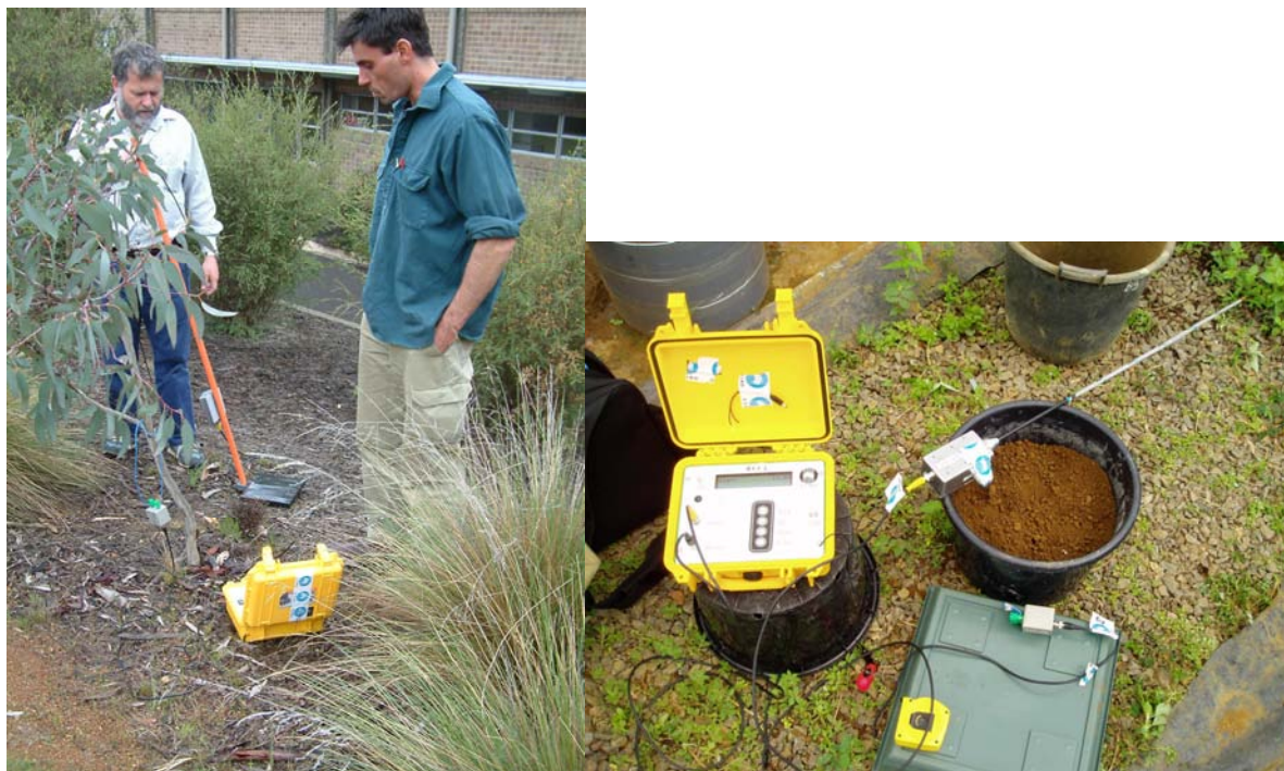
Figure 16 Shielded loop magnetic field sweep (left) in use with the portable vector voltmeter. Excitation of the tree is achieved using either a metal probe or, in this case, an induction loop around the stem. The electric field probe is shown on the right, connected to the vector voltmeter.
