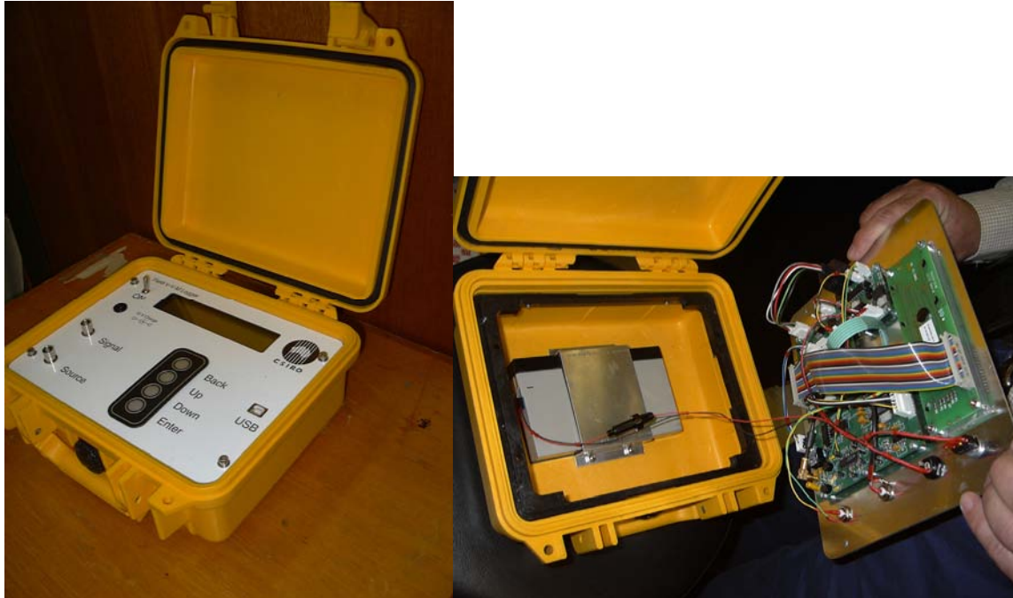
Figure 15 Portable vector voltmeter plus source developed to allow simultaneous excitation of plants in the field. This was used in conjunction with tuned receiver probes to detect electric and magnetic fields associate with plant roots.
