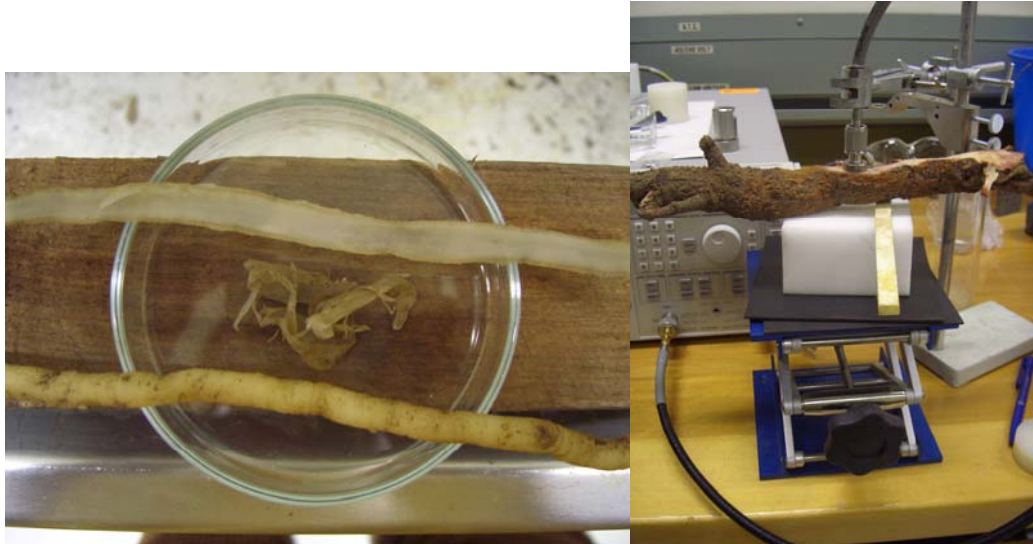
Figure 23 Agapanthus ( Agapanthus africanus ) root and root epidermis specimens in a Petri dish prepared for permittivity measurement (left) and the Hewlett Packard 85070B dielectric probe, connected to a Hewlett Packard 8714ES network analyser (right), measuring the permittivity of hakea root ( Hakea sp. ).
