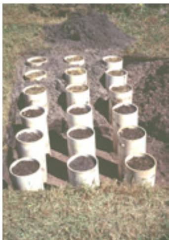
Plate 4. Soil cores from pasture (back) and plantation (front) areas being repositioned and buried in the pasture site.
