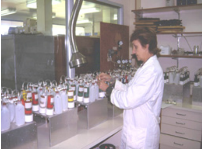
Plate 2. Multiple micro-lysimeter system used to determine cumulative mineral-N production in pasture and plantation soils.
