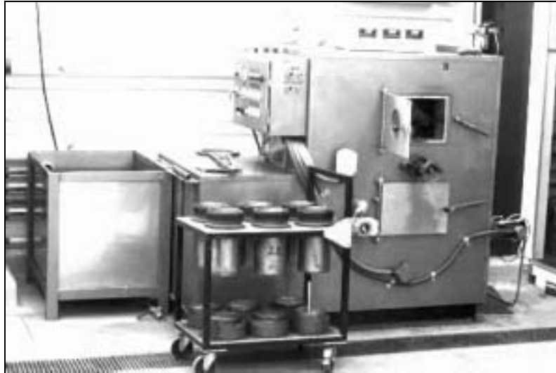
Figure 6 Air bath used for kraft pulping trials with pressure vessels in foreground
