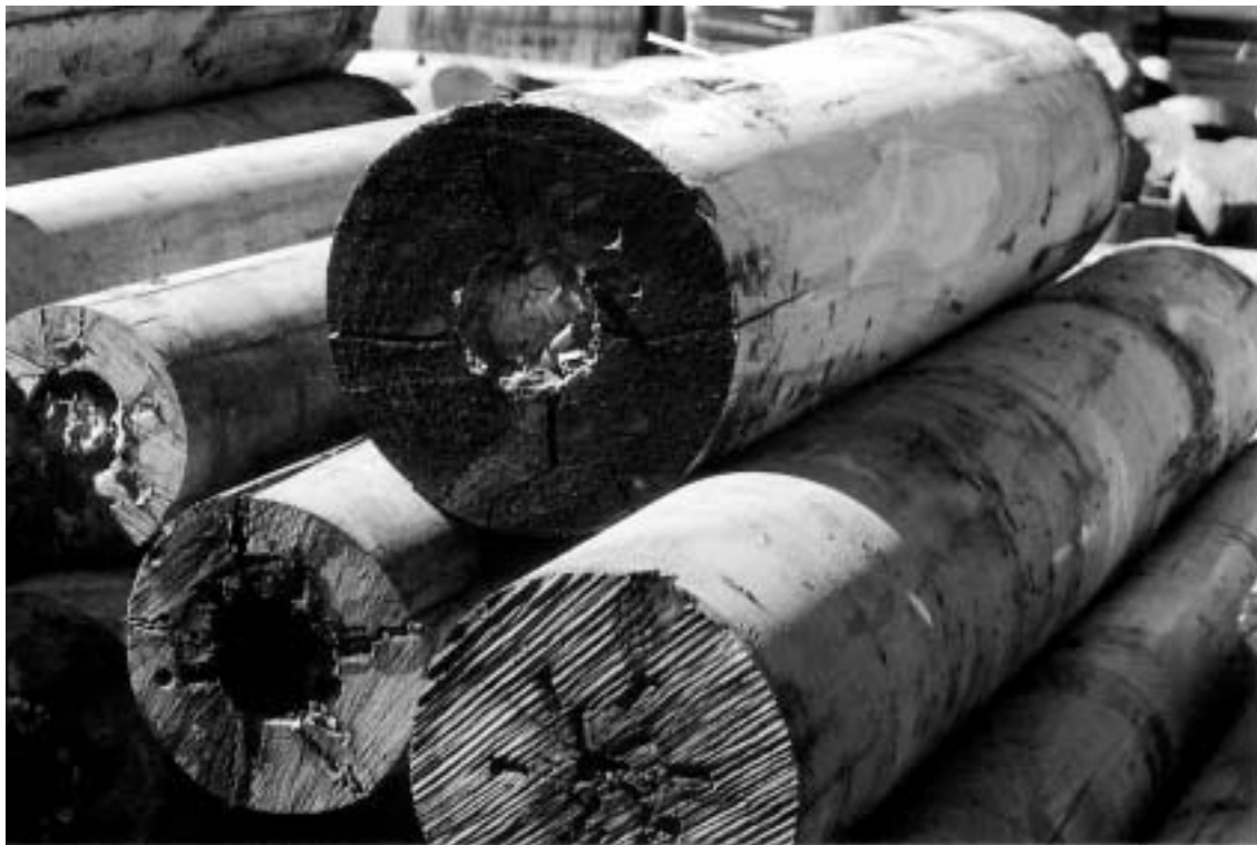
Figure 9: The effect of core defect on veneer logs. These logs were rejected after the turning chuck failed to grip.
