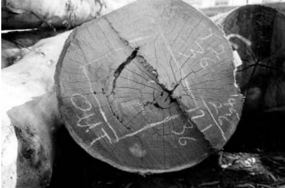
Figure 7: The total of core defect and loose ring defect has made this log unacceptable. Chalk marks show miller's estimate of volume to be "boxed out".
