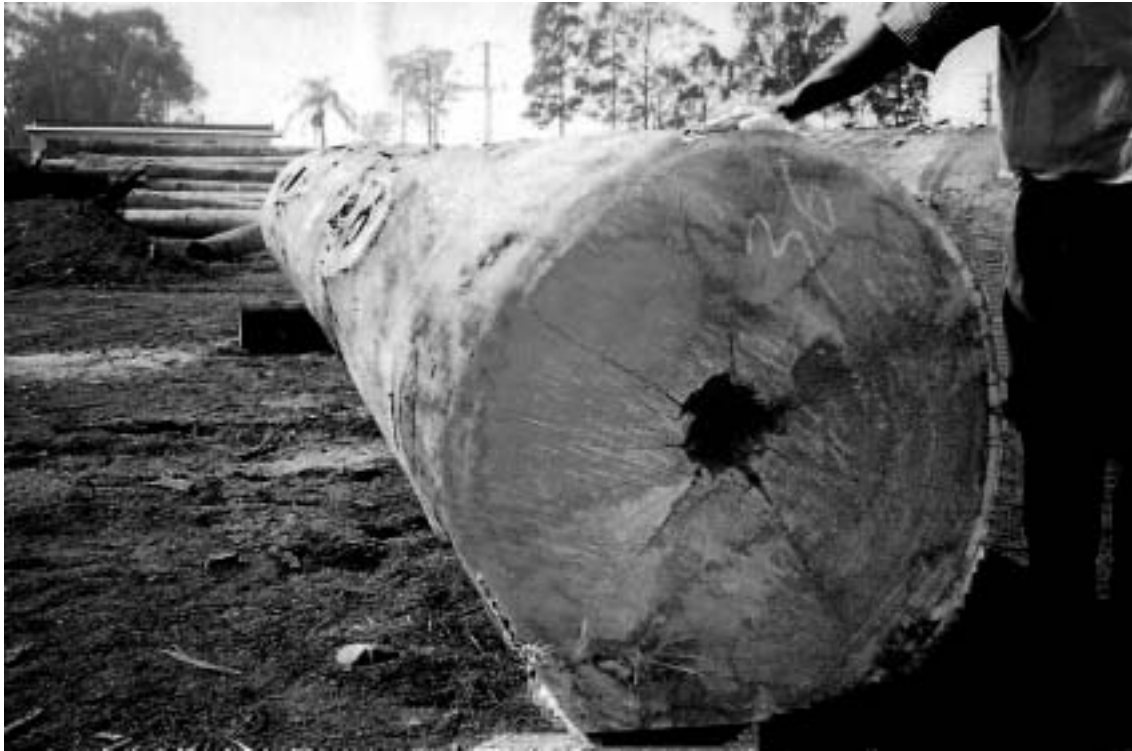
Figure 1 : A high quality Tallowood sawlog from the North Coast of NSW. Only a small volume is lost to pipe defect.
