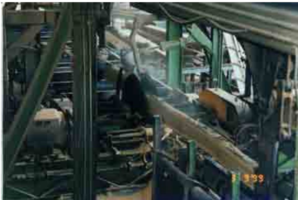
Plate 4 E. dunnii log being processed through a twin circular saw edger
