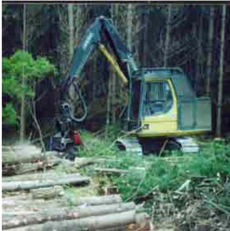
Plate 9 Sample trees of Pinus radiata being mechanically harvested and cut into logs for sawing.
