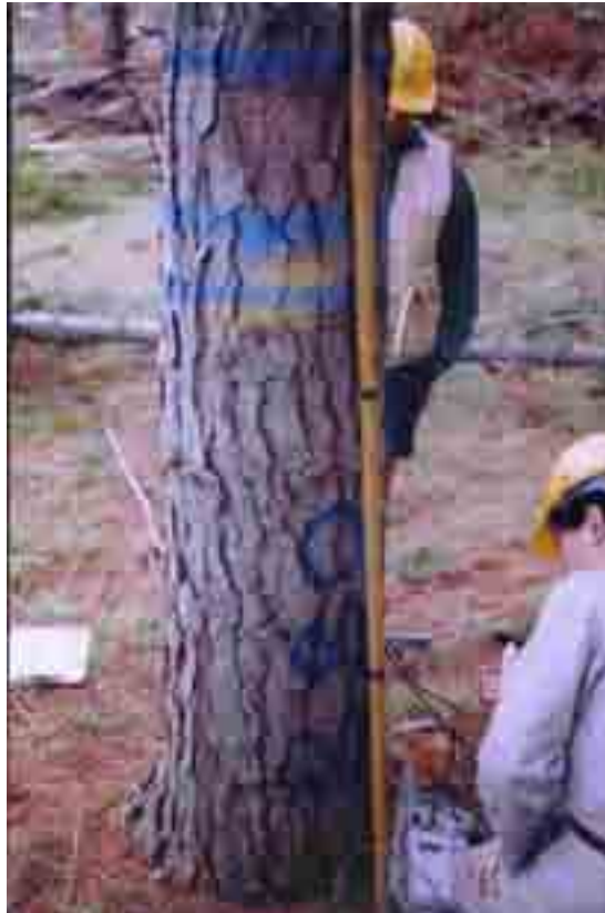
Plate 7 A standing tree of Pinus radiata being measured acoustically using a FAKOPP stress wave timer. A stress wave is induced by tapping the “start” probe (located at the bottom of tree) with a hammer, and the time it takes to reach the “stop” probe is read off from the instrument.
