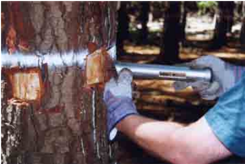
Plate 8 A Pilodyn wood tester is fired into the outer wood of the standing tree and the depth of pin penetration is read off the instrument to nearest 0.5 mm.
