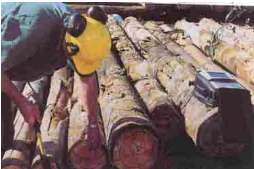
Plate 3 E. dunnii logs being measured acoustically with a HP stress wave resonance device.
