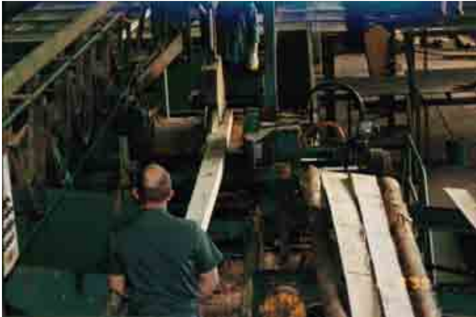
Plate 5 E. dunnii flitches being processed at a Gibson hob resaw bench.
