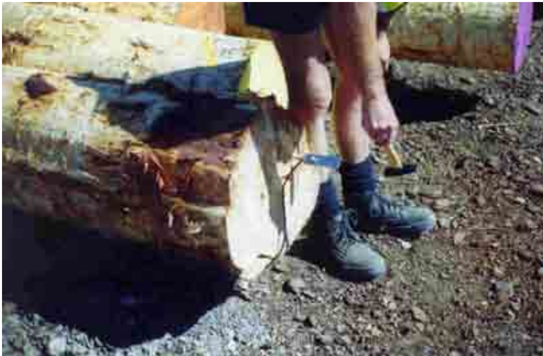
Plate 11 A sample log shown is being measured acoustically with a FAKOPP stress wave timer at the mill yard.
