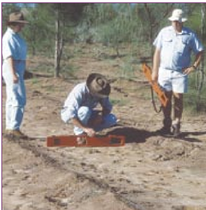
Photo 1.3 Measuring soil salinity with the EM38. (Photograph Stephen Midgley)
