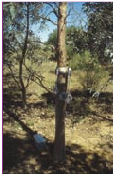
Photo 1.7 Heat pulse equipment installed onto the stem of an E. camaldulensis tree (Photograph Nico Marcar)
