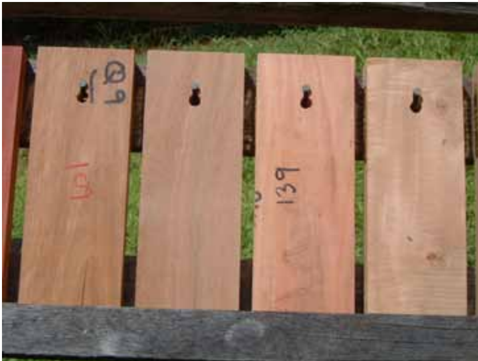
Figure 3. Assessment of above-ground durability using a flat panel test at Innisfail
