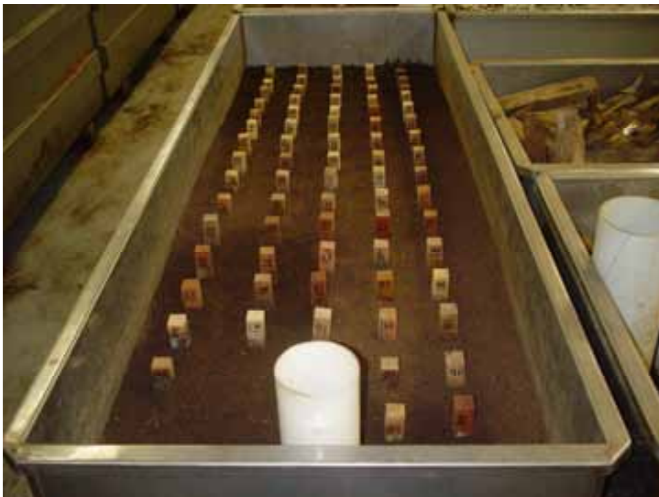
Figure 4. CSIRO's Accelerated Field Simulator used to test in-ground decay resistance
