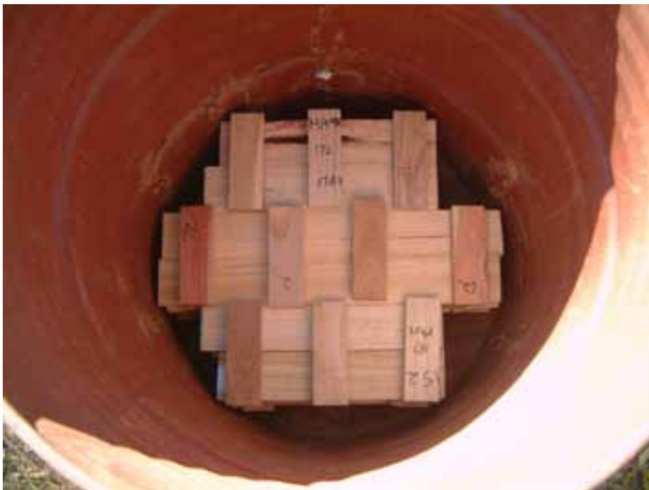
Figure 5. Testing wood samples for resistance to termite attack
