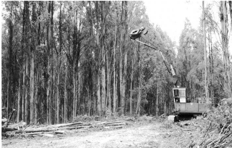
Figure 2.1 Cable thinning at Repulse 3, southern Tasmania in 1991. The skyline cable system used a gravity return carriage mounted on a Prentice excavator to yard logs upslope to the roadside landing
