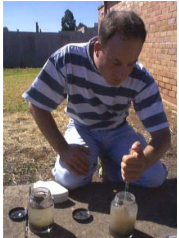
A farmer using the turbidity meter prior to main SAS kit session to test sodicity to test his sub-soil.
