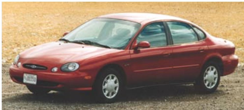
Ford Taurus flexible fuel vehicle (FFV) that runs on E85
