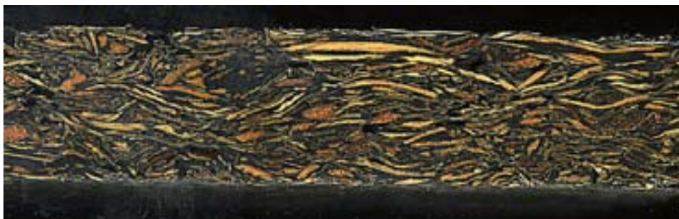
Plate 4-8: Cross-sectional profiles of CBPs made from (a) factory-produced particles of radiata pine, and screened small-sized elements of (b) blue gum and (c) mallee eucalypt.
