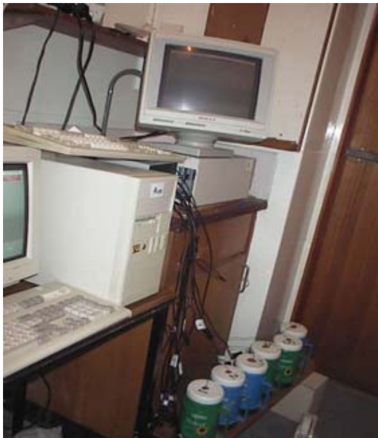
Plate 2-2: Apparatus used to measure cement hydration temperature.
