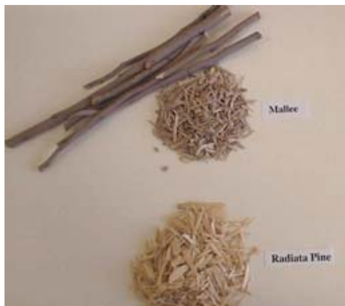
Plate 3-3: Chipped mallee eucalypt particles and radiata pine particleboard flakes.
