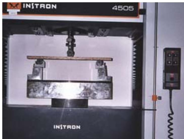
Plate 3-1: Three-point bending test for board samples.
