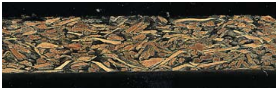
Plate 3-2: Sanded cross-sections of cement bonded boards made from (a) radiata pine particleboard flake, and (b) chipped residues from E. polybractea .
