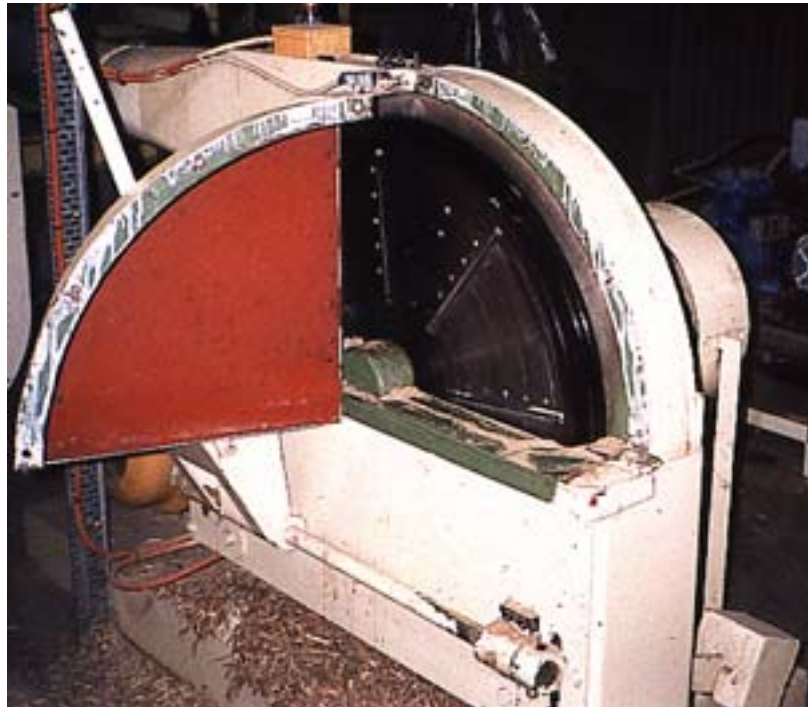
Plate 4-1: Disk flaker used to produce flakes and particles from log samples.
