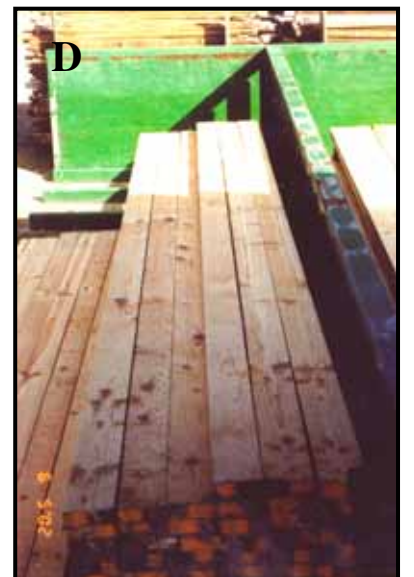
Figure 37: Typical knot characteristics. A & B shows clusters of smaller diameter knots with distinct nodal spacing in P. canariensis . C & D show less uniform spacing of larger knots in P. brutia .
