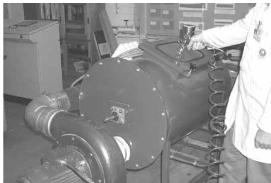
Figure 11: Resin and wax application to dried fibres
