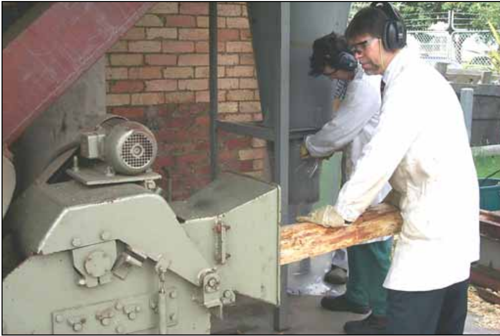
Figure 4: Chipping the billets in a Bruks pilot-scale chipper
