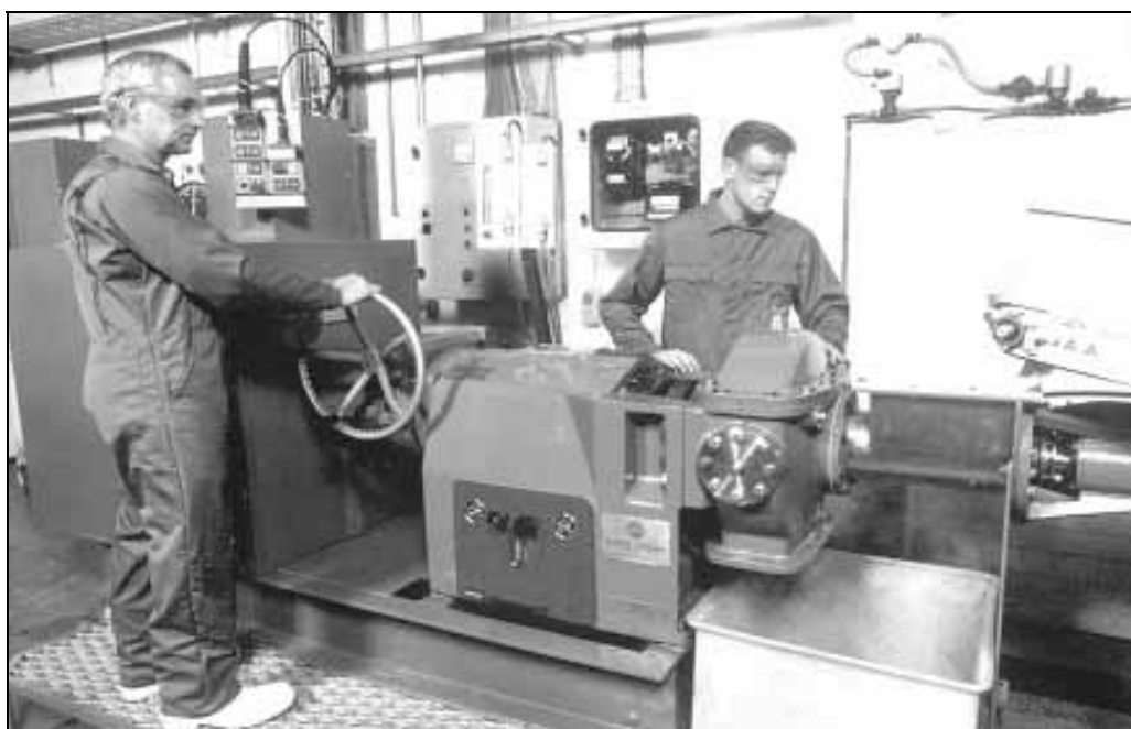
Figure 10: The Sunds Defibrator ROP20 used for secondary refining
