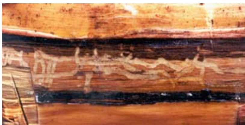
Figure 5. Typical cypress pine jewel beetle damage on outer sapwood.
