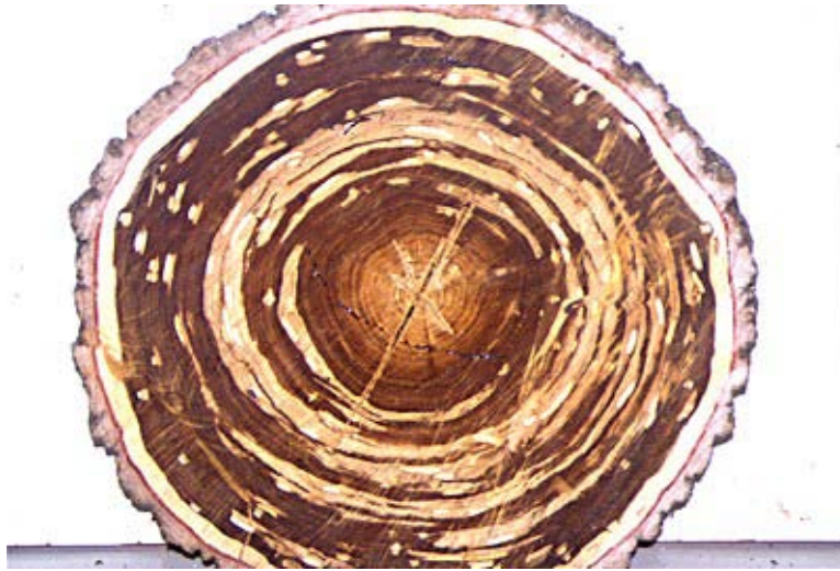
Figure 9. Severe DWG damage in cypress heartwood (white patches).
