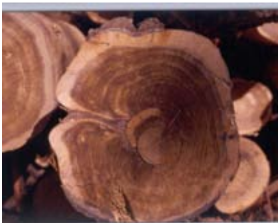
Figures 17 and 18. Cypress log and stump showing patch of decay (pale crescent) under healing scar.
