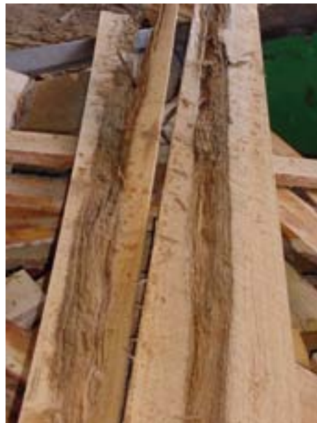
Figure 19. Brown rot ( Gloeophyllum spp.) in a board sawn from a log harvested at site 7 of the study.
